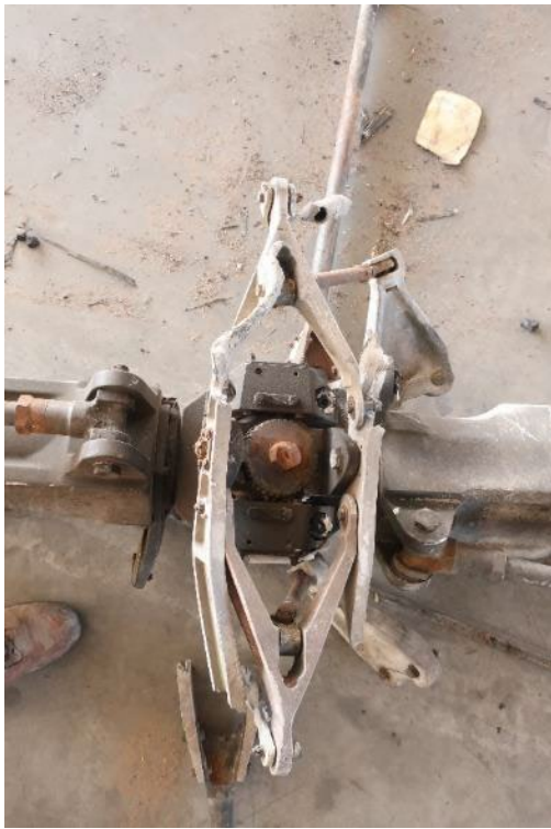
Photo 15. Rotor Head with Stabilizer Bar
