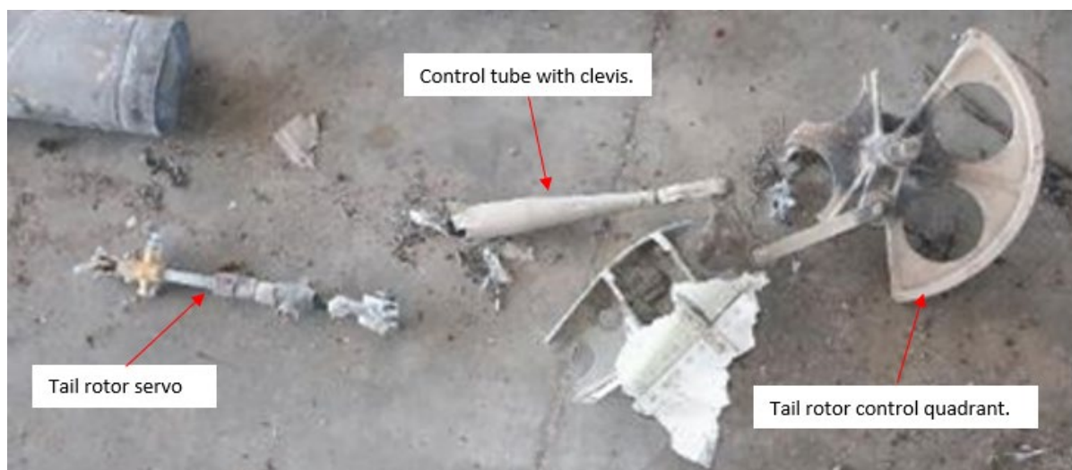
Photo 7. Tail rotor control quadrant, control rods, and hydraulic servo.
