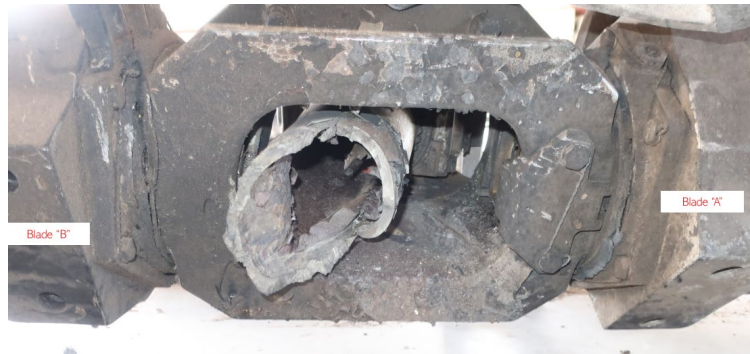
Photo 16. Rotor Head Main Mast Fracture
