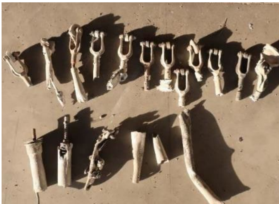
Photo 5. Flight control tube rod ends (clevis assemblies).
