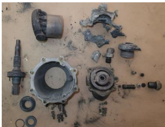
Photo 11. Hydraulic pump disassembled.
