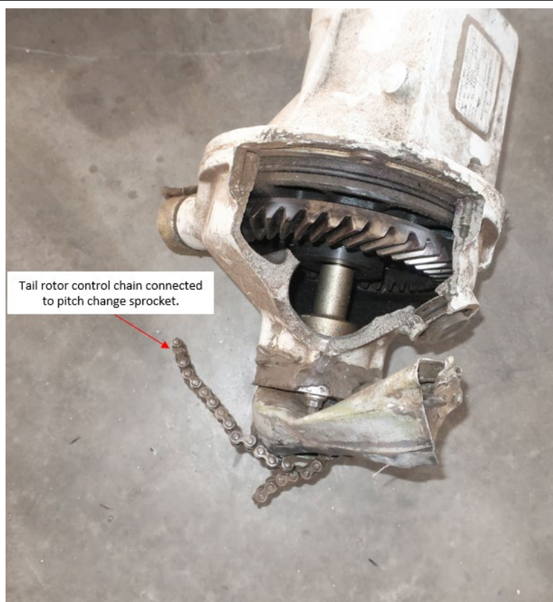
Photo 9. Tail rotor gear box and control chain segment connected to the pitch change sprocket.
