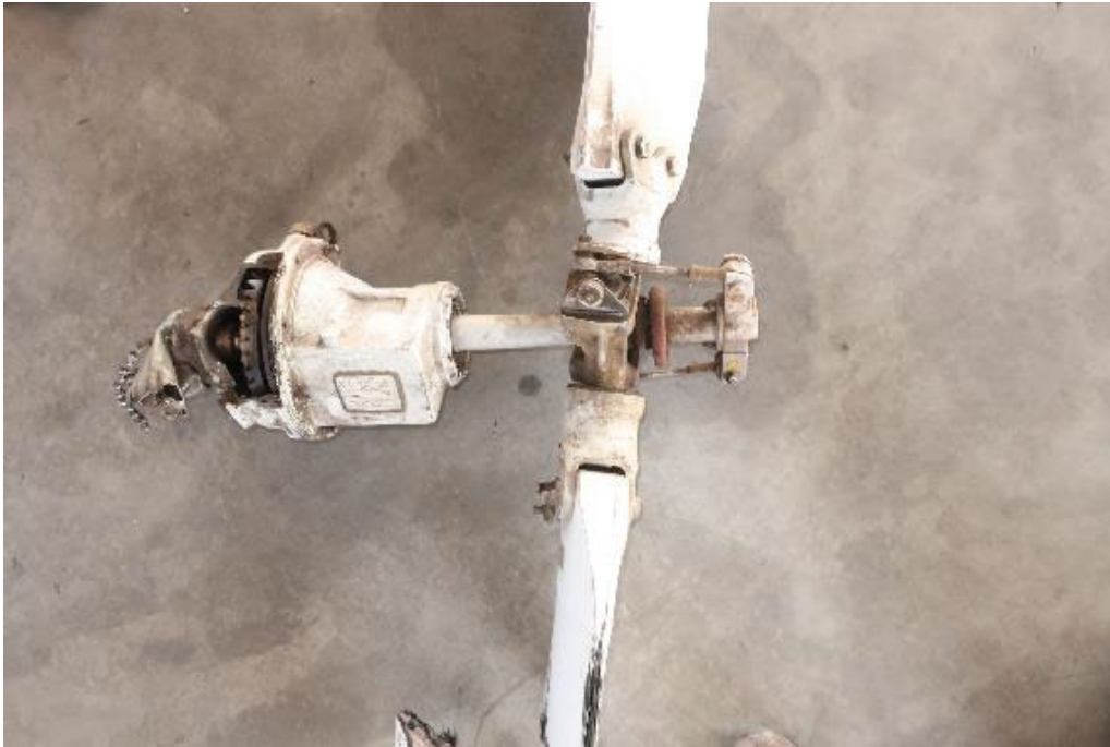
Photo 20. Tail rotor gearbox, rotor hub and blade assembly.
