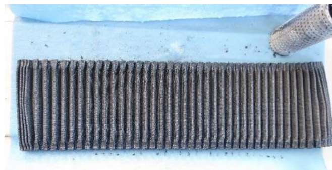
Photo 12. Hydraulic filter disassembled.
