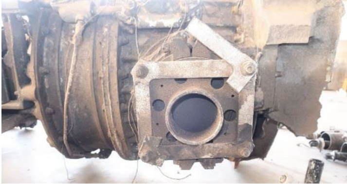
Photo 13. Transmission Power Input Quill
