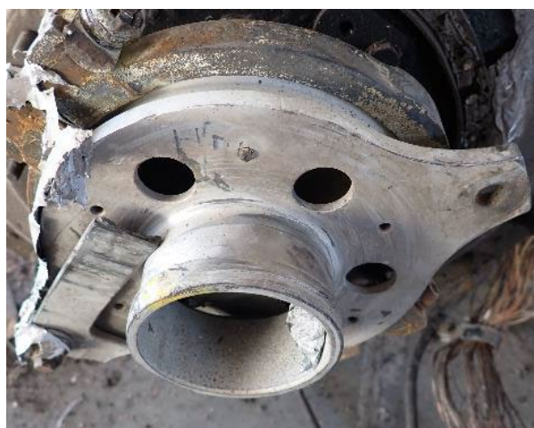
Photo 25. - Rotational scoring on the engine output flange.
