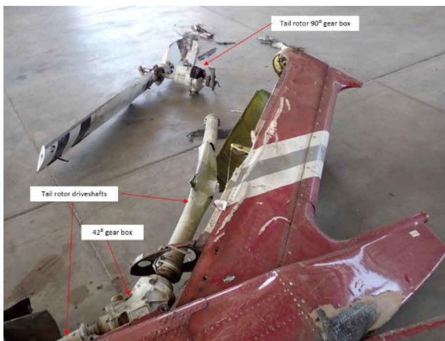
Photo 19. Tail section and tail rotor drive system.
