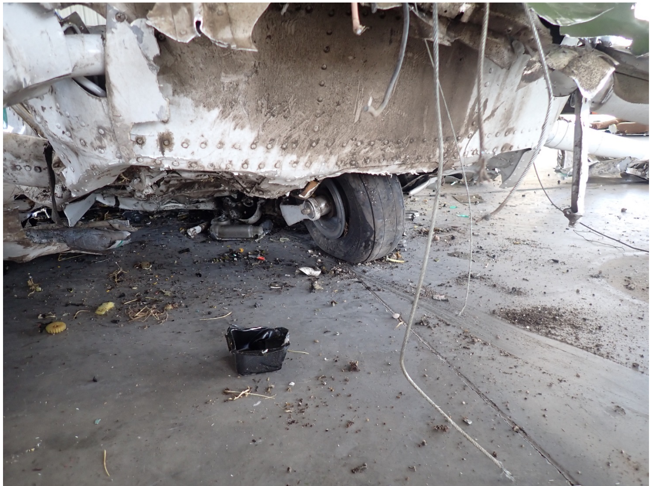
Nose landing gear forced aft through cabin floor, ASI-20-CO-012
