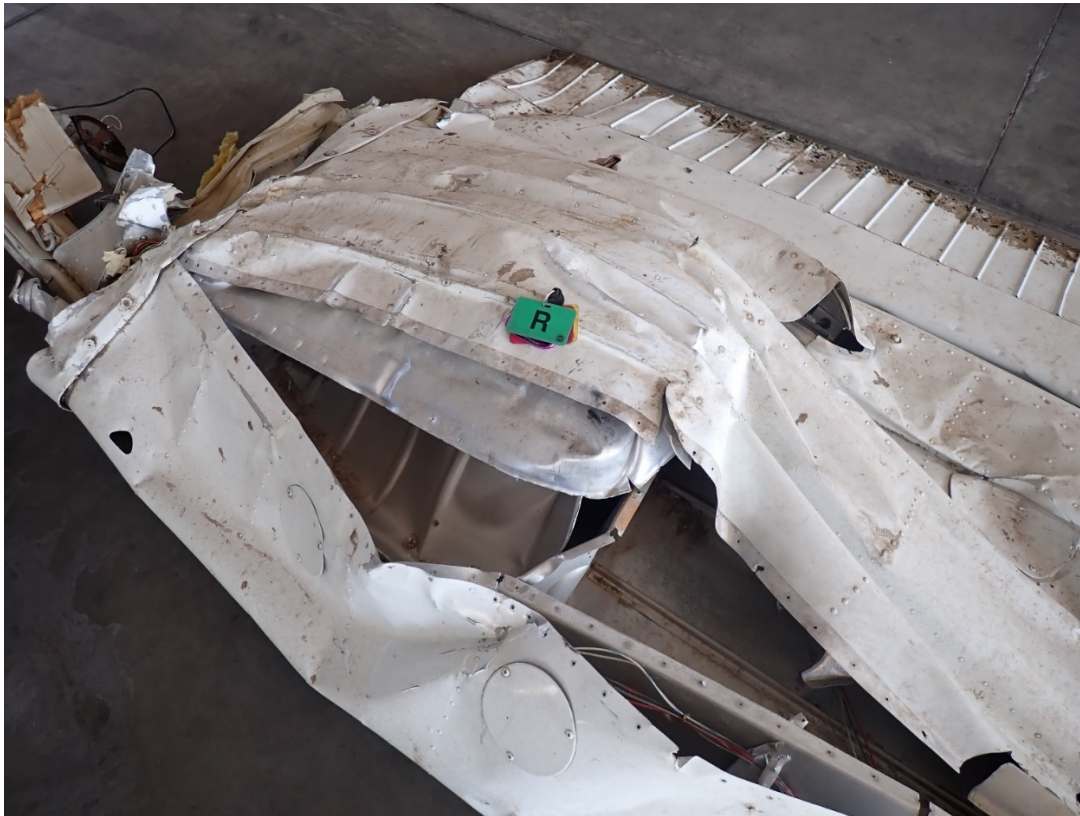
Right wing fuel tank, ASI-20-CO-063
