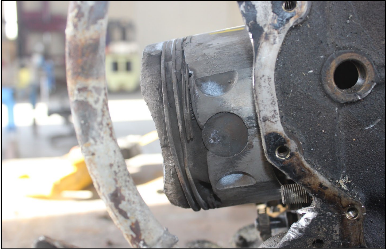
Figure 3: No. 4 cylinder piston head as viewed from the side.
