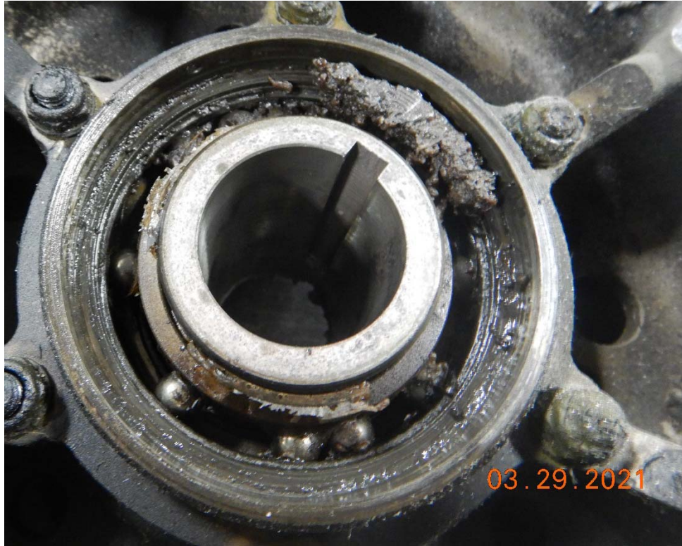
Figure 2. Overrunning Sprag Clutch - Forward Side
