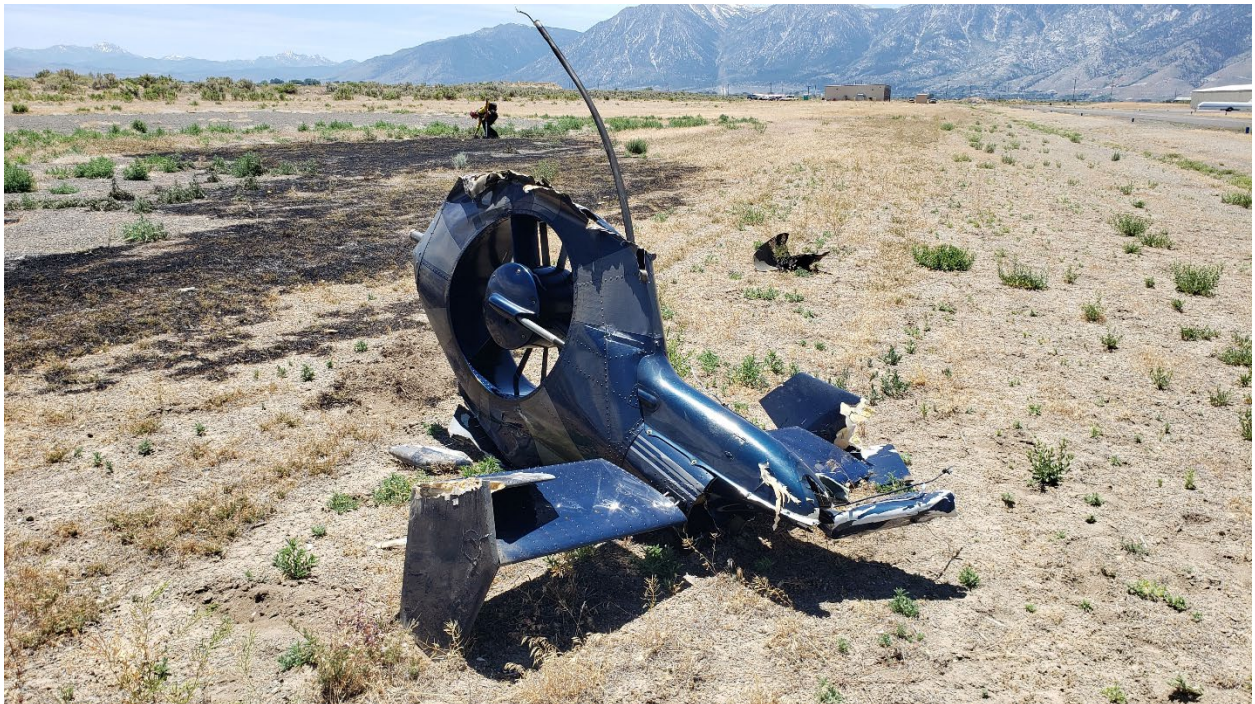
Figure 3. Photo of the fenestron and tailboom end. Photo courtesy of the airport manager.
