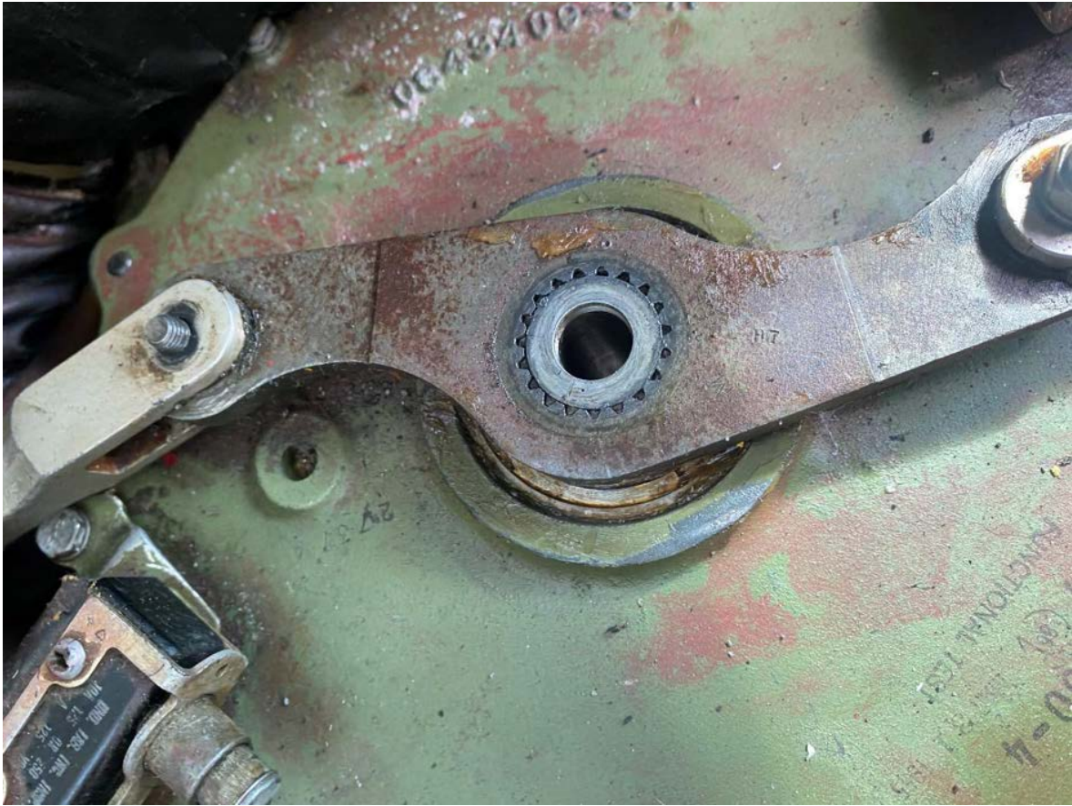
Actuator splines intact
