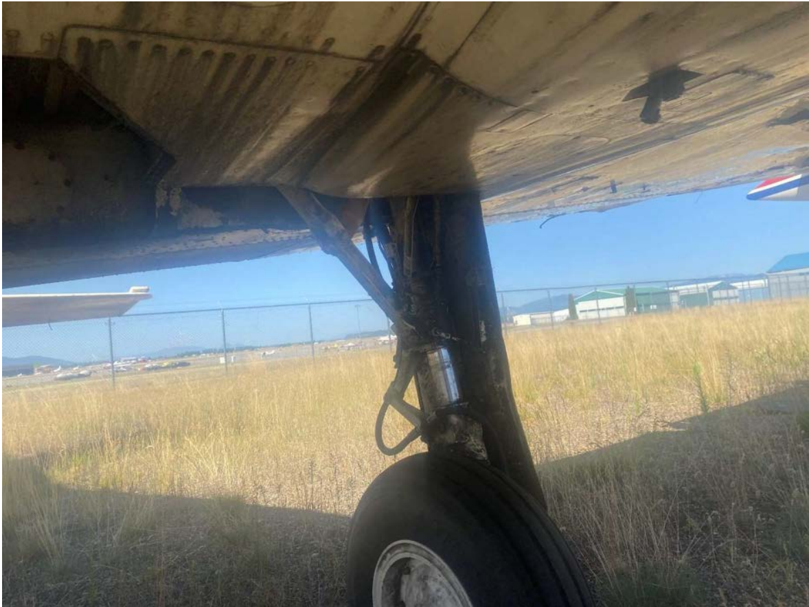
General Condition of Oil and Dirt throughout gear wells
