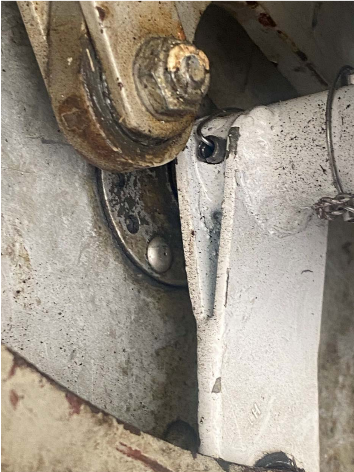
L/H Gear close up of replaced roll pins
