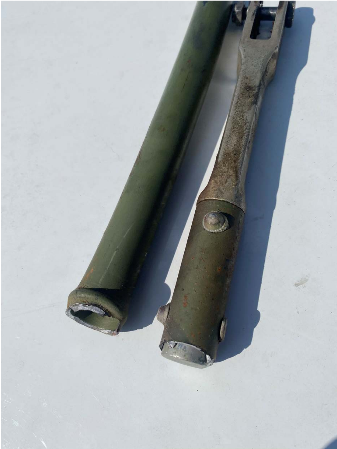
L/H Gear close up of broken drive tube
