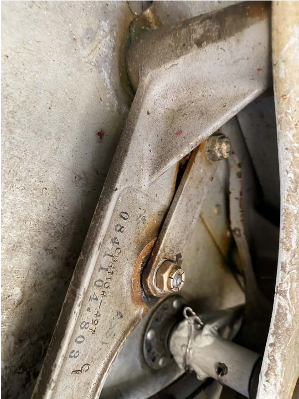
L/H Gear no bolt protrusion
