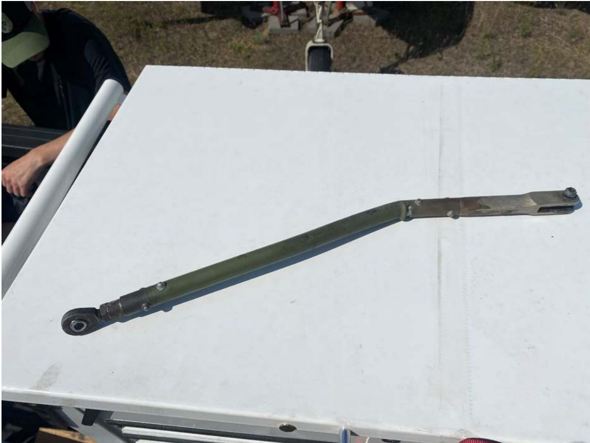
L/H Gear Main Drive Tube removed from A/C
