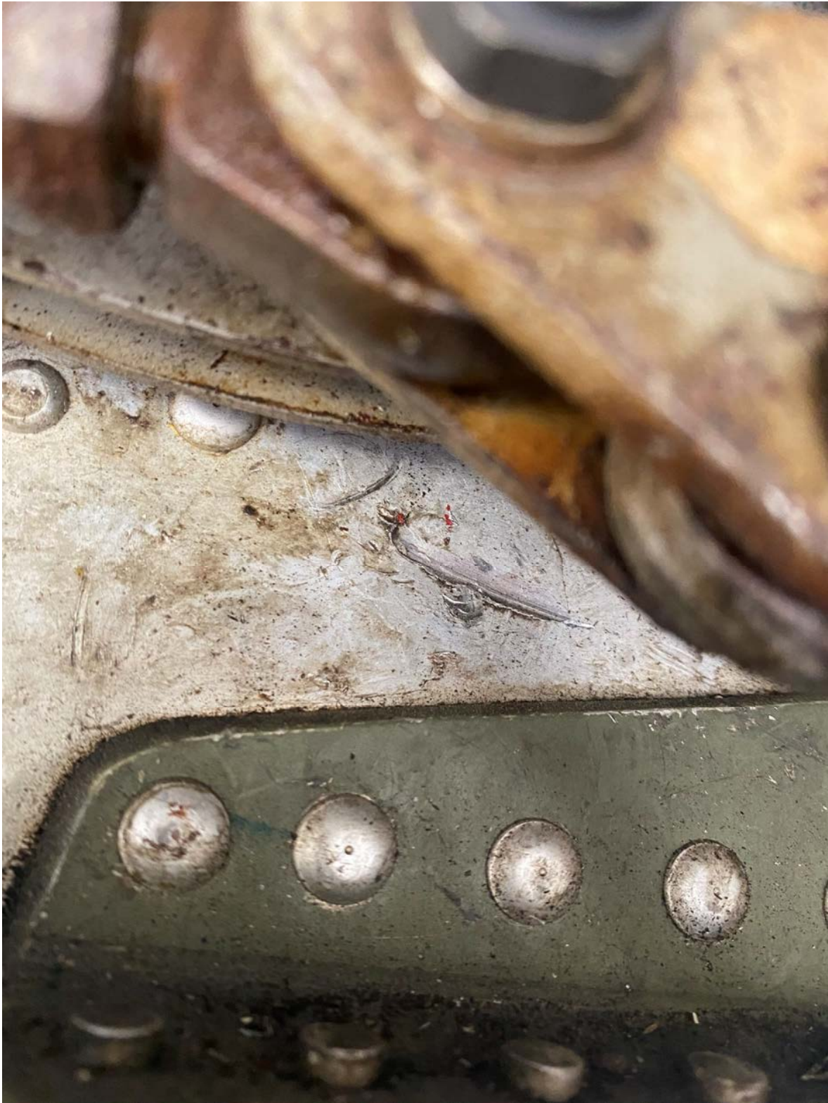
L/H Gear recent gouge in bulkhead behind idler arm undetermined cause
