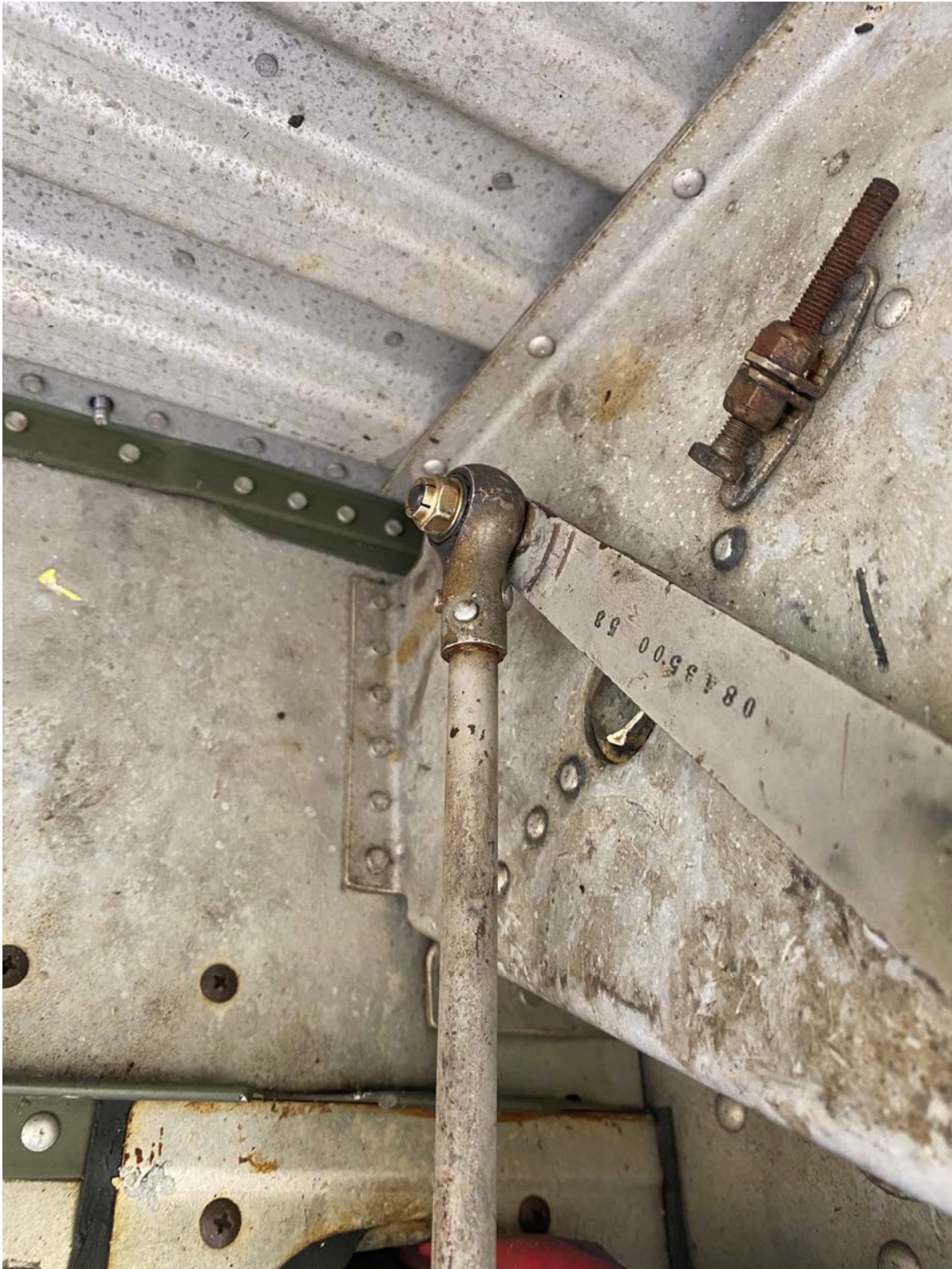
R/H Gear new "short" hardware on gear door
