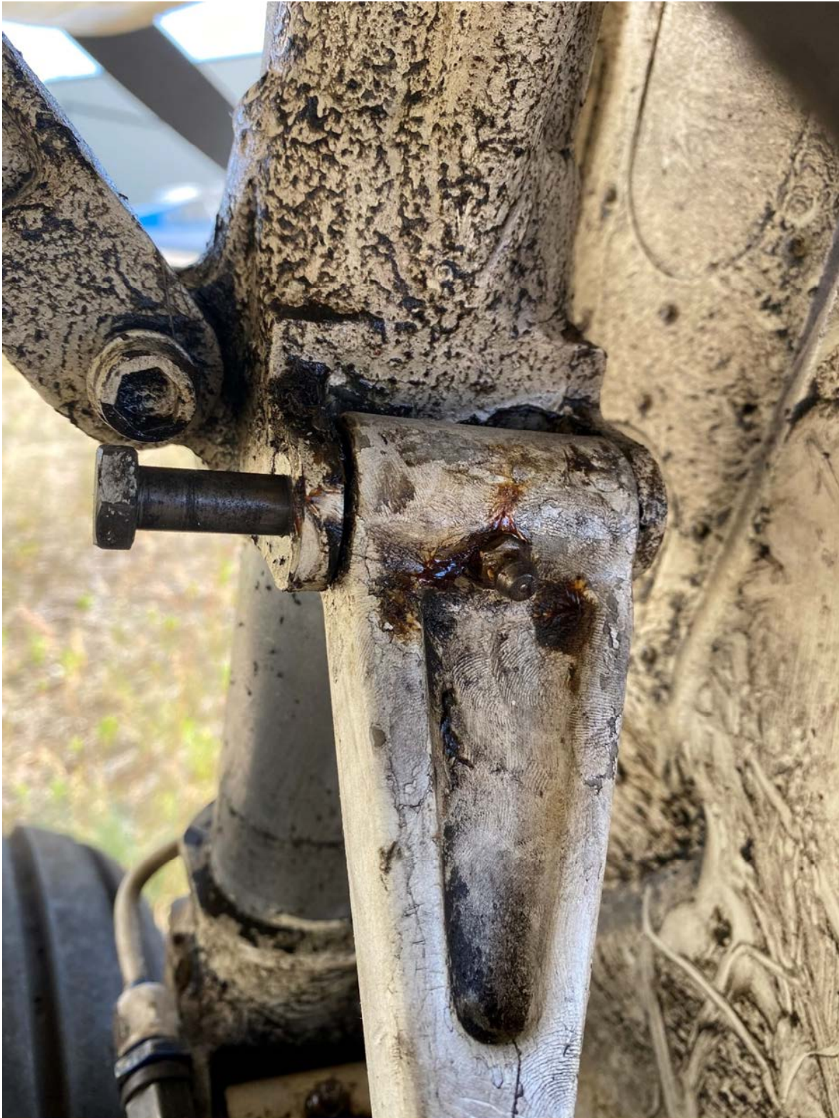
Backed out bolt on r/h Gear
