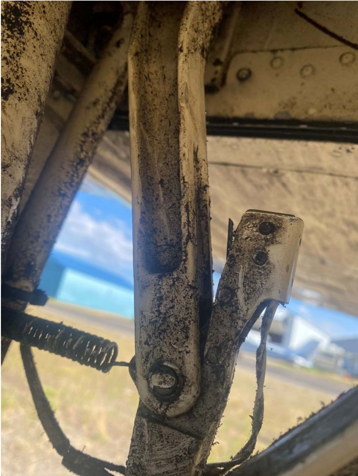
L/H Gear Lock Link as found condition (unlocked)
