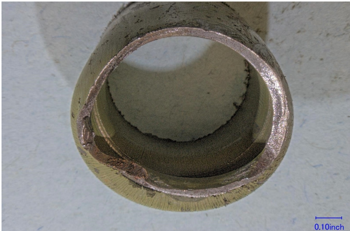
Figure 5 – Closer view of the outboard fracture surface, after sectioning and cleaning.
