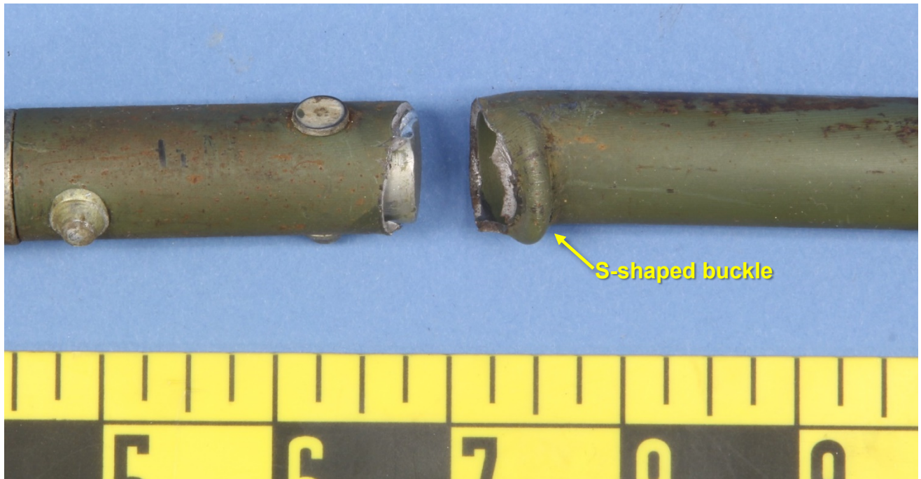
Figure 3 – View of the mating fracture surfaces, viewed from the compression side.
