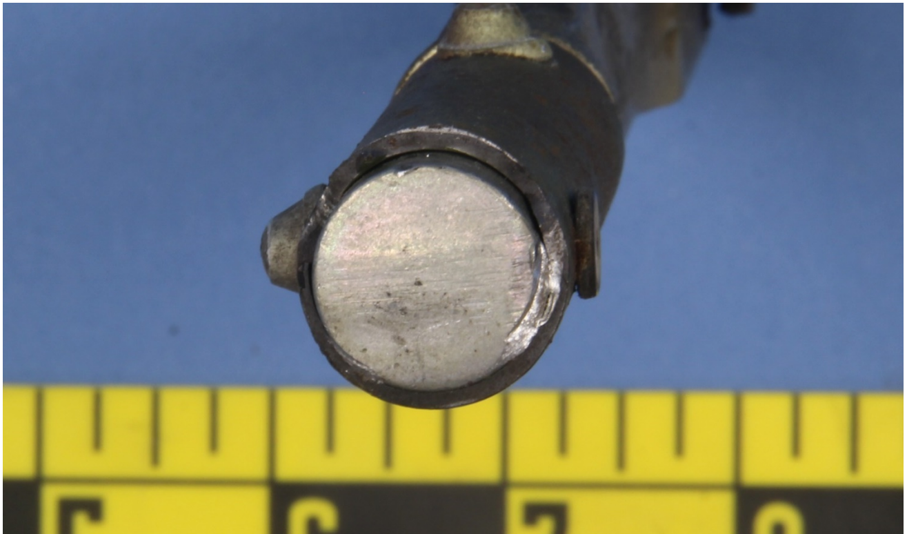
Figure 4 – View of the fracture surface from the inboard side, showing the clevis base.
