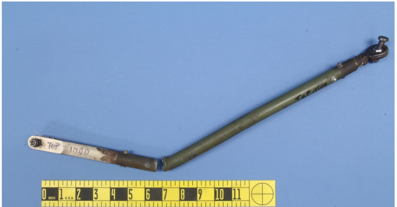
Figure 1 – The left hand MLG drive tube remnants, viewed as received and positioned in their orientations at final fracture.
