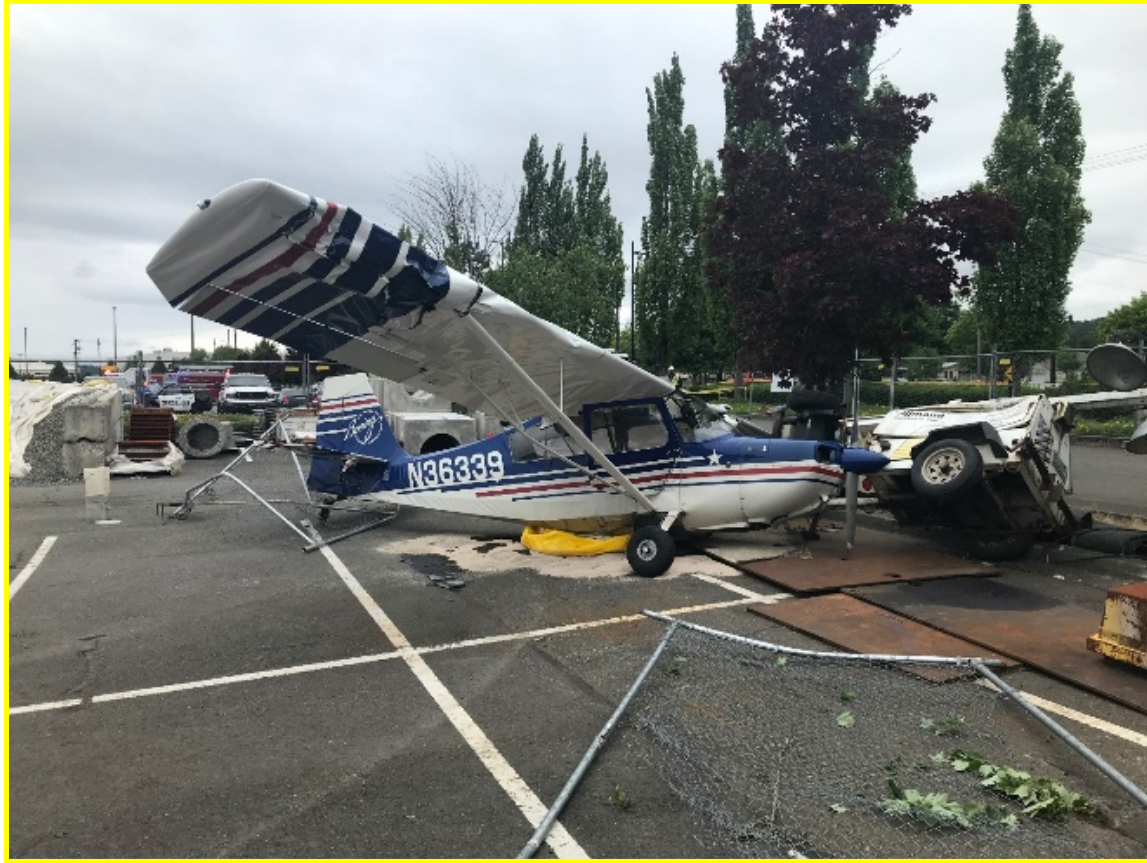
Photo 4 - View of right-wing damage
