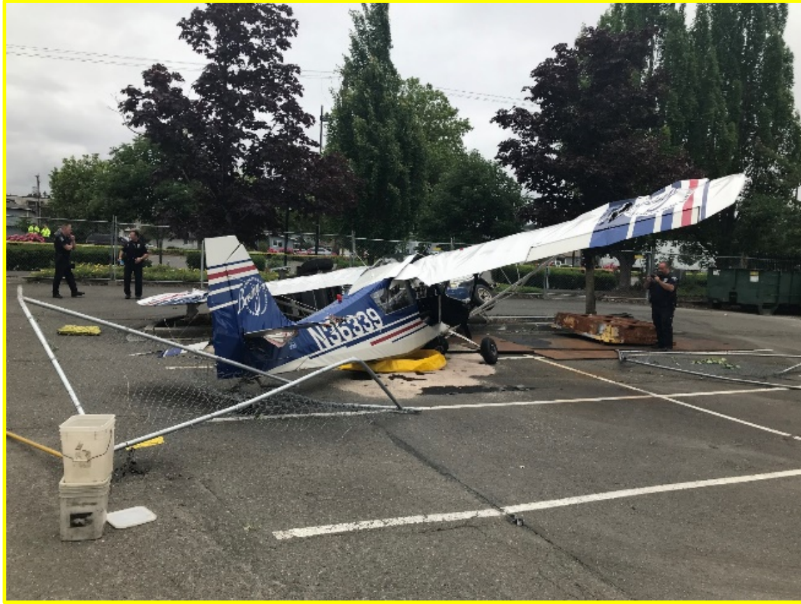
Photo 6 - View of empennage damage
