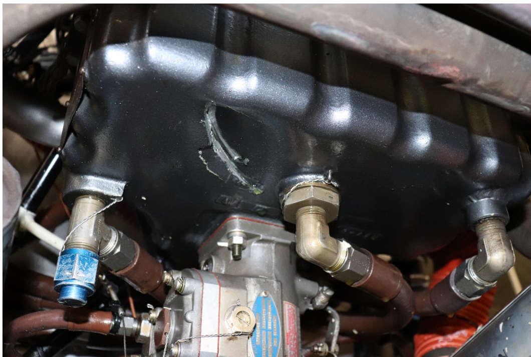
Figure 14. View of damage to the oil sump
