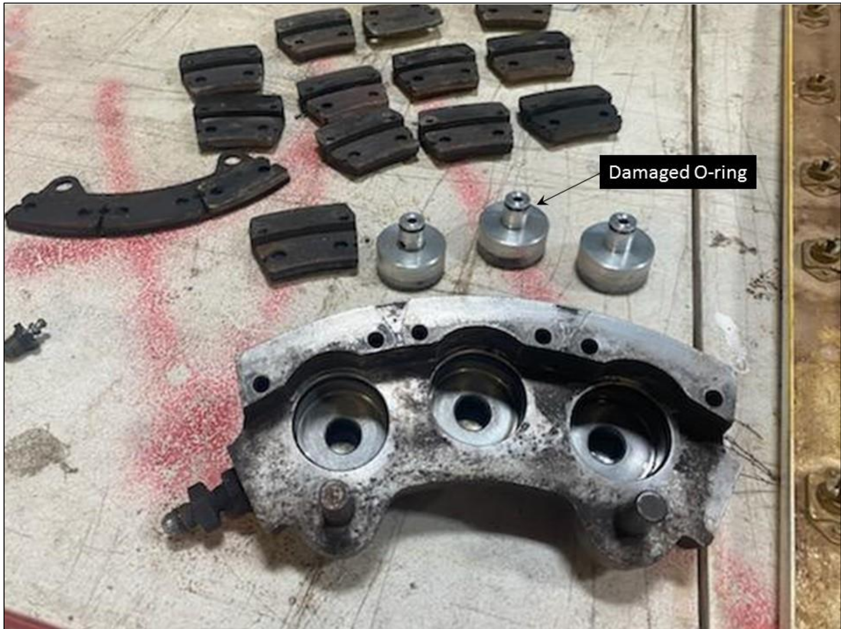
Photo 2 – Postaccident examination-brake parts.(Courtesy of the Airplane Owner)
