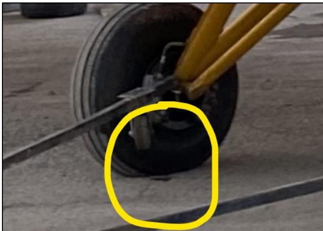
Figure 1-Right main landing gear tire and brake fluid puddle.
