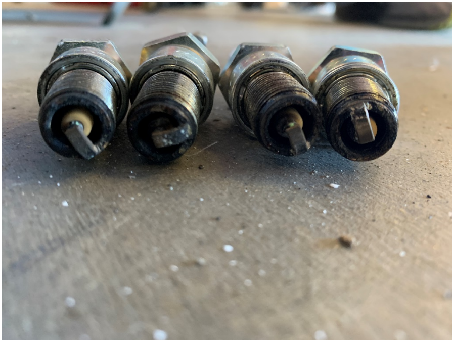
Figure 5: Removed spark plugs.
