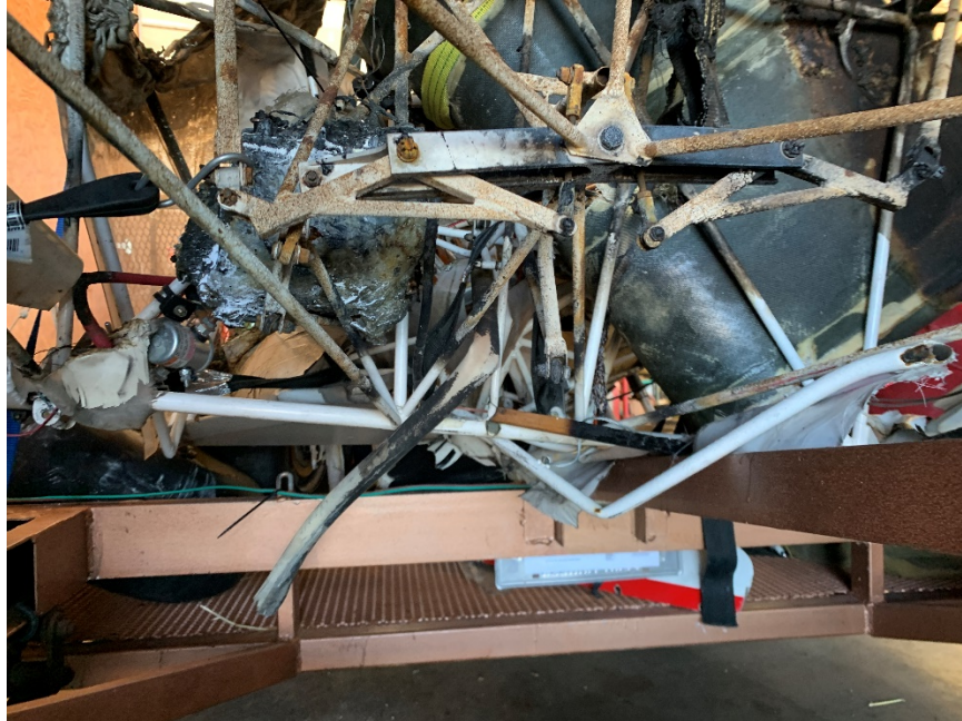
Figure 3: Control linkages, note the elevator torque tube damage.
