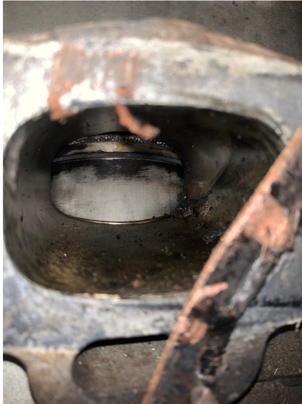
Figure 6: View of one piston through the exhaust port.
