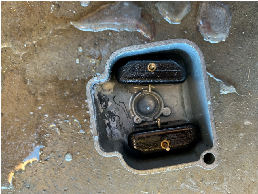
Figure 8: Debris within the carburetor float bowl.
