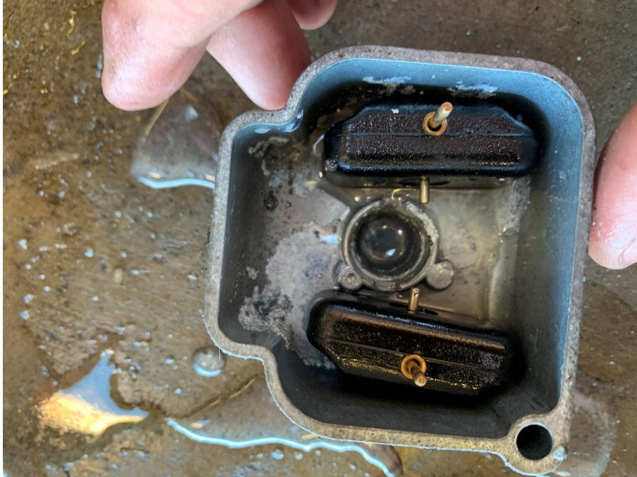
Figure 7: Debris within the carburetor float bowl.
