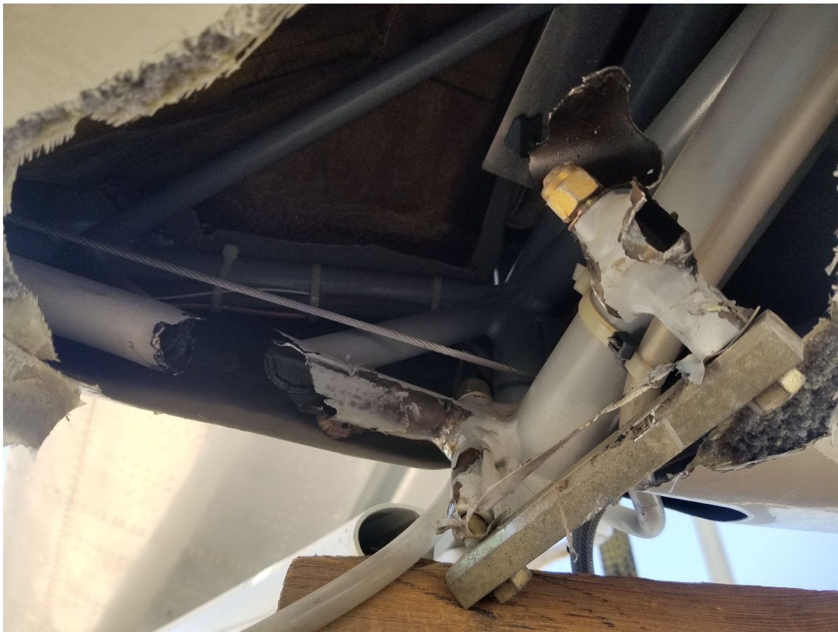
Photo 3 – Right main landing gear support tubing (Courtesy of Fox Aviation)
