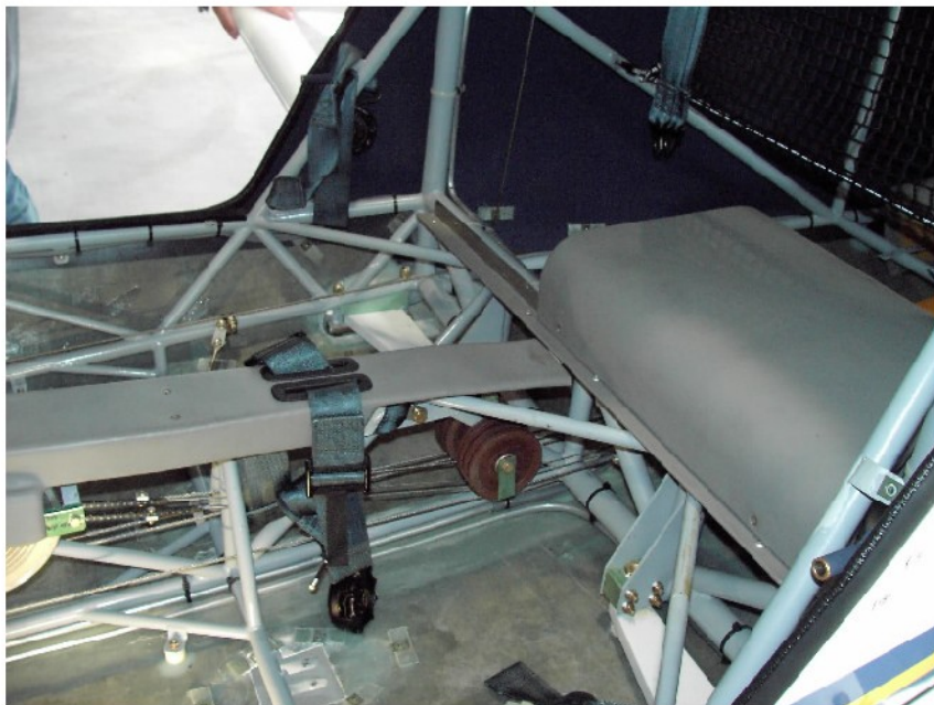
Figure 2: Removal of fuselage tank cover
