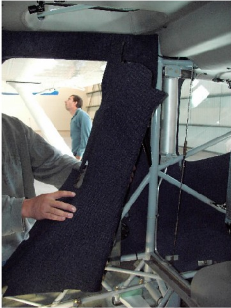
Figure 3: Removal of wall fairings
