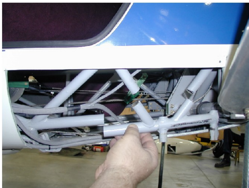
Figure 6: cutting the cage
