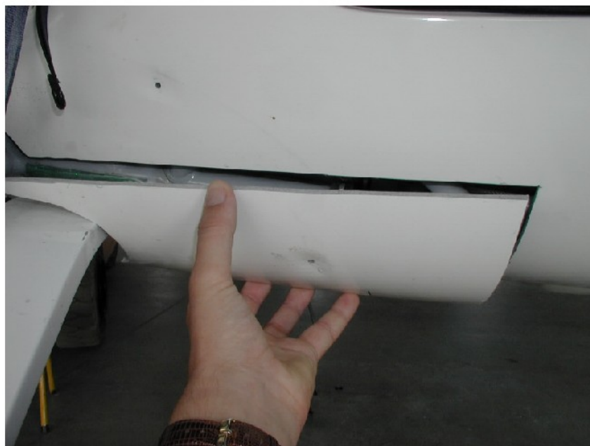
Figure 5: cut fuselage shell
