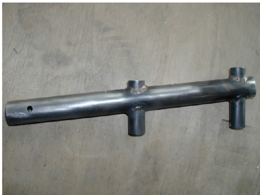
Figure 8: new tube supporting main landing gear leg
