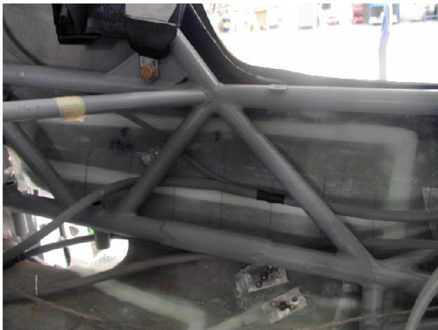
Figure 14: filling of gaps with filler material and lamination form inside and outside (gussets are not shown)
