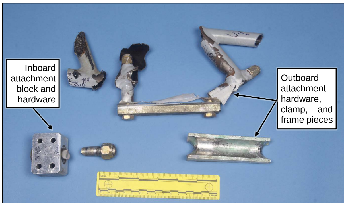
Figure 1. Overall view of the submitted RMLG attachment hardware, clamp, block, and fuselage frame pieces.
