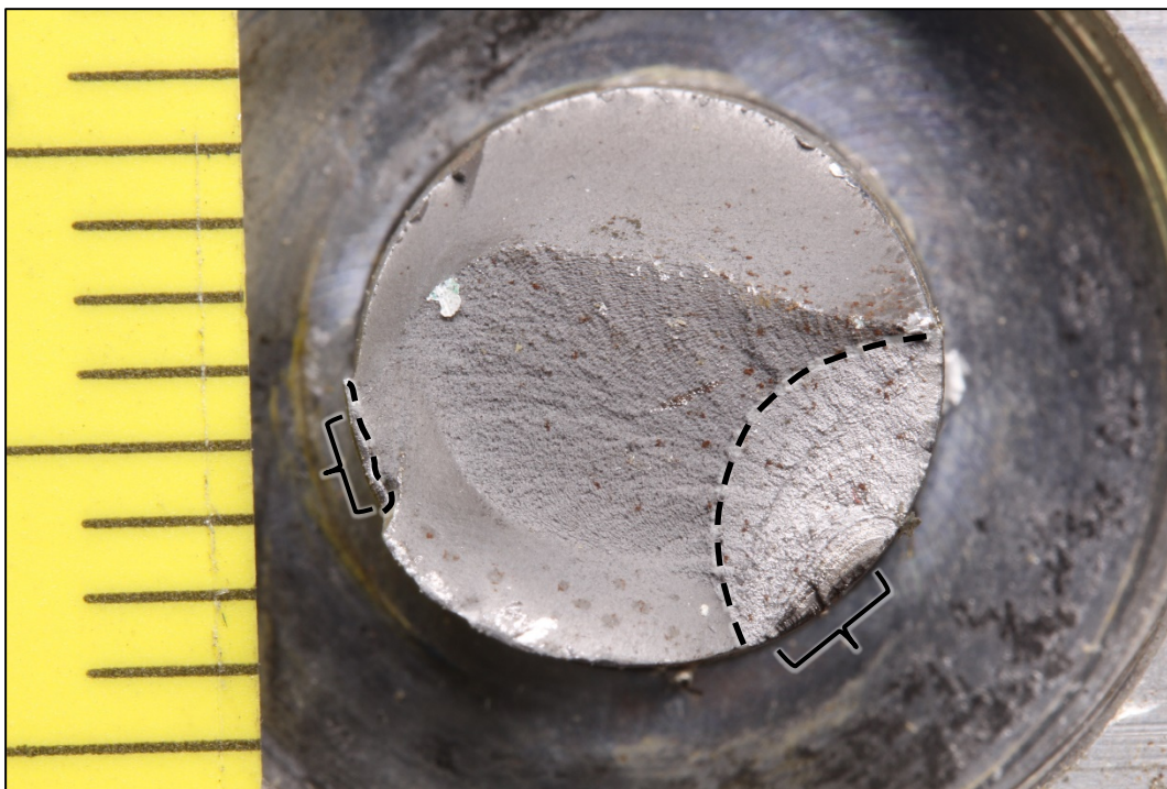
Figure 3. Upper fracture face on the RMLG inboard attachment bolt. Dashed lines indicate fatigue boundaries, and unlabeled brackets indicate fatigue origin areas.
