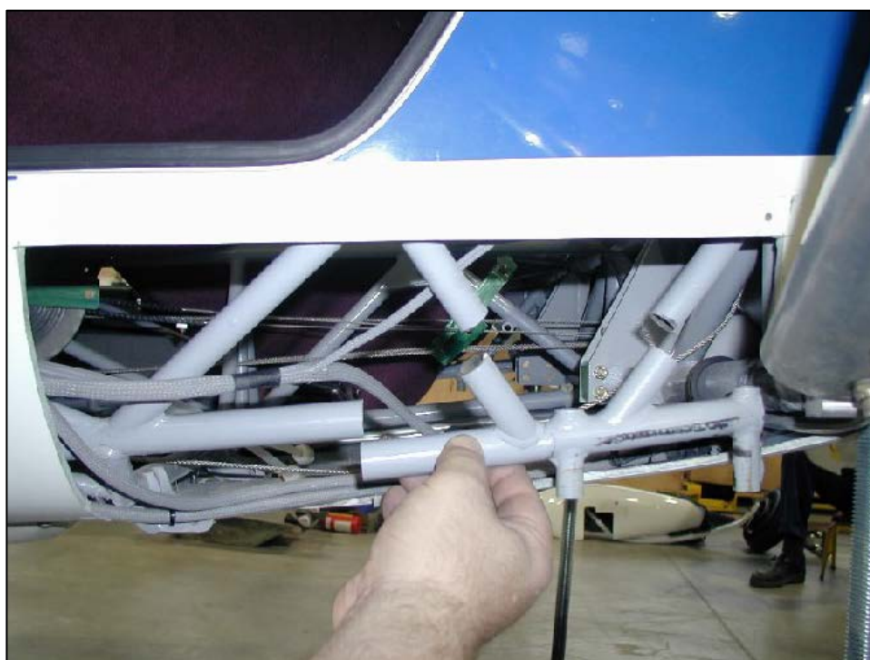
Figure 15. Image from OMF Process Specification PS-OMF 100-0006 showing the frame piece cut from the left side of the fuselage of an exemplar airplane being repaired.
