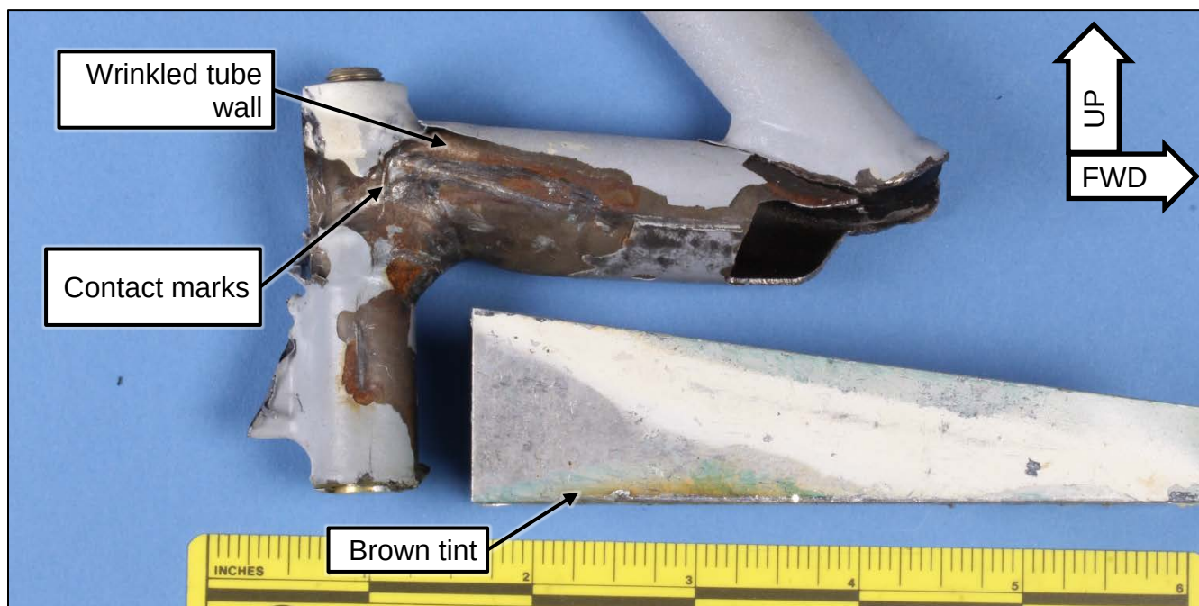
Figure 12. Outboard side of the sectioned frame piece and upper clamp. A wrinkle in the tube wall and marks consistent with contact with the upper corner of the displaced upper clamp are indicated. An area of brown tint is shown on the upper clamp.
