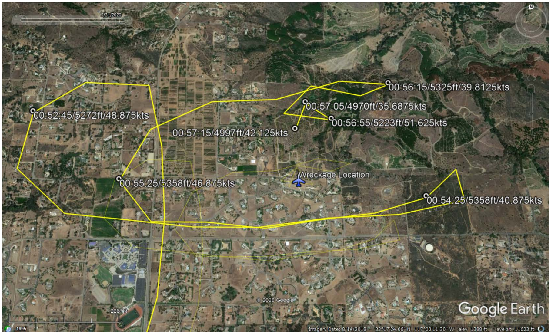
Figure 4. Google Earth overlay for the end of the accident flight recorded on the Dynon FlightDEK-D180.
