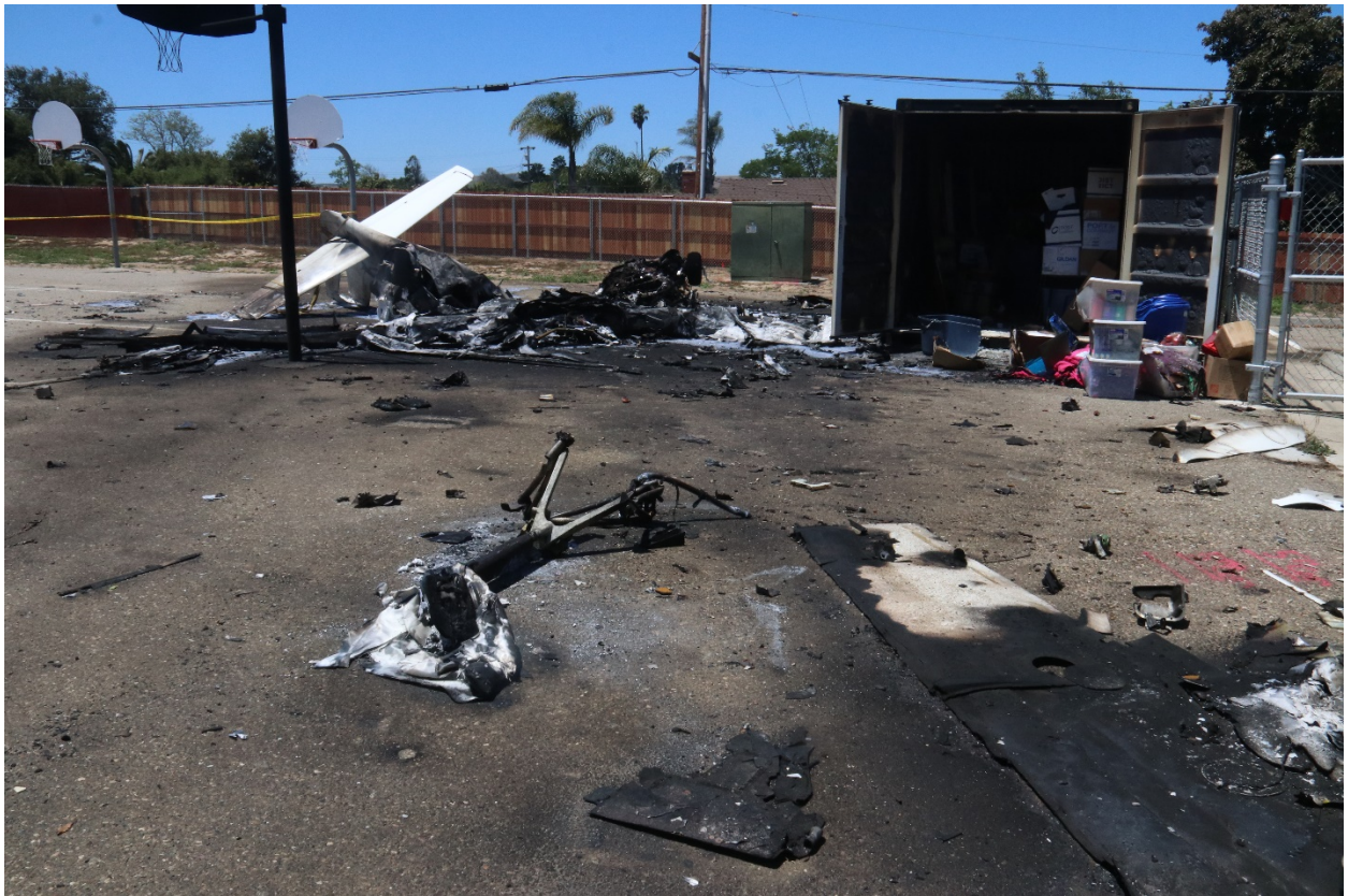
Figure 6: Wing Skin, Nose Landing Gear Assembly, and Main Wreckage.
