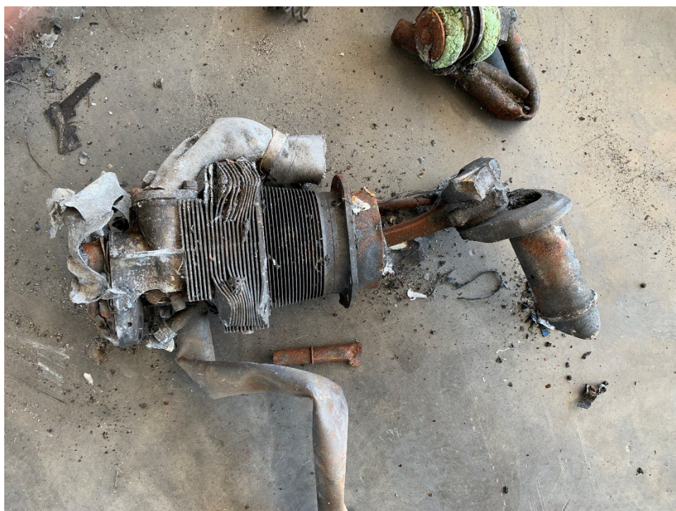
Figure 14: Number 6 Cylinder Assembly and Portion of Crankshaft
