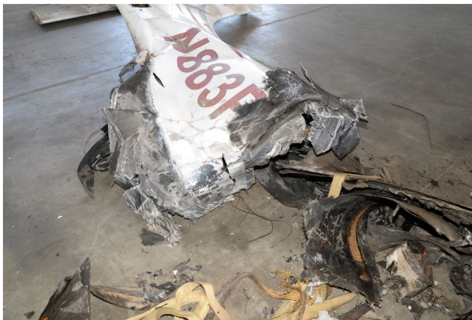
Figure 4: Aft Fuselage Immediately Infront of the Empennage
