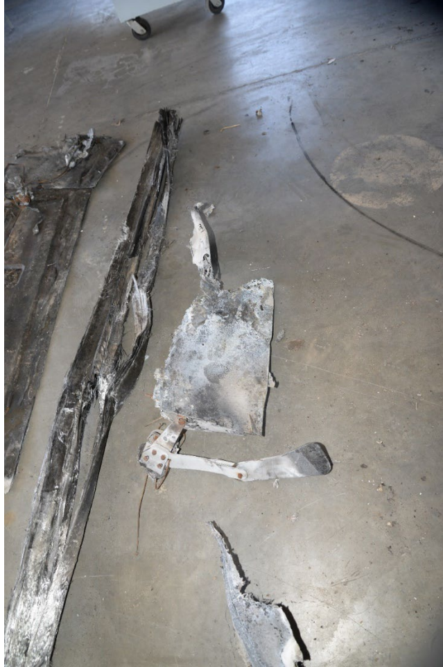
Figure 3: Right side Aileron Fragment and Wing Spar
