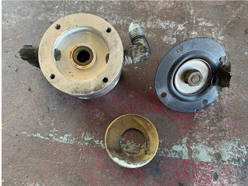
Figure 15: Fuel Manifold Valve
