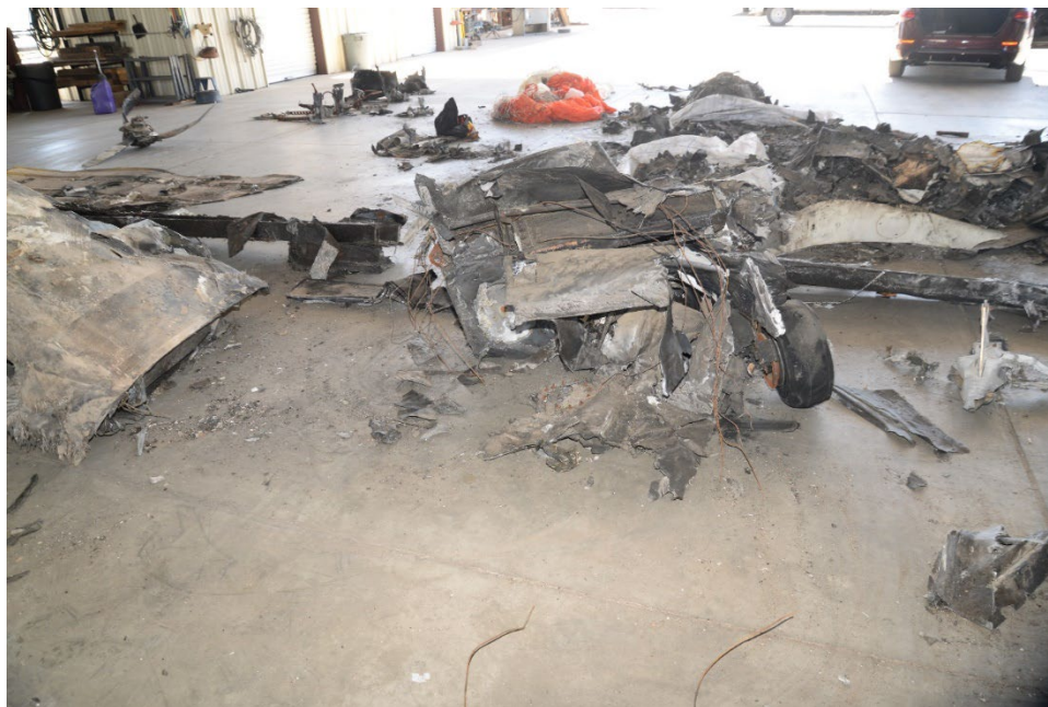
Figure 2: Center Fuselage and Wing Spar
