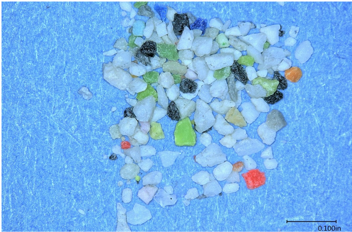
Figure 5 – The solid debris from the bag marked governor body outlet bore, after cleaning with acetone.
