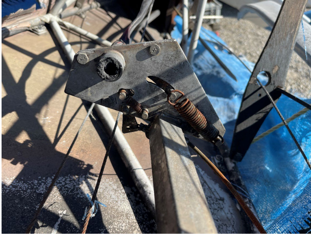
Figure 1: View of the airframe tow rope cutting mechanism.
