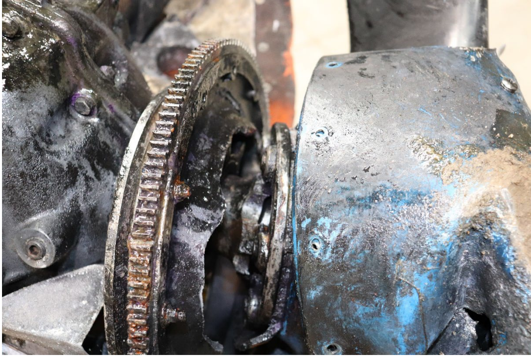
Figure 4. View of starter ring gear and crankshaft propeller flange damage
