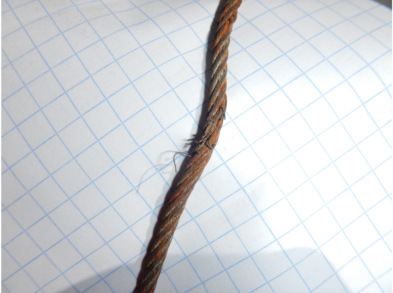
Figure 14. Example of the multiple broken wires found in the aileron control cables. Photo courtesy of Piper Aircraft.
