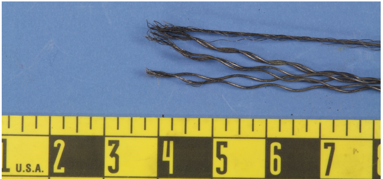
Figure 7 – View of the fractured control cable strands.
