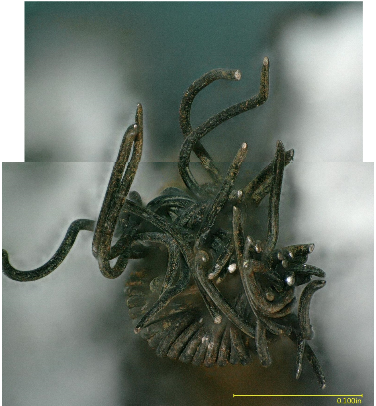
Figure 11 – Montage view of the 4 th and 5 th wire strand sets from the fractured cable.
