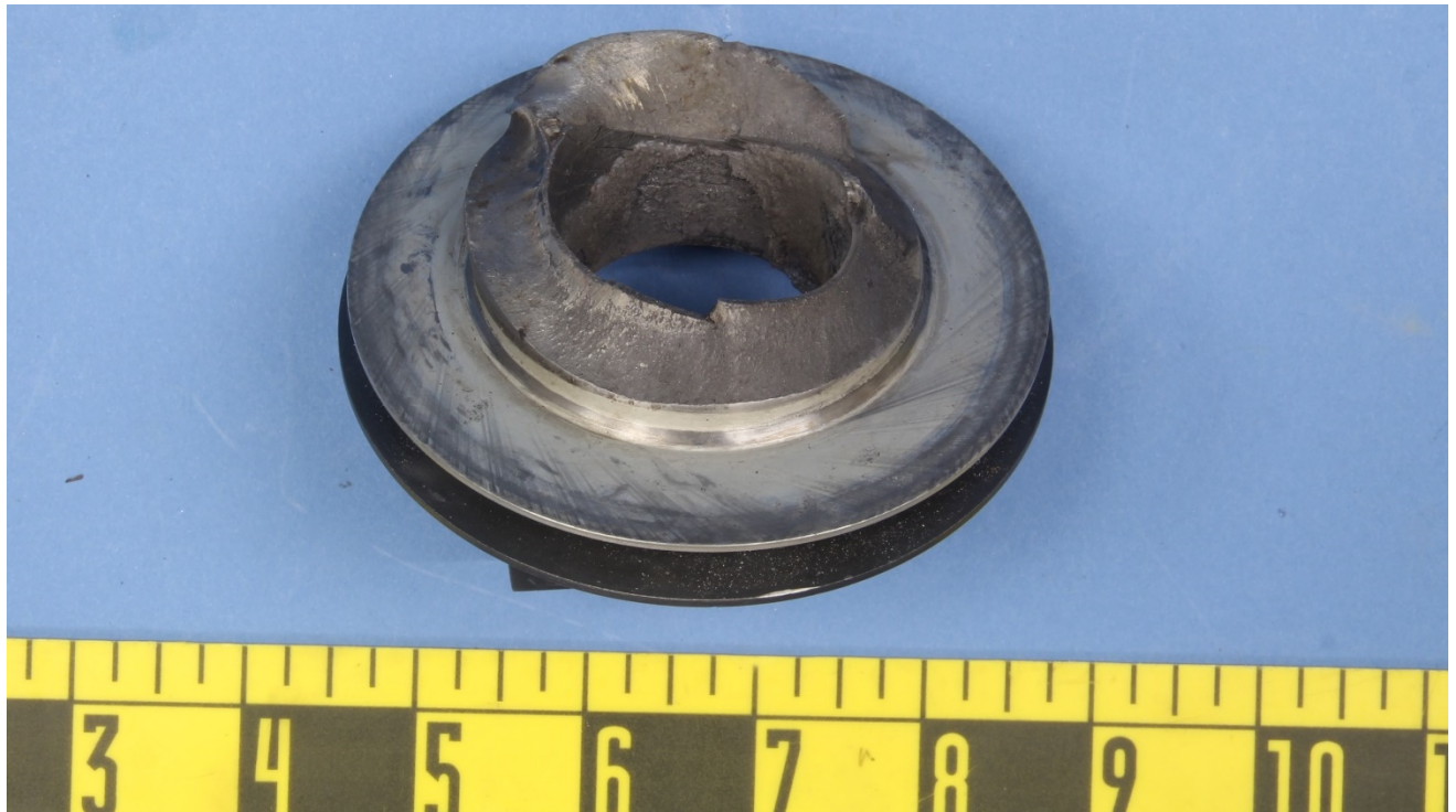
Figure 2 – The flange remnant, viewed from an angle, showing the angled fracture surface.
