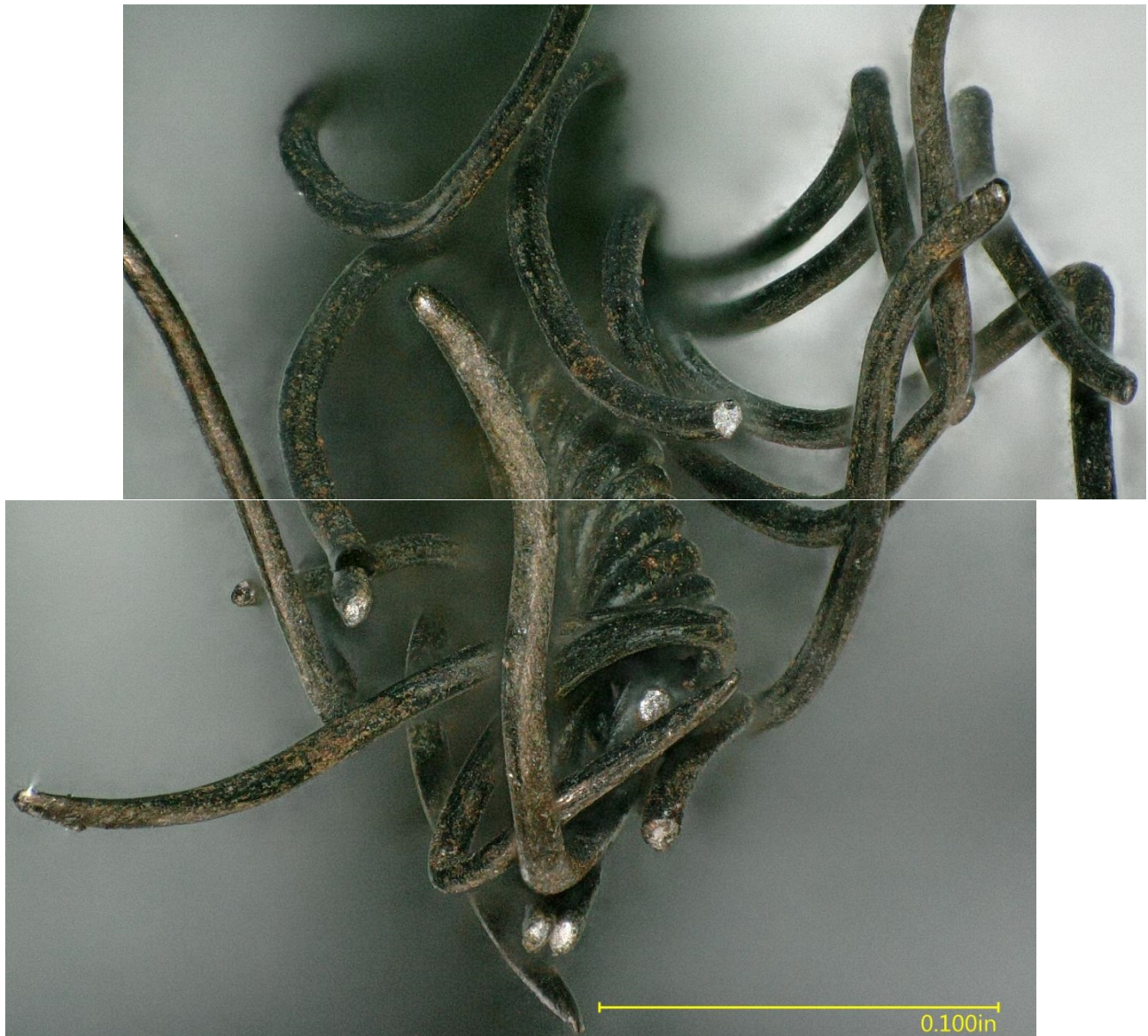
Figure 8 – View of some of the fractured wires from the frayed strand of the cable fracture.
