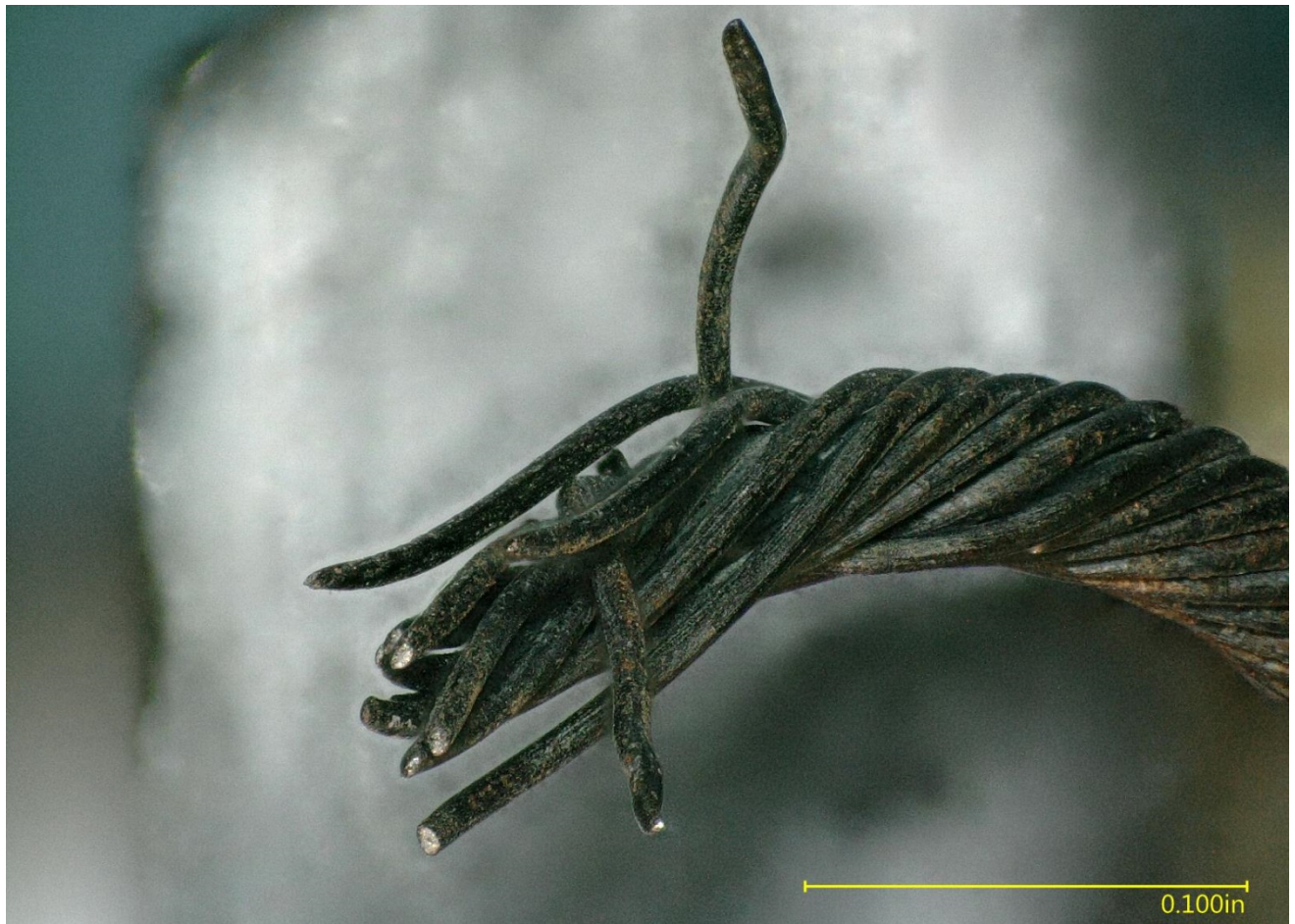
Figure 10 – View of the third set of wire strands on the fractured cable.
