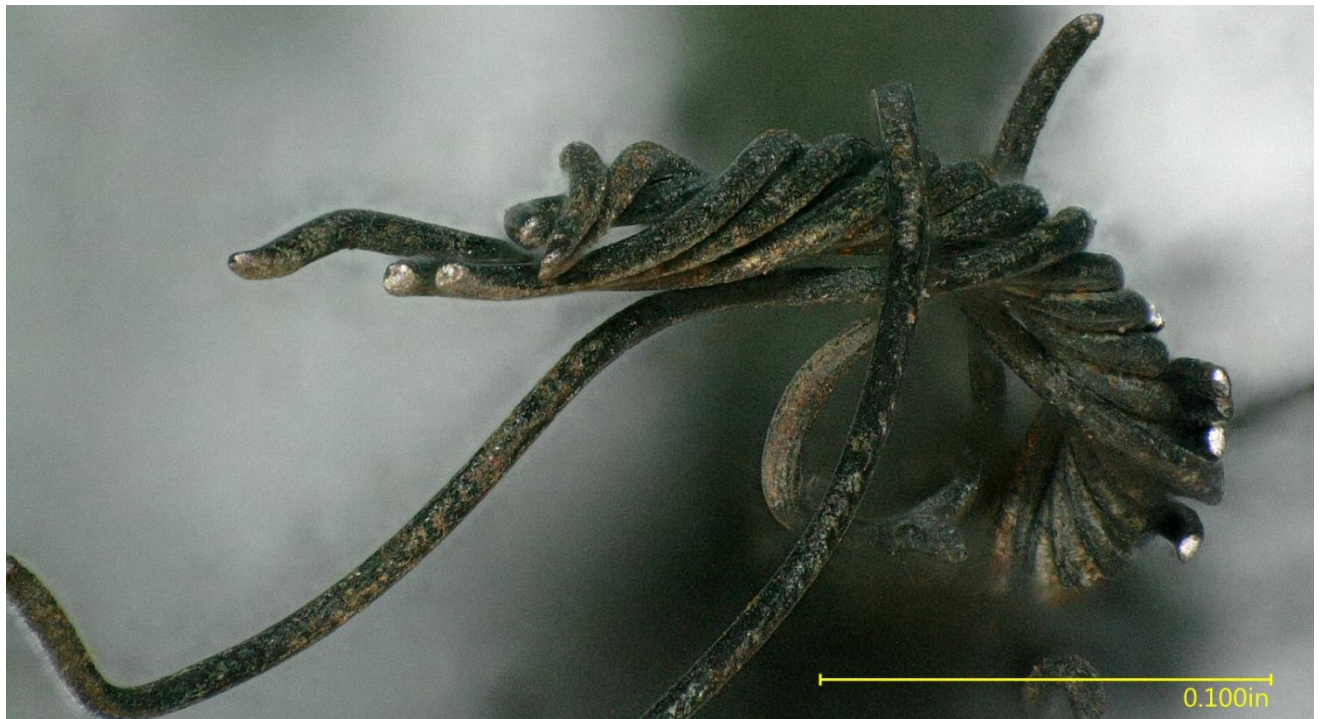
Figure 9 – View of the second strand of frayed wires on the fractured cable.
