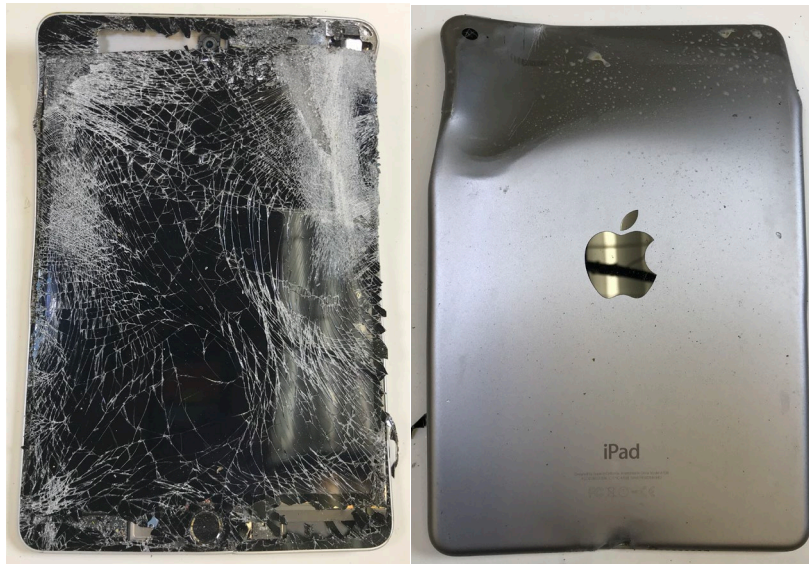
Figure 1. Front and back of the iPad Mini 4 as received.
