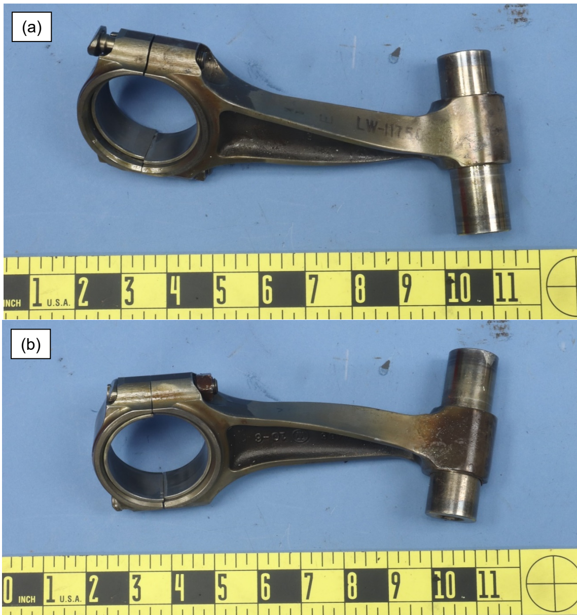
Figure 3 – View of the connecting rod recovered from the #3 cylinder, showing a 90° twist from (a) the marked flange face and (b) the opposite flange face.
