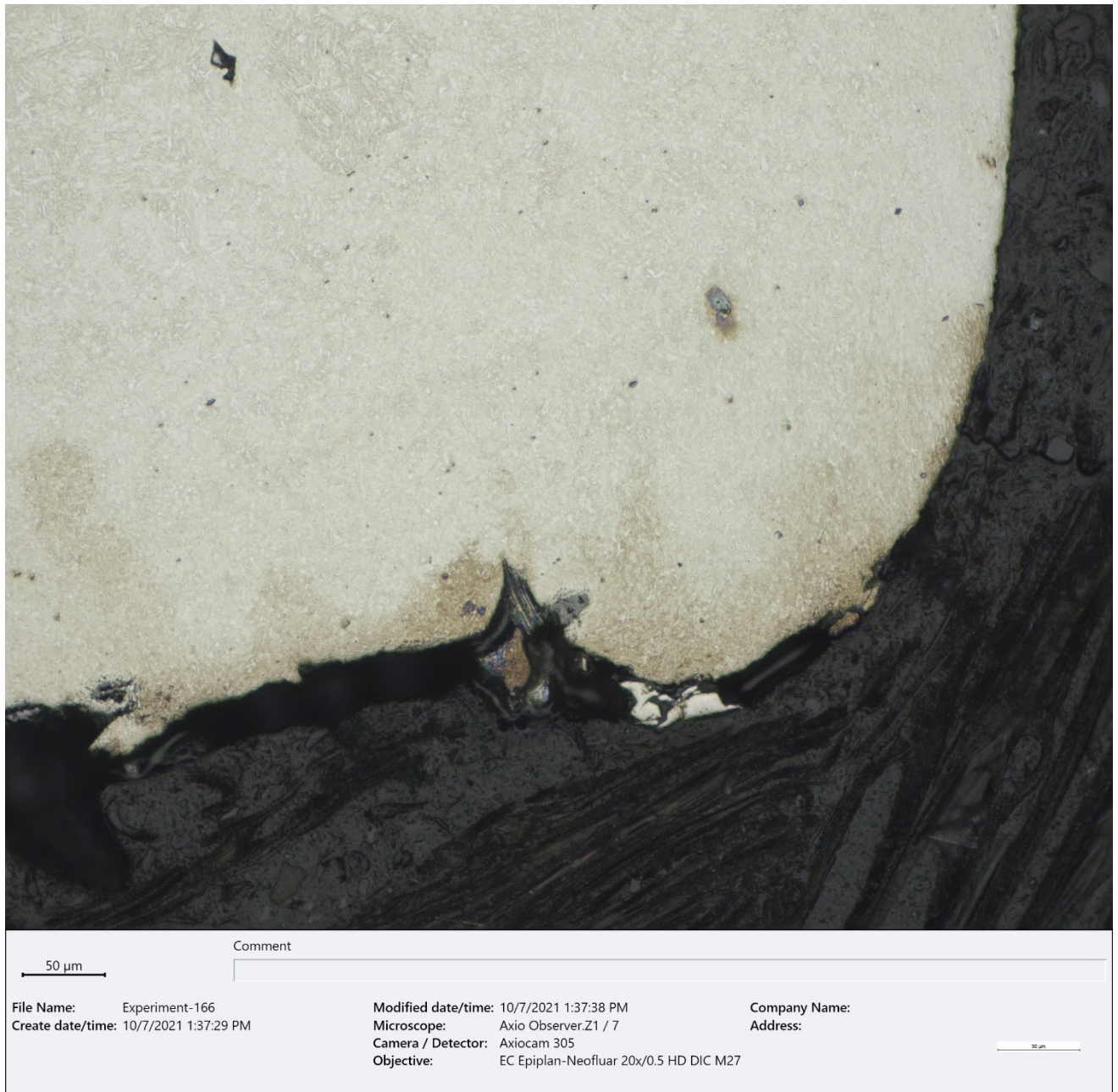
Figure 26 – BF micrograph of a closer view of the initiation site corner (~200X, etched 2% Nital).
