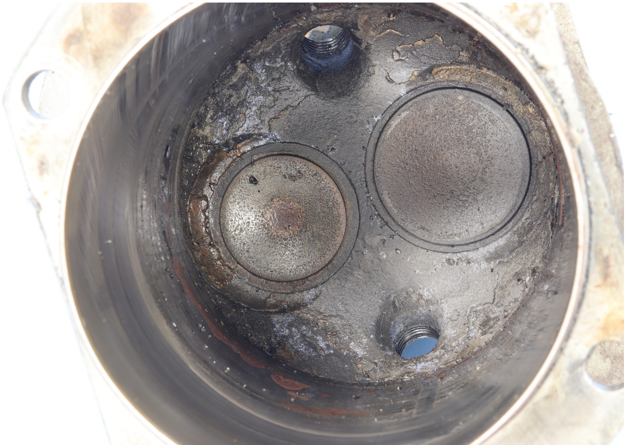
Figure 6 – View of the interior bore surfaces and valve seats of the #4 cylinder after removal of the piston and spark plugs.
