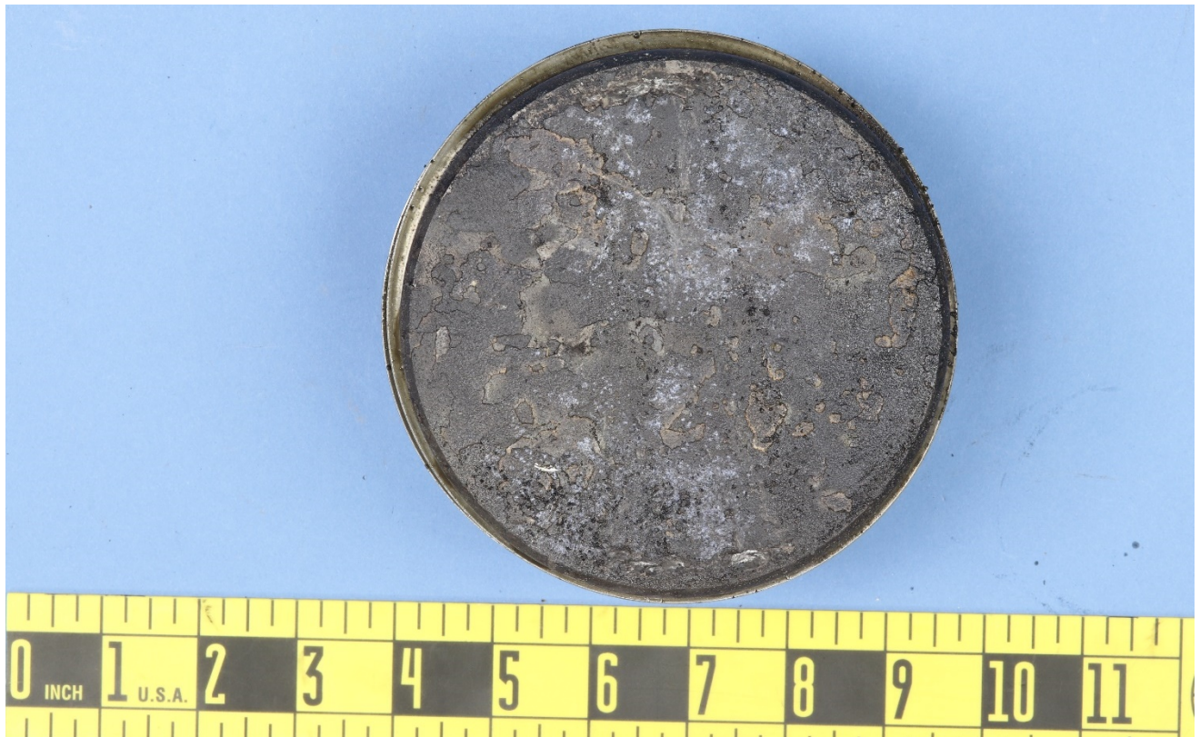
Figure 7 – View of the #4 piston crown, after removal. The surface exhibited deposits consistent with combustion products thick enough to begin spalling.
