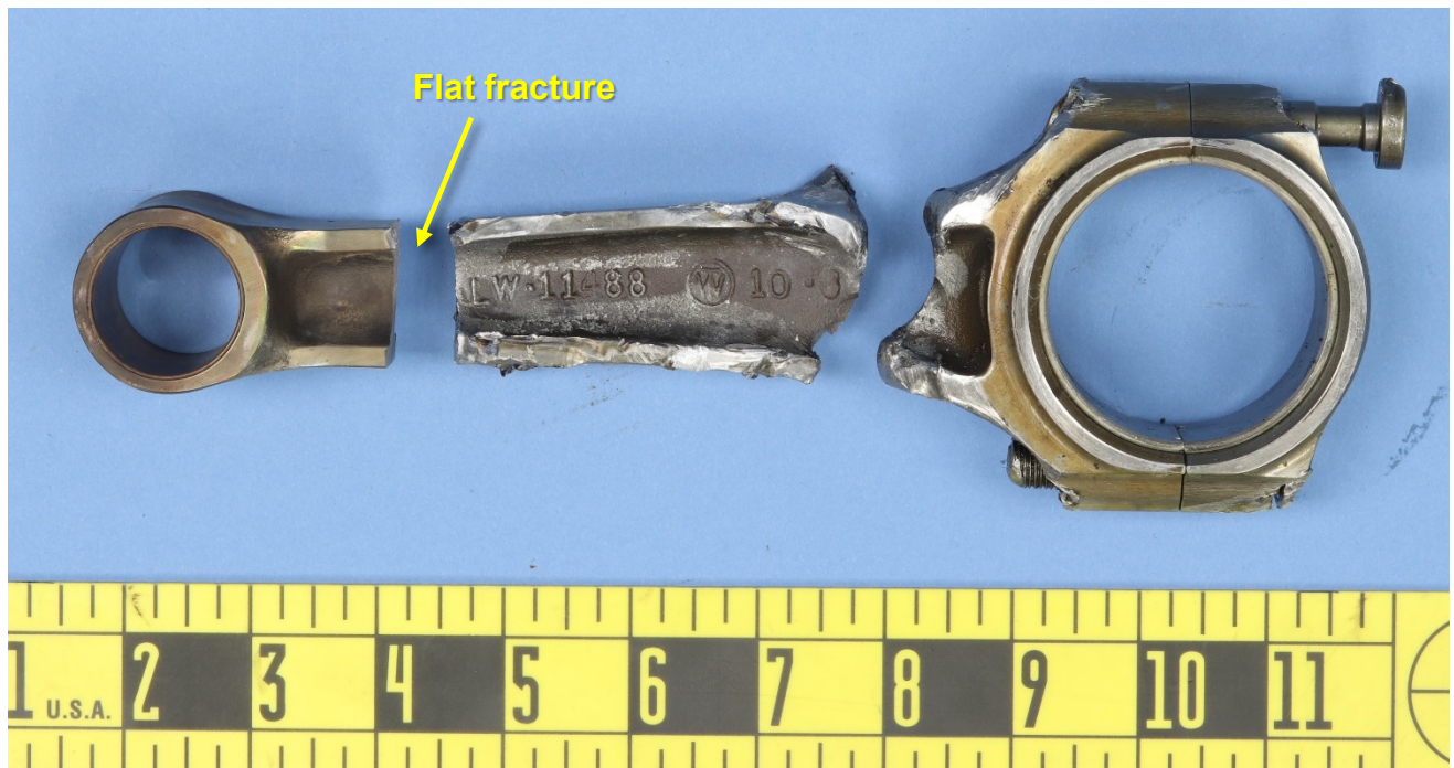
Figure 9 – View of the #4 connecting rod remnants, positioned after removal of the pin remnant from the piston, viewed from the marked web side.
