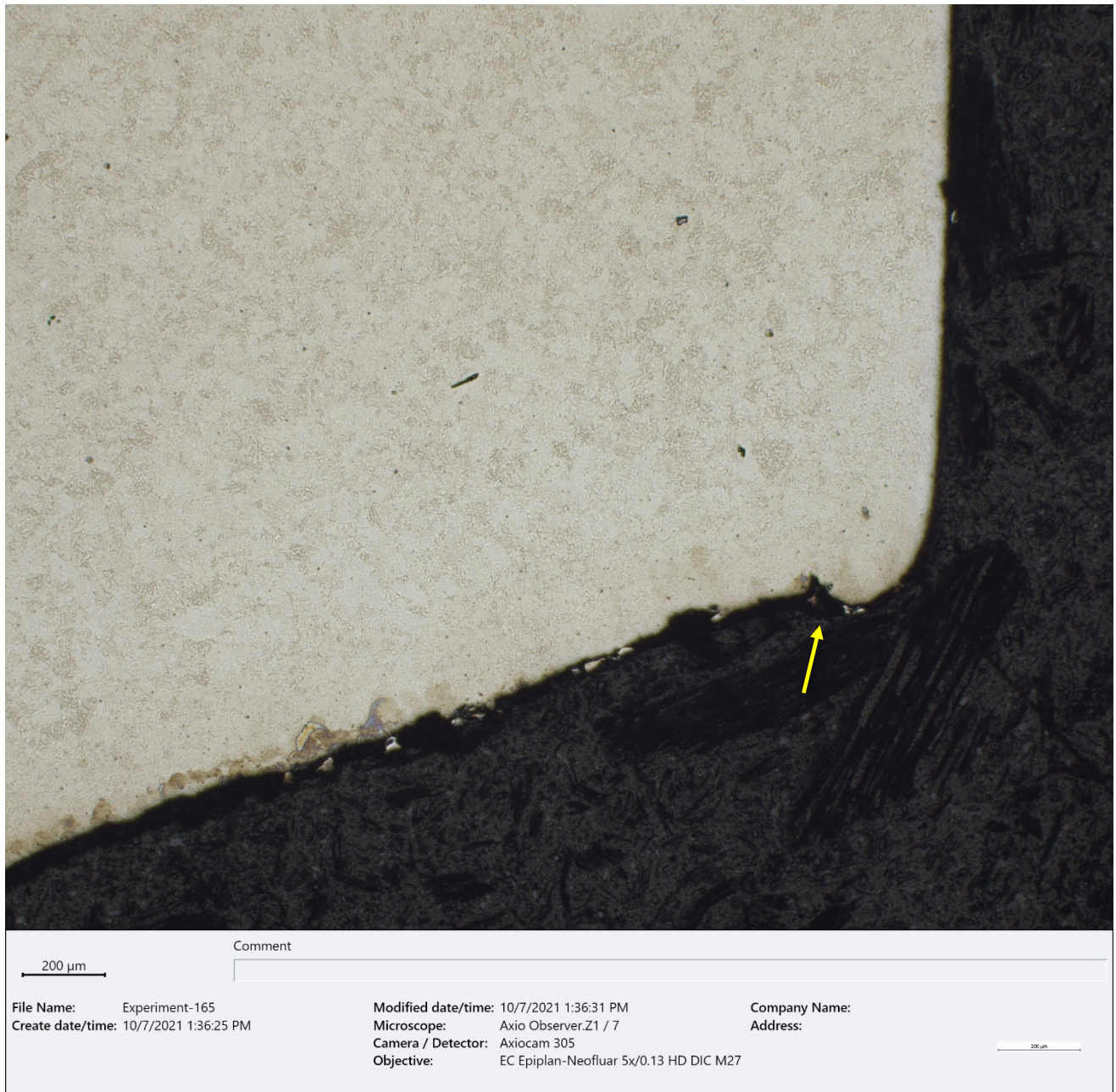
Figure 25 – Bright-field (BF) optical micrograph of the cross section through the crack initiation site (~50X, etched 2% Nital).
