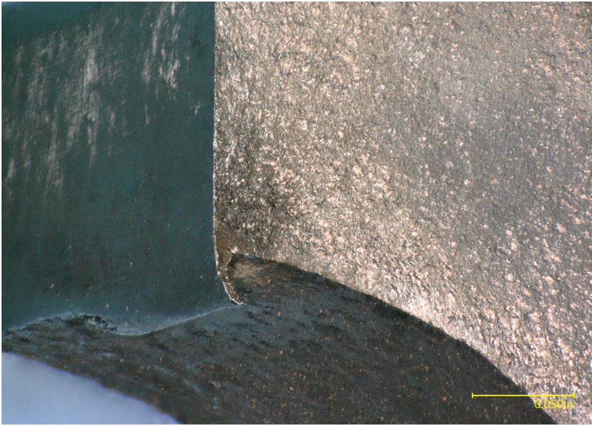
Figure 15 – Side angle view of the crack initiation site.
