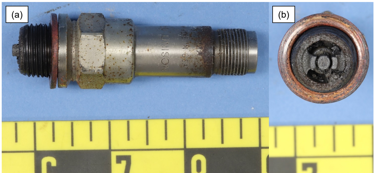
Figure 8 – View of the #4 spark plug after removal from (a) the side and (b) the electrode.
