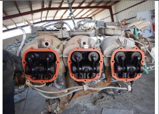
Figure 6-Right cylinder's overhead components.
