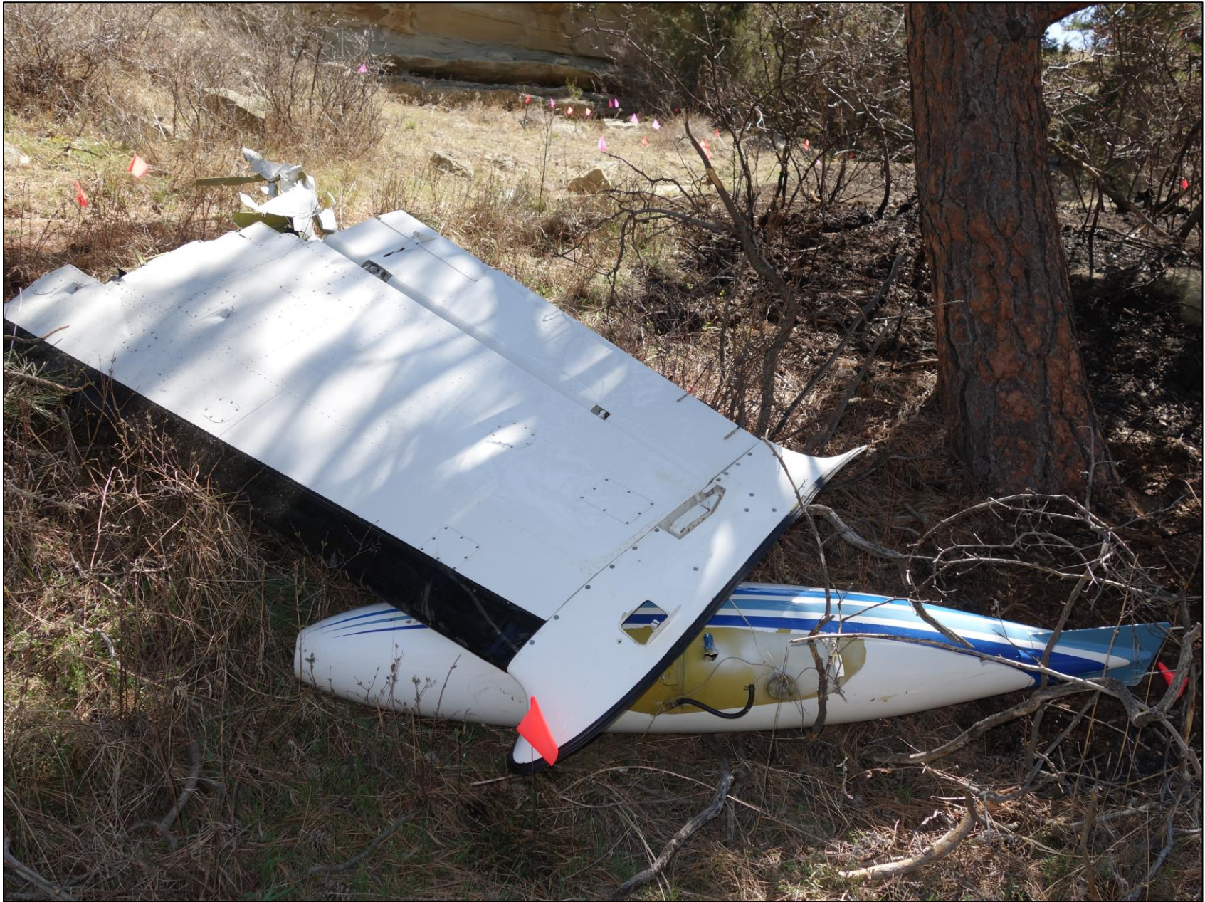
Photo 6 – Right outboard wing section and tip tank. (Courtesy of the FAA)
