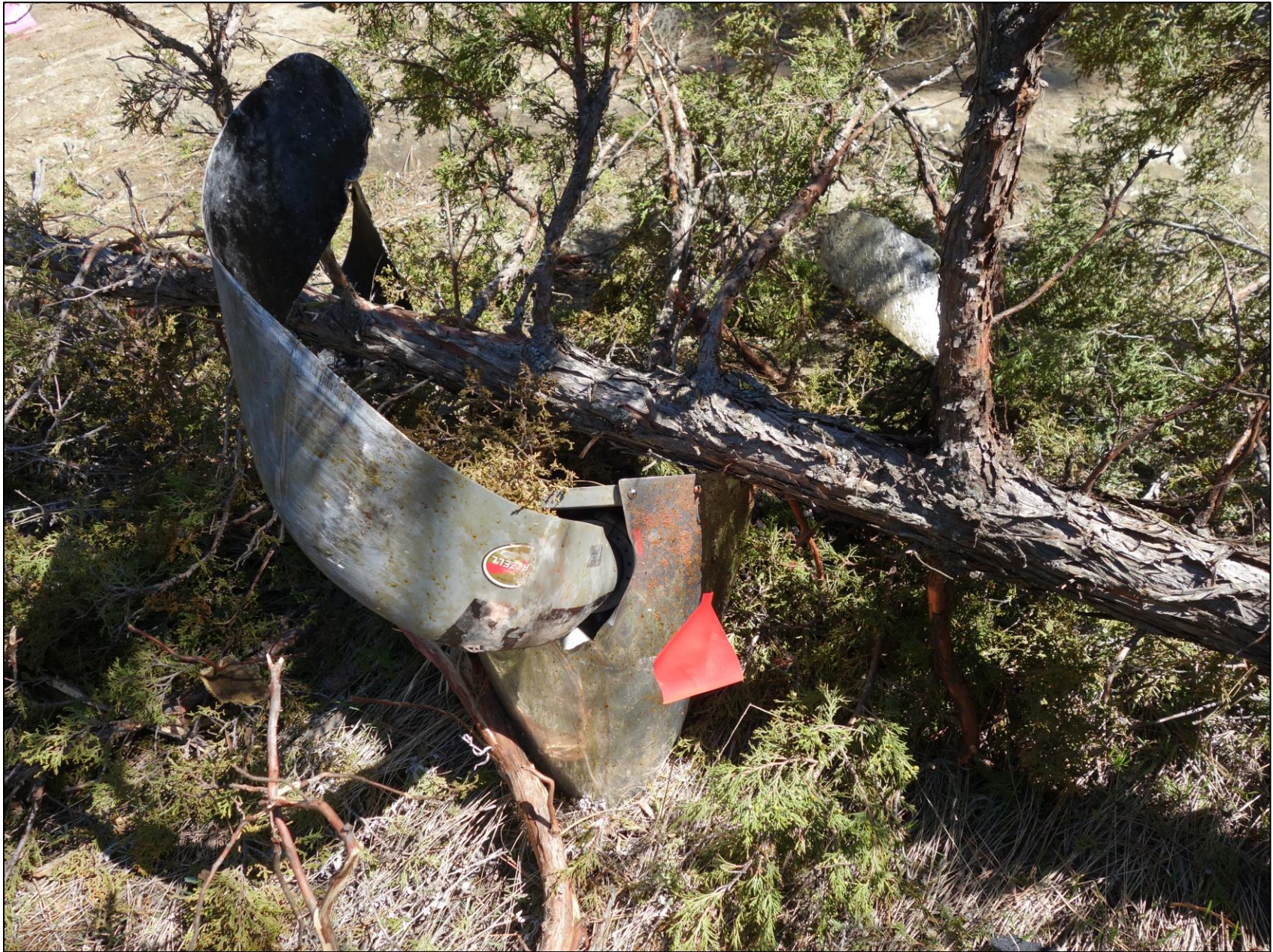
Photo 10 – Accident site, left propeller assembly. (Courtesy of the FAA)
