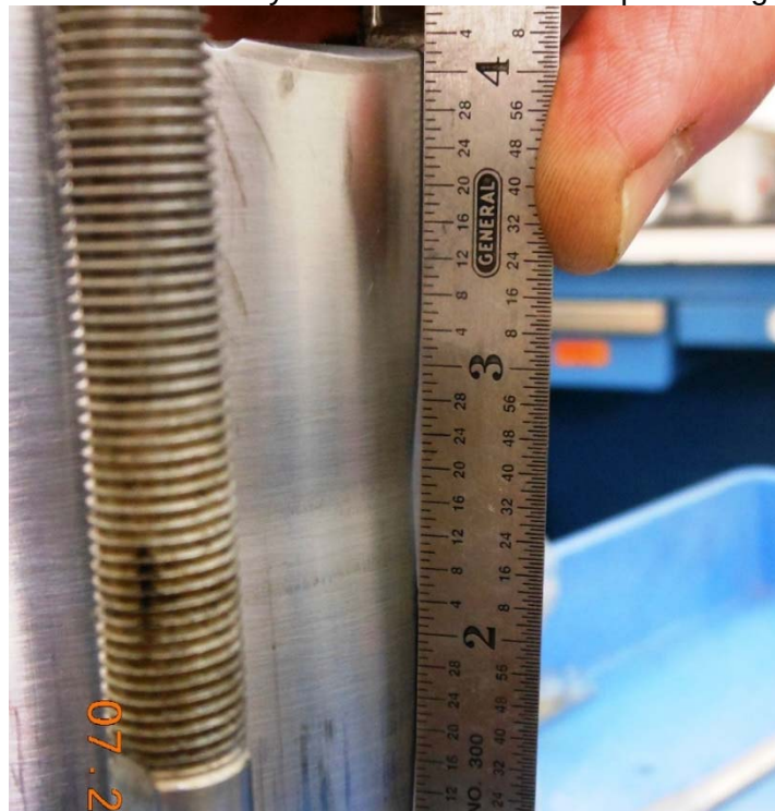
Photo #23 – Left cylinder crease/dent from piston edge
