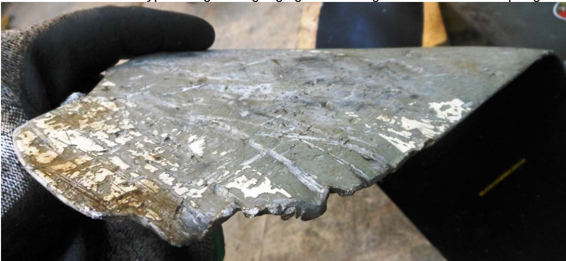
Photo #27 – Blade L3 typical degree of gouging and scoring on camber side of tip region
