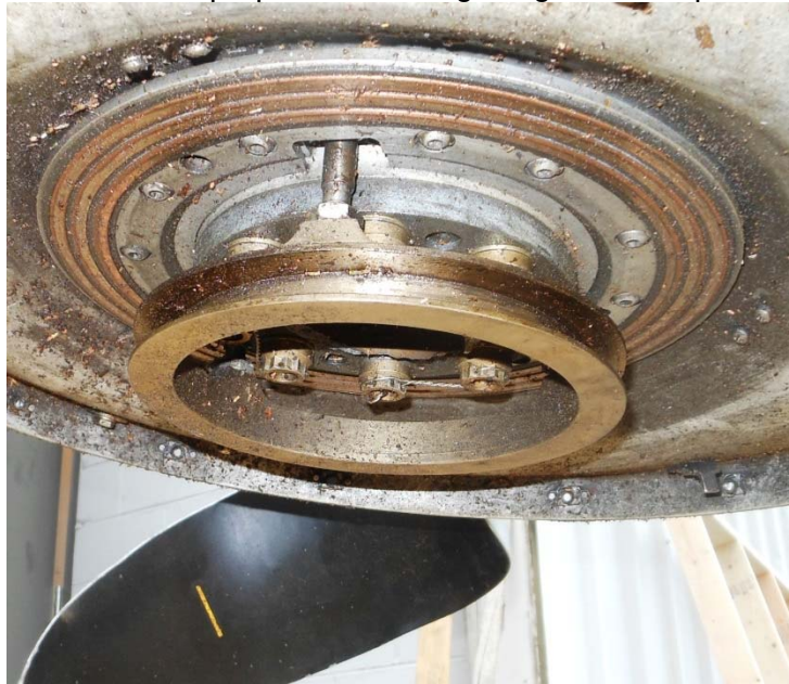
Photo #16 – Left propeller mounting flange area as-presented
