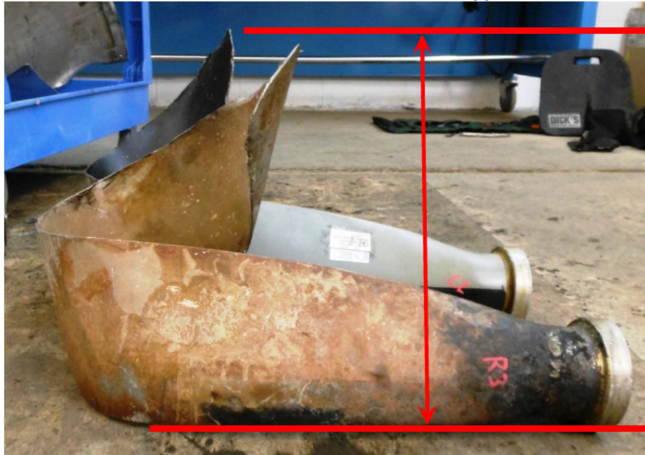
Photo #5 – Blades R3 and L2 amount of bend opposite rotation
