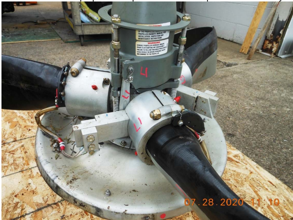
Photo #17 – Left propeller components numbered prior to disassembly
