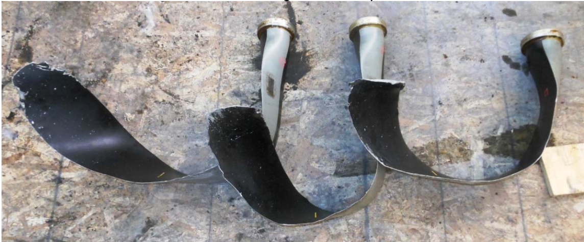
Photo #28 – Left blades trail-edge view, compound bend and twist
