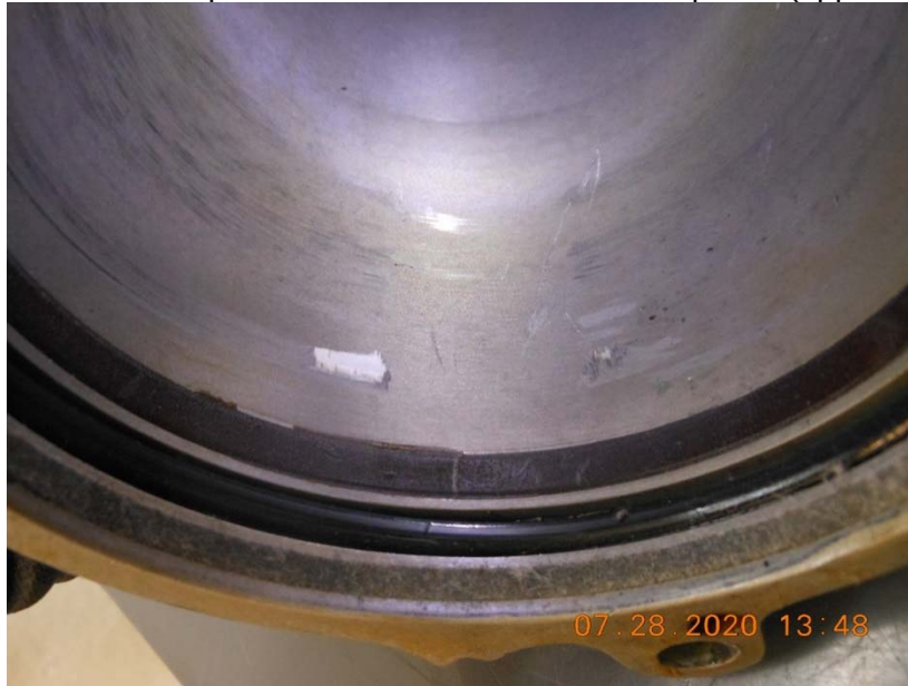
Photo #20 – Left impact marks on internal surface of piston (opposite side)
