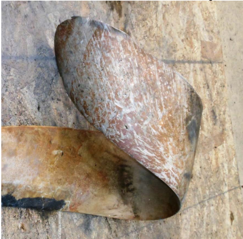
Photo #13 – Blade #R3 camber-side scoring
