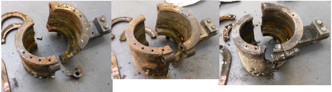
Photo #12 – Blade retention clamps
