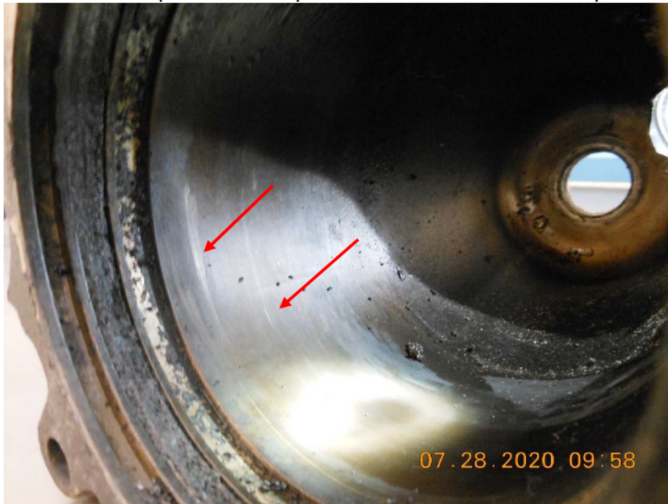
Photo #9 – Representative impact marks on internal surface of piston
