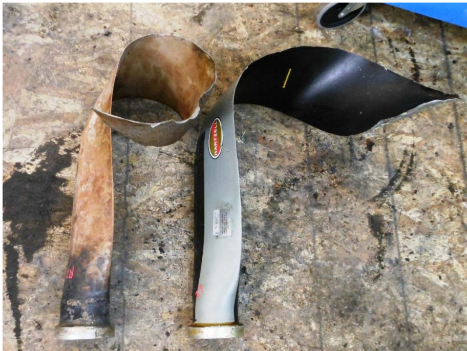
Photo #4 – Blades R3 and L2 relative bend and twist
