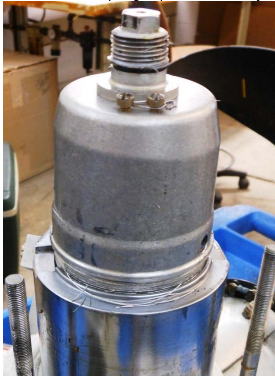
Photo #22 – Left forward spring cup forced from cylinder mount
