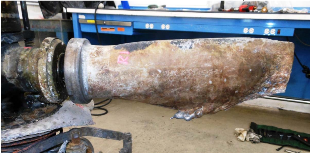
Photo #15 – Blade R1 could not be removed from hub/pilot tube
