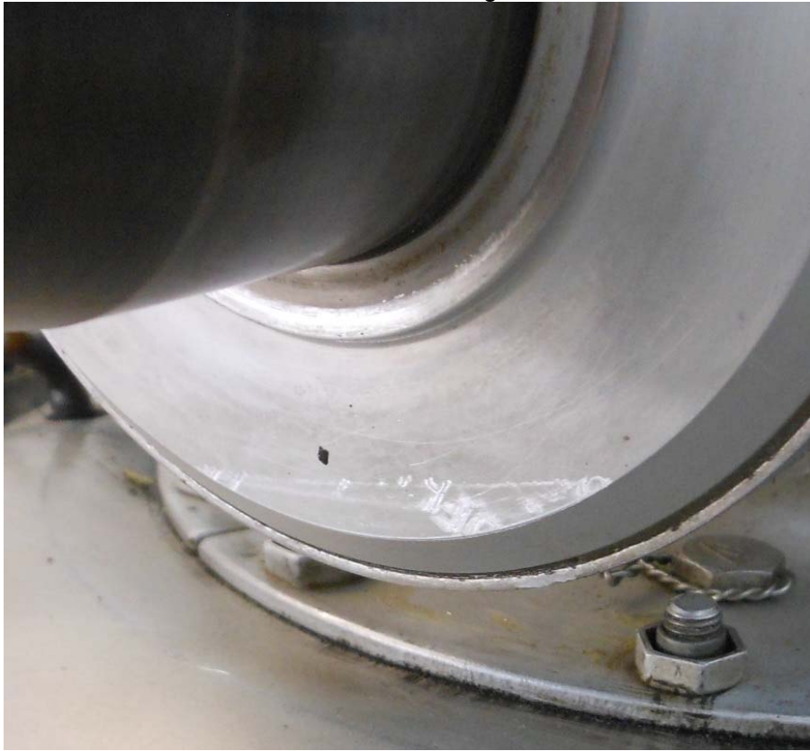
Photo #26 - Blade L1 hub arm flange letter transfer mark
