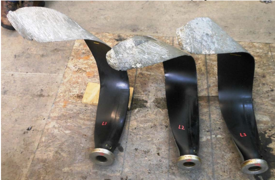
Photo #29 – Left blades camber side of tip region
