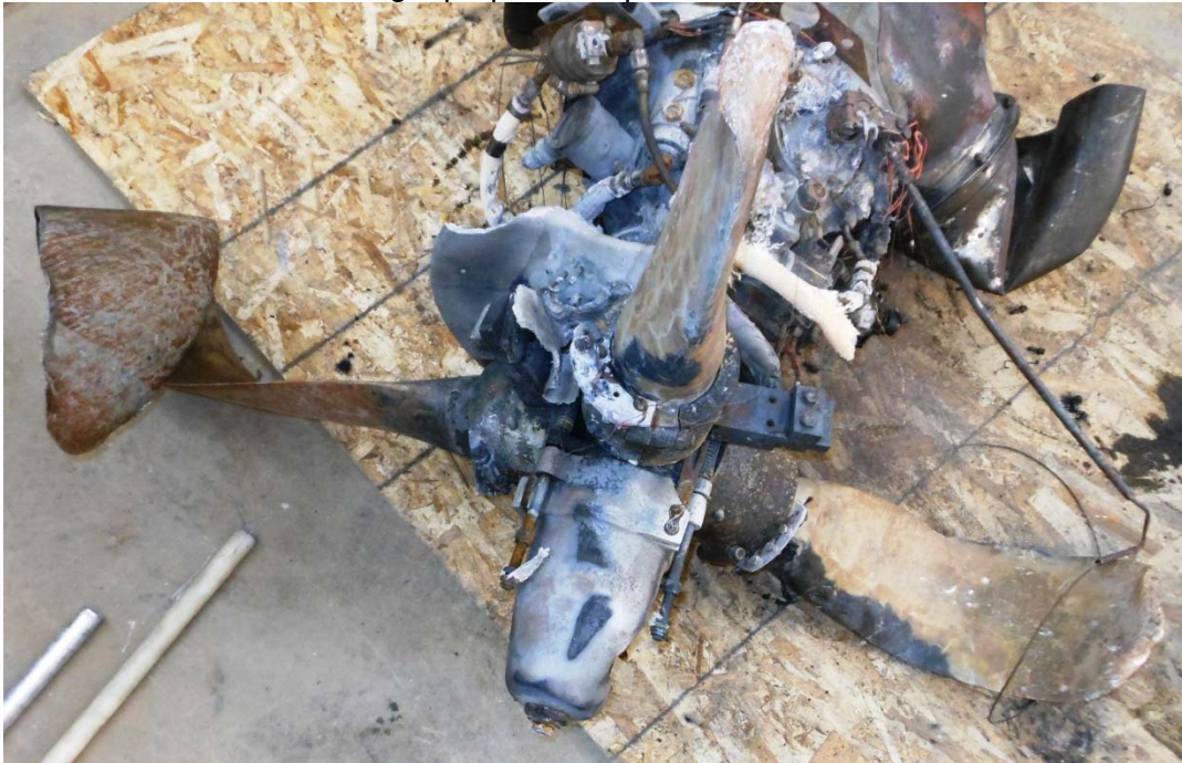
Photo #2 – Right propeller as-presented for examination
