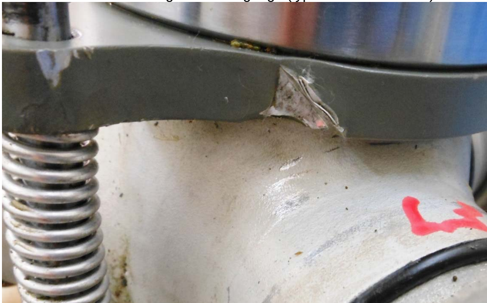
Photo #21 - Left guide collar gouge (typical three locations)
