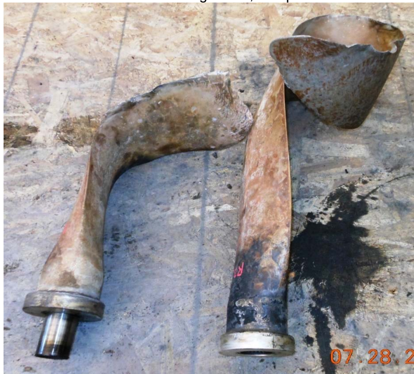
Photo #14 – R2 and R3 trail-edge view, compound bend and twist
