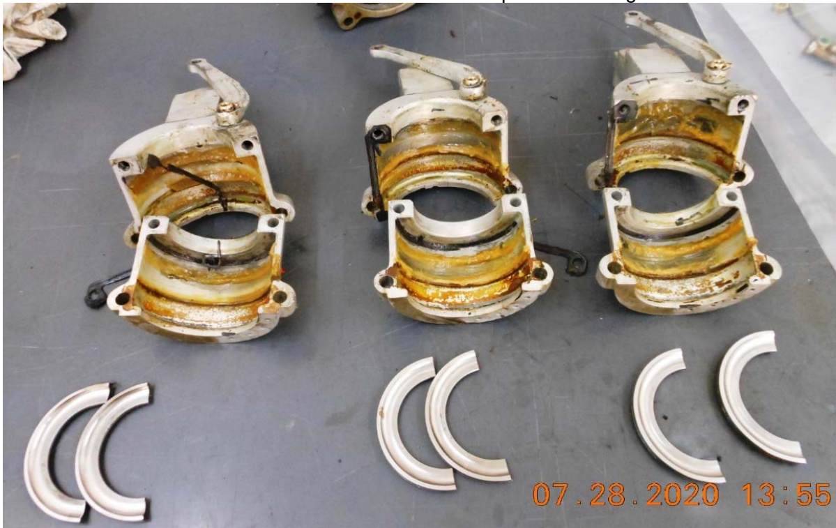
Photo #24 – Left blade retention clamps and bearings
