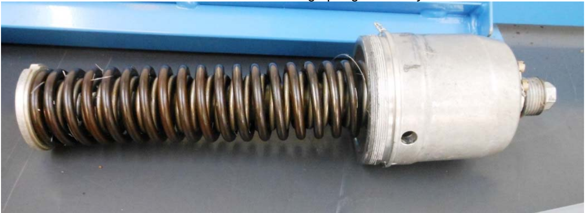
Photo #25 - Left feathering spring assembly
