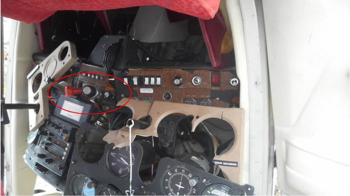
Figure 5: The Instrument Panel - The throttle, mixture, and carburetor heat were all pushed into the instrument panel.
