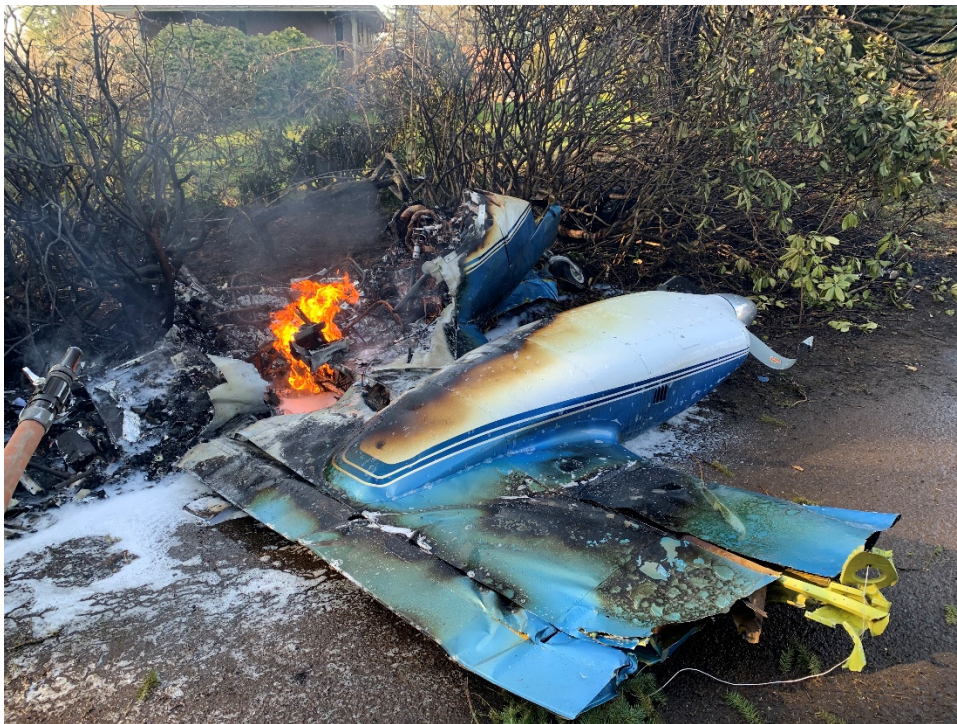
Figure 4: The Main Wreckage was Thermally Damaged
