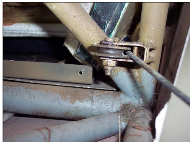
Figure 5-Right Rudder Cable and Pulley
