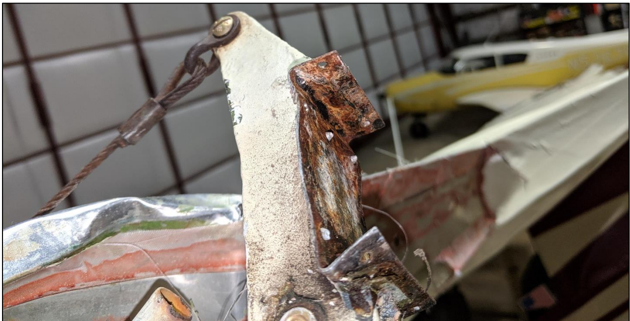
Figure 7-Left Aileron Bellcrank Aileron Attachment
