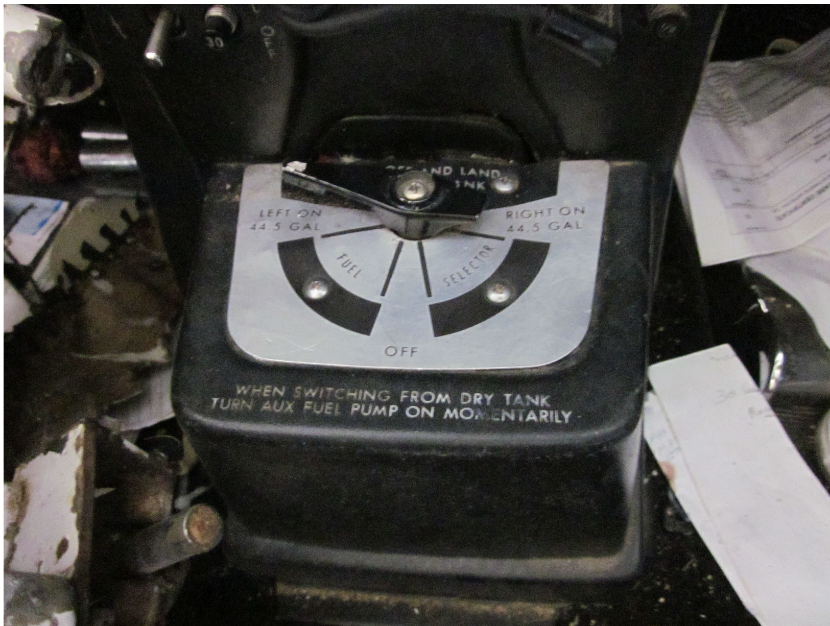
Photo 4 – Fuel selector (courtesy of Federal Aviation Administration)
