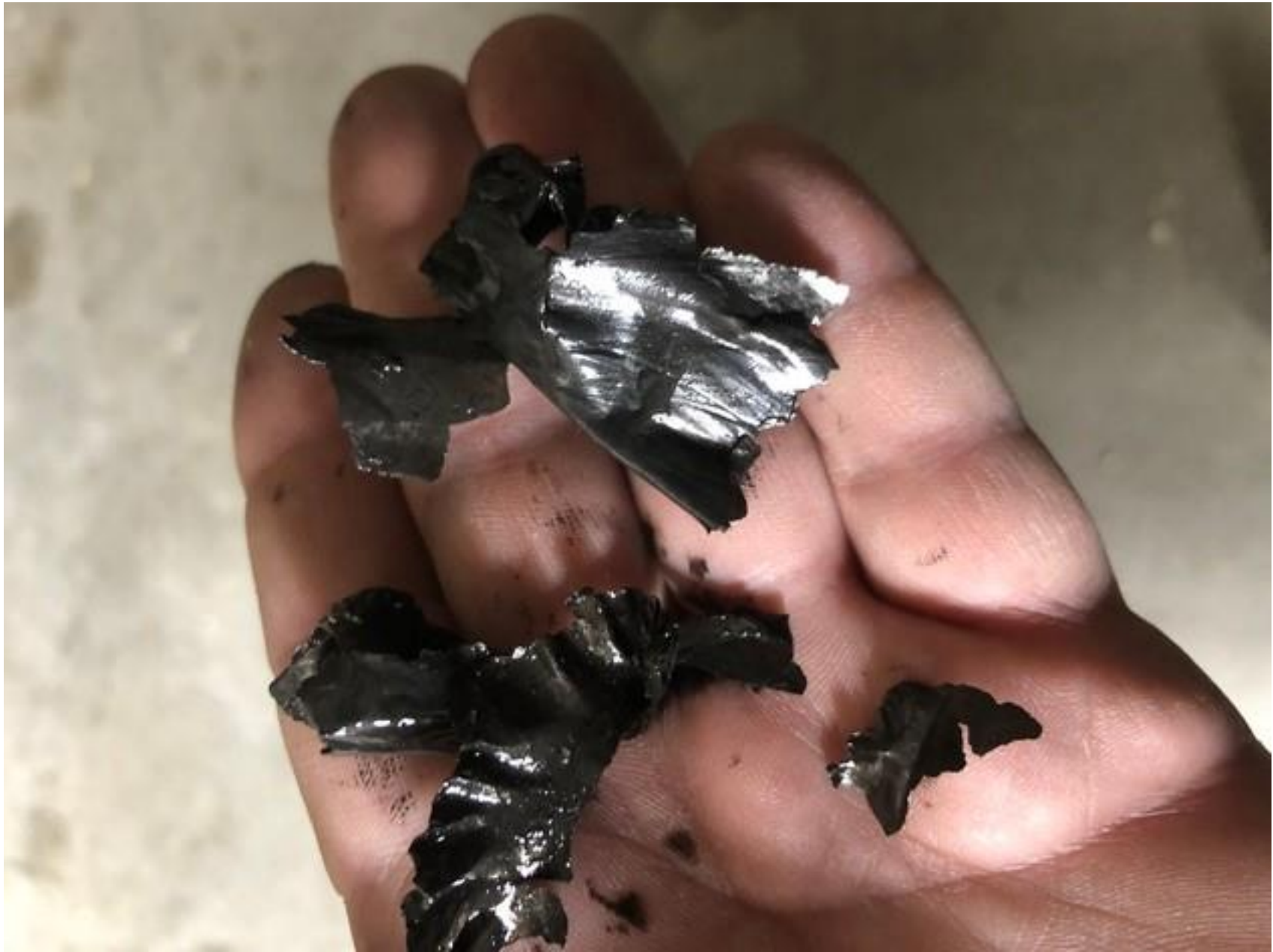
Photo 6 – No. 2 connecting rod bearing material. (Courtesy of the hired mechanic)
