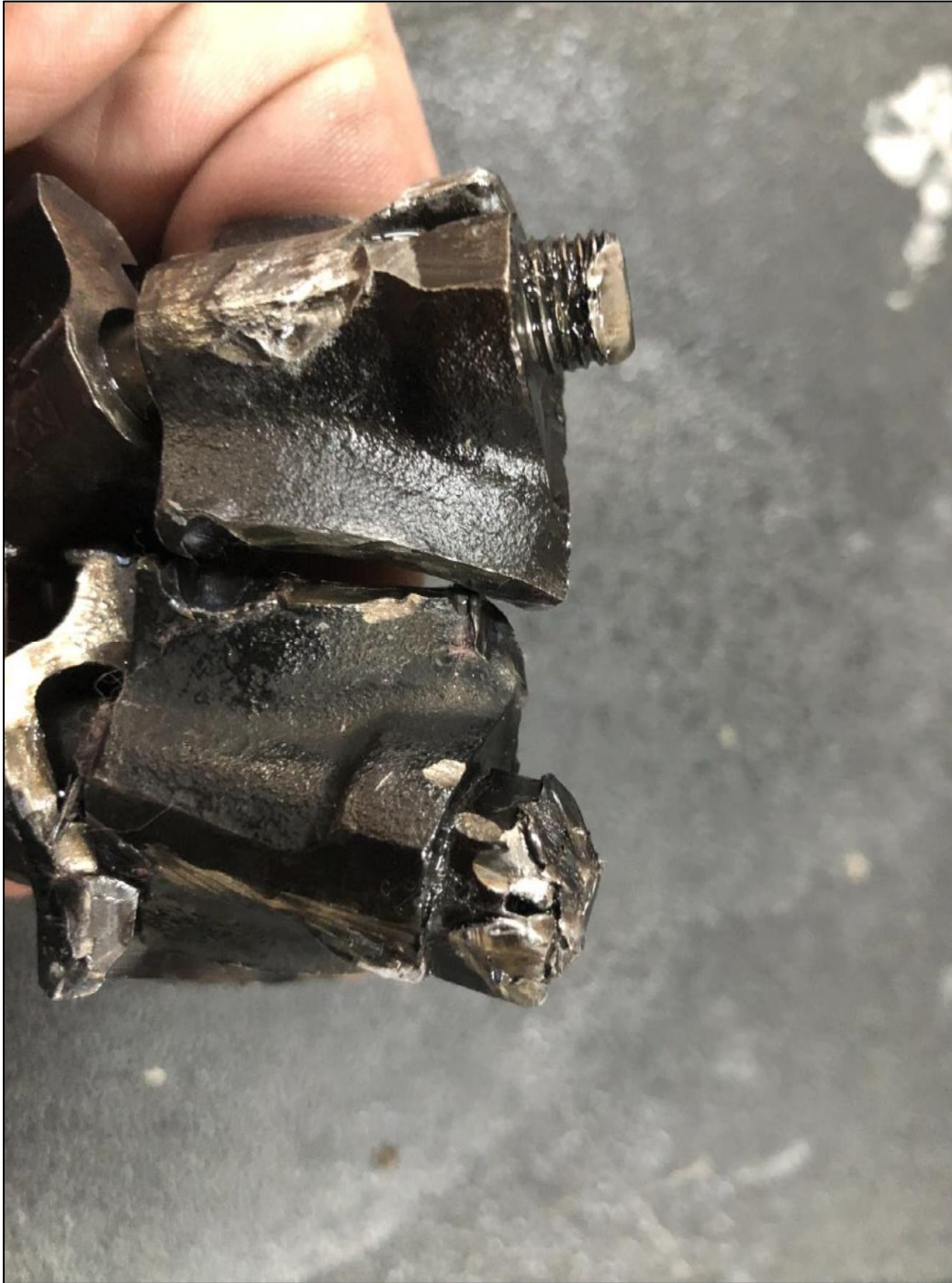
Figure 8-The No. 2 connecting rod end cap and yoke end sections.
