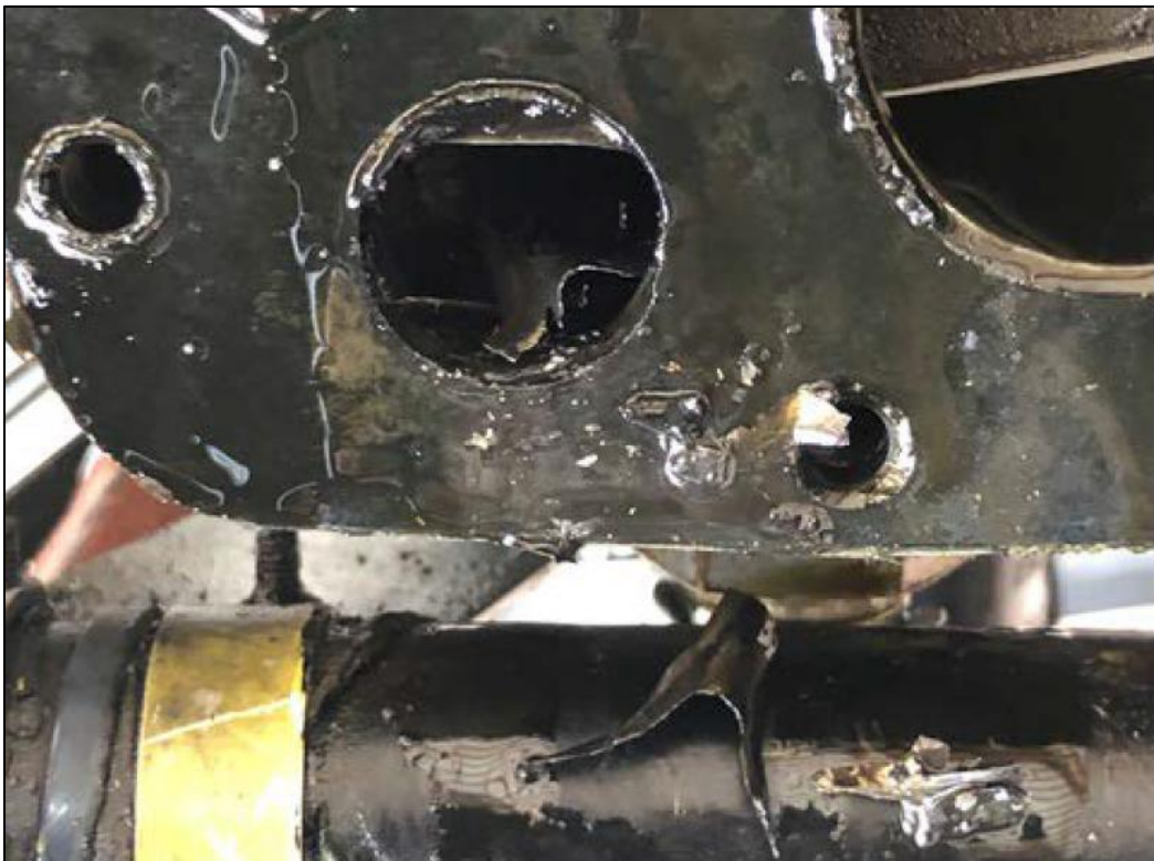
Figure 7-Oil pickup screen location and metal fragments.
