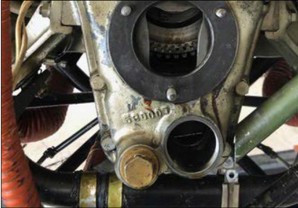
Figure 6-Accessory section and oil pickup screen location.
