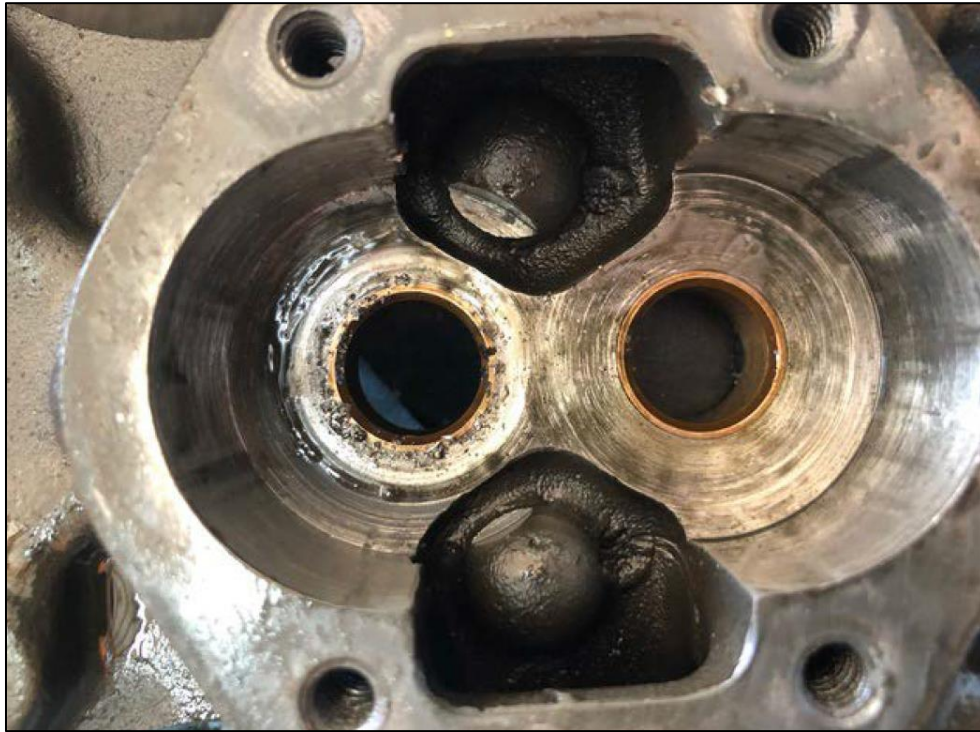
Figure 4-Oil pump gear cavity.
