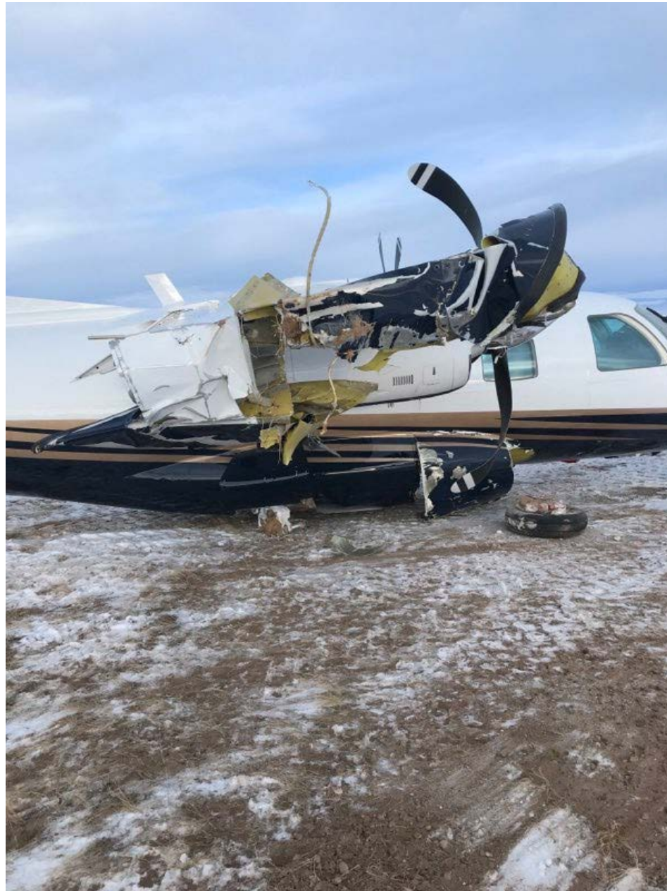
Photo 1 – Substantial damage to the right wing
