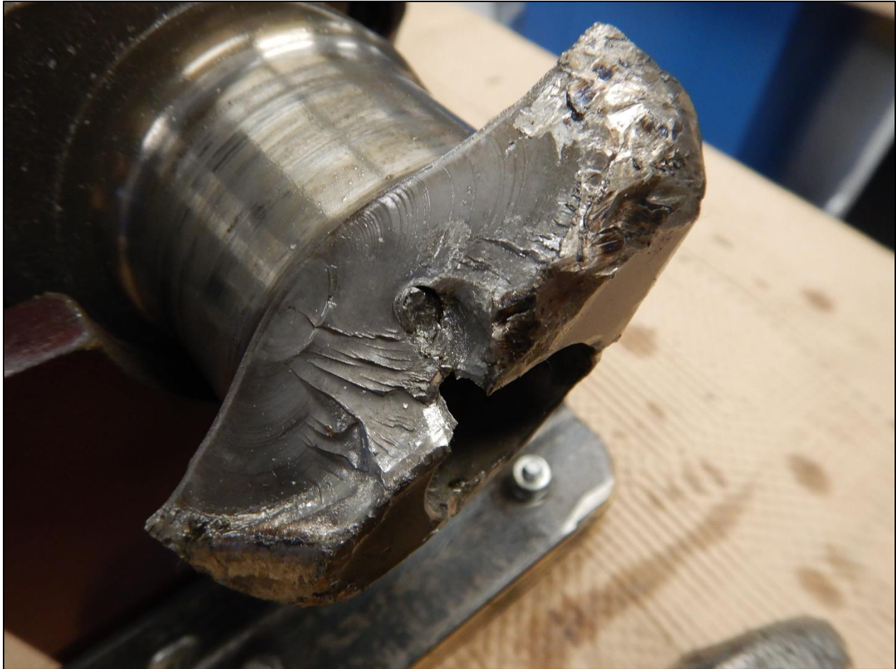
Figure 2-Crankshaft separation surface near the No. 3 main bearing journal.
