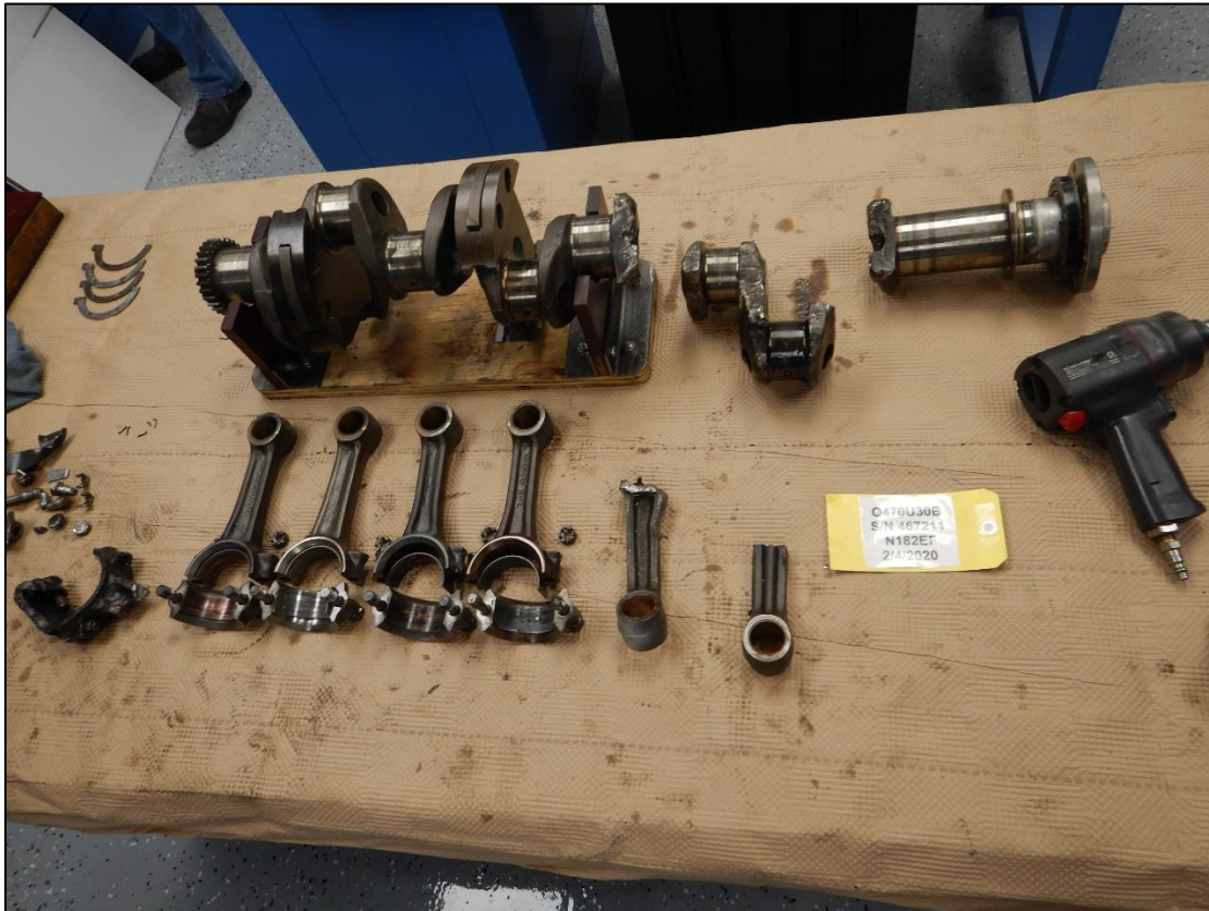
Figure 3-Crankshaft (3 sections) and connecting rods.
