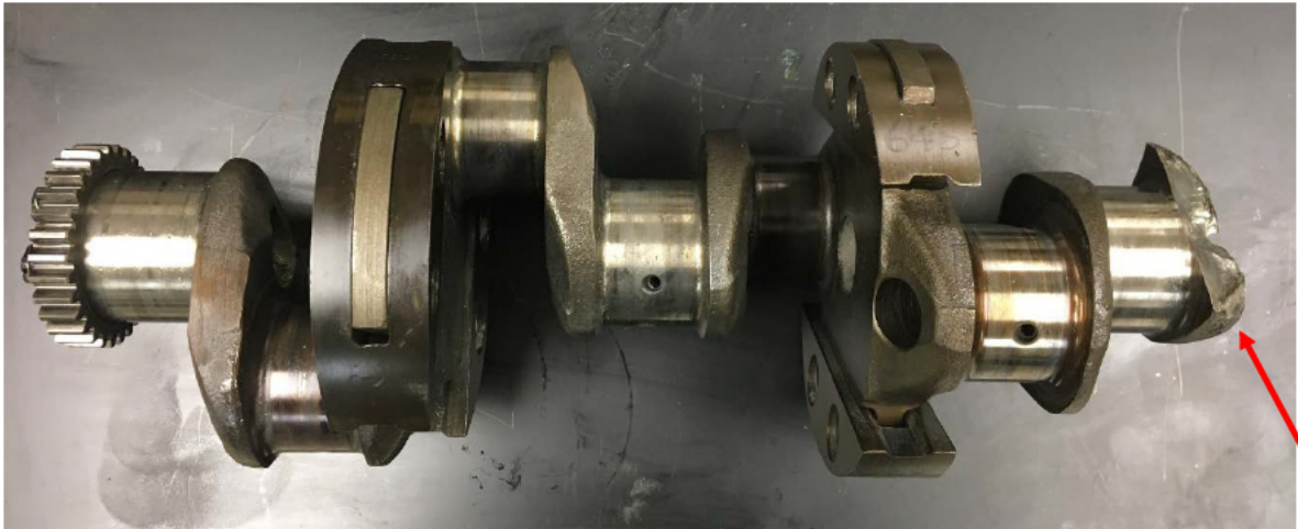
Figure 1 Fractured aft portion of the crankshaft (arrow to fracture surface)
