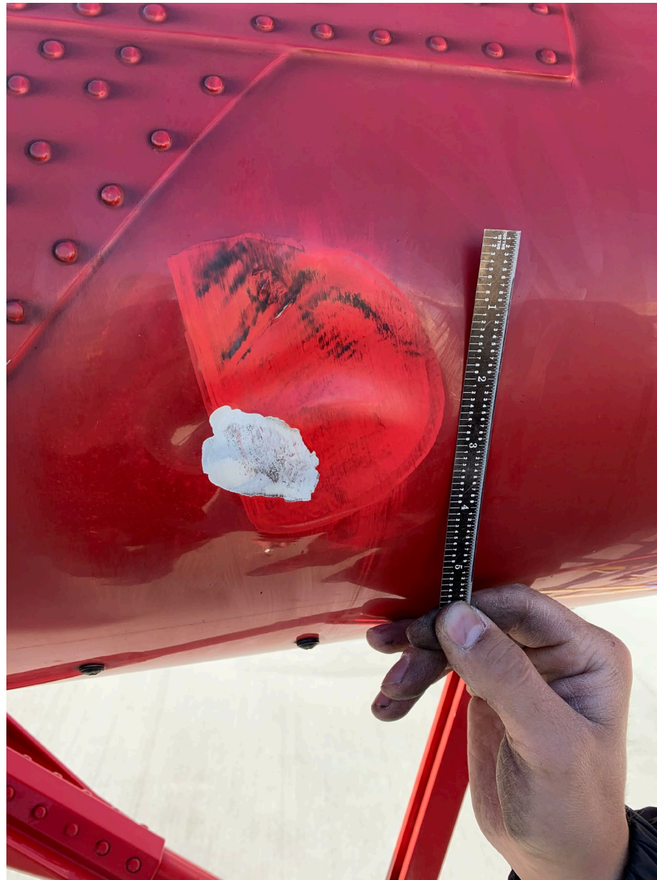
Photo 3 – Closeup of Damage to Left Side Empennage (Courtesy of Intermountain)
