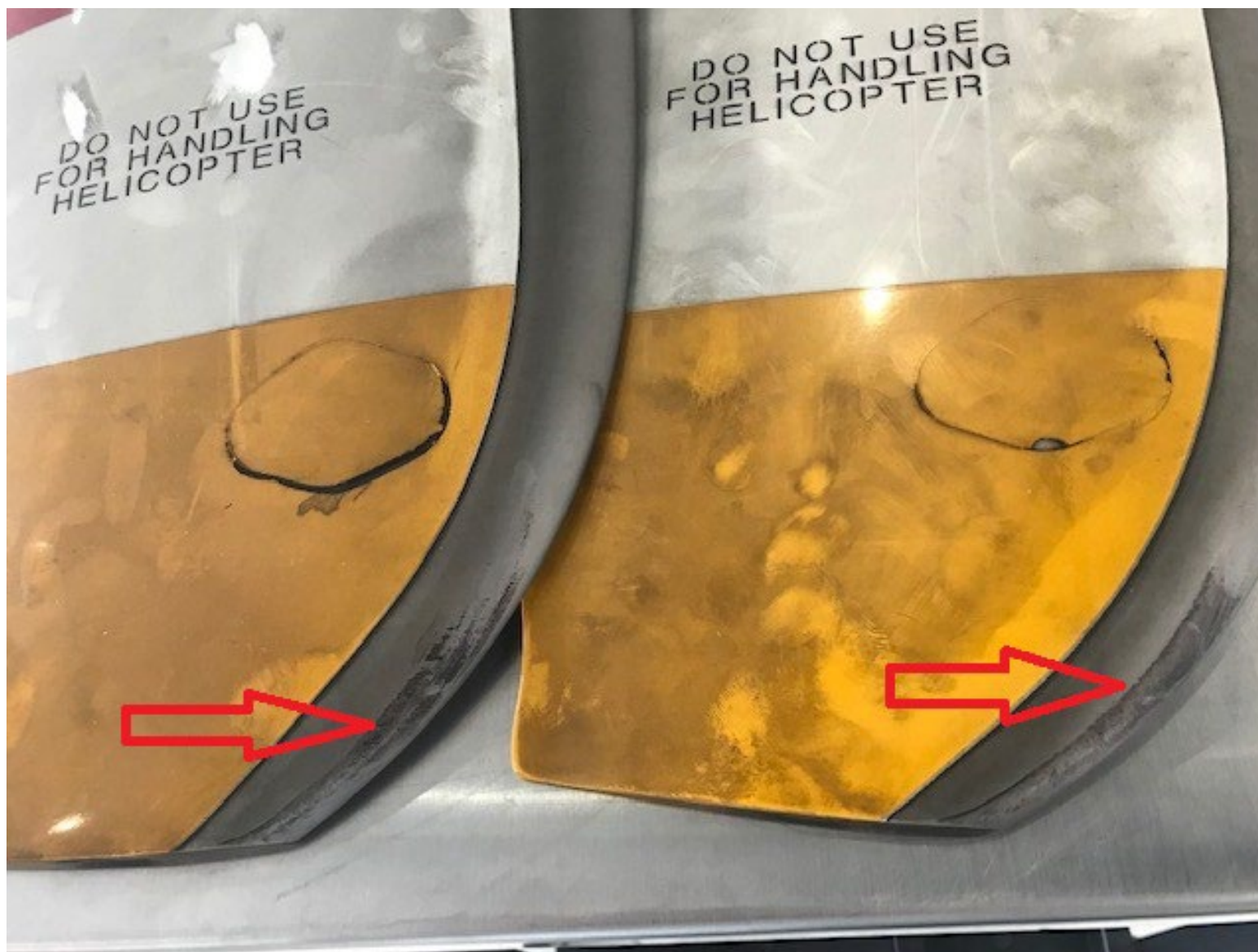
Photo 4 – Damage to Tail Rotor Blades (Courtesy of Intermountain)
