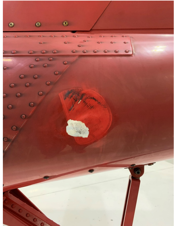
Photo 2 - Close-up view of strike damage to empennage.
