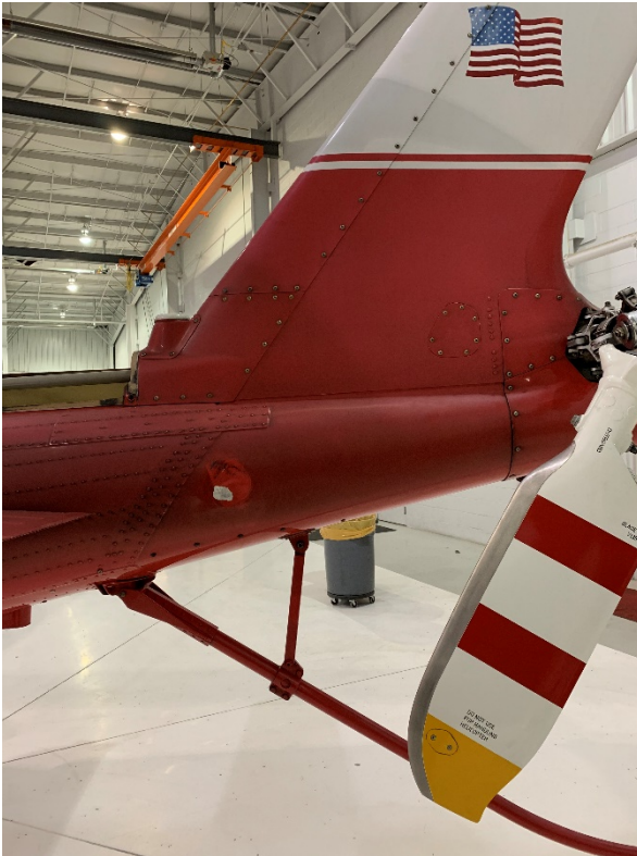
Photo 1 - Tail section showing tail rotor blade tip strike on the empennage.
