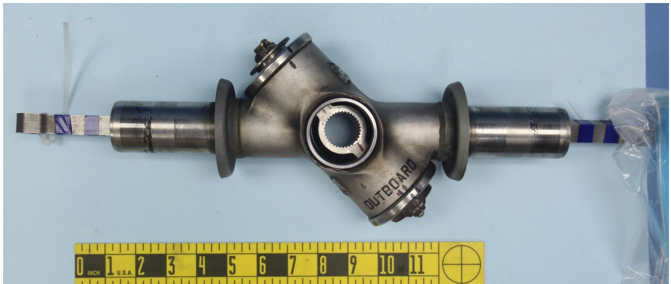
Figure 14 – The tail rotor hub assembly, from the outboard side.
