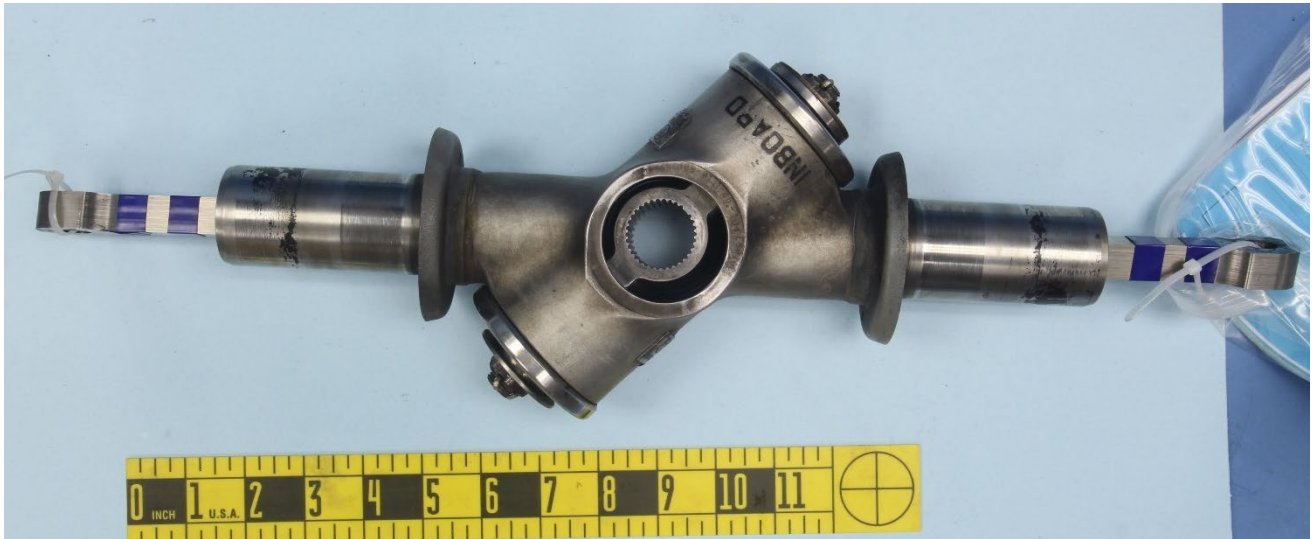
Figure 15 – The tail rotor hub and blade assembly, viewed from the inboard side.
