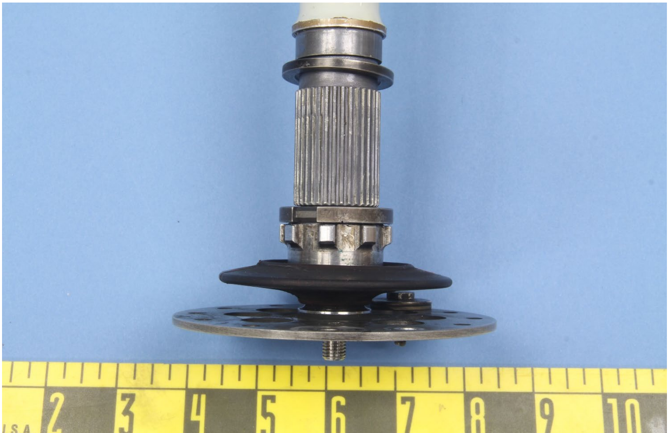
Figure 8 – Side view of the arm from Figure 7, showing the splined area of the shaft and the washer (loose on the shaft).
