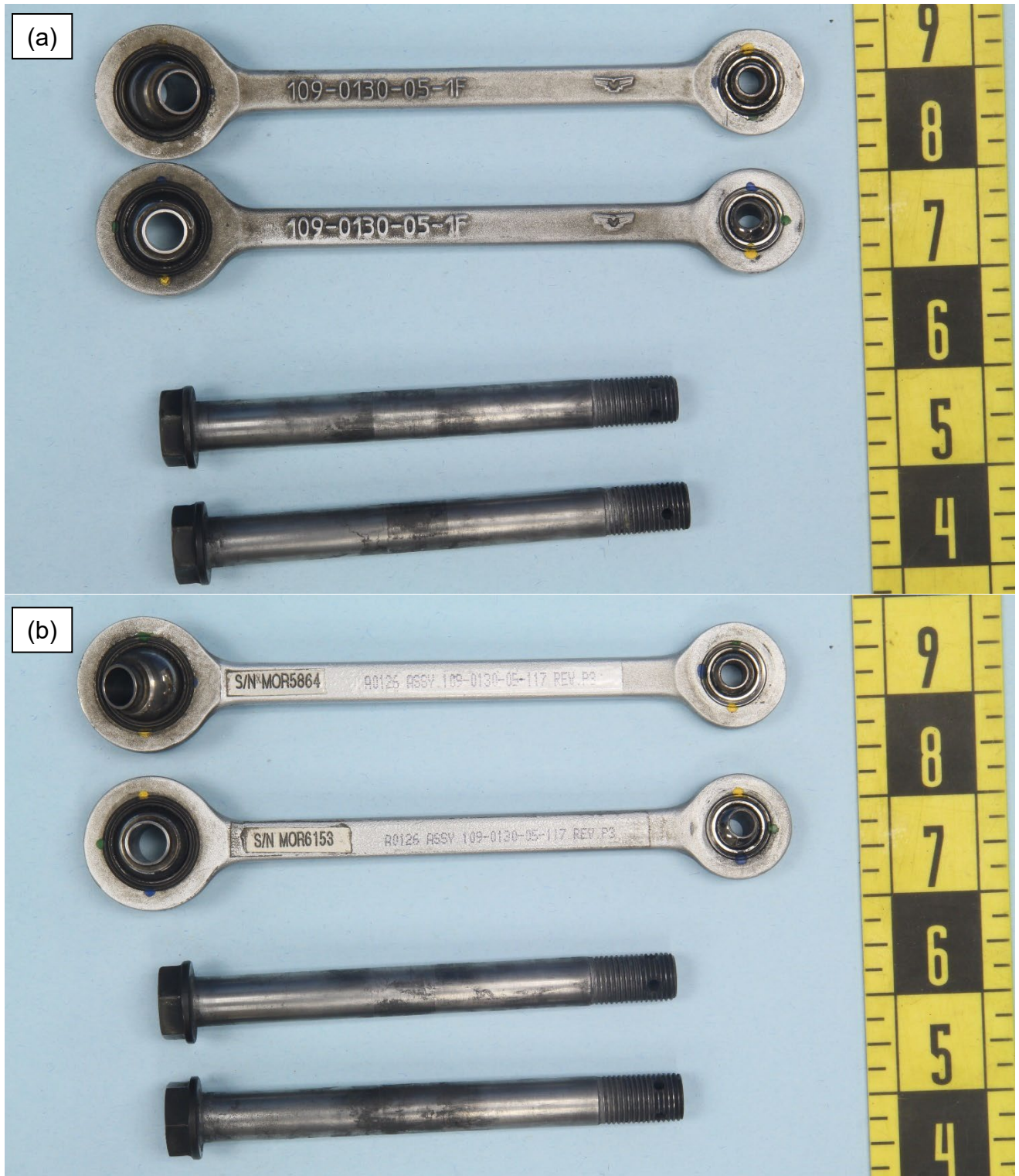
Figure 9 – One set of links and bolts from (a) the obverse and (b) reverse sides.
