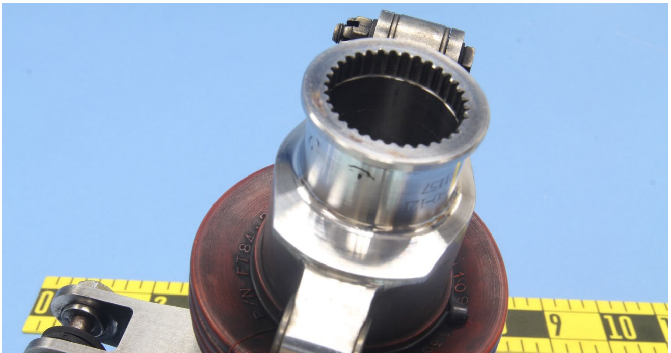
Figure 12 – View of the splined driven connection of the slider assembly in Figure 11.
