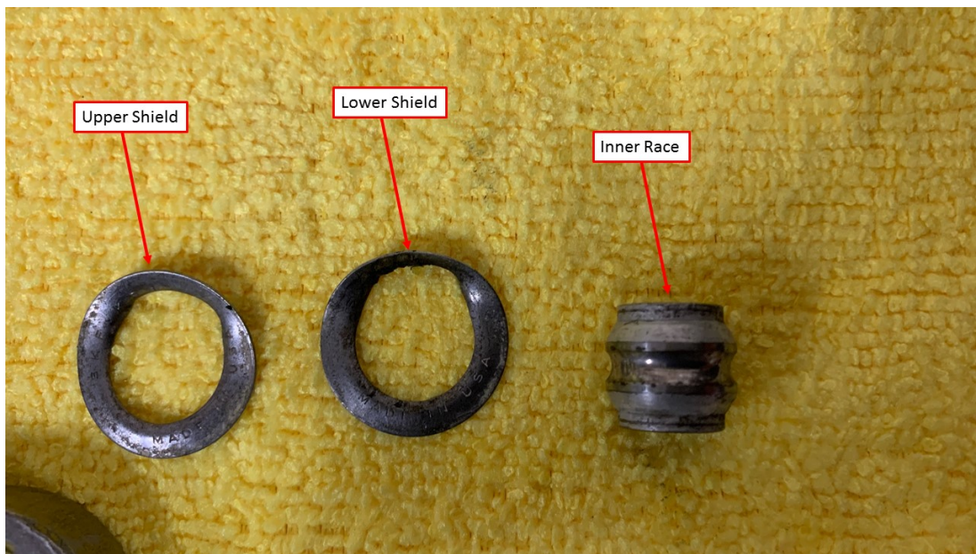
Figure 5: Upper and lower bearing shields and inner race.
