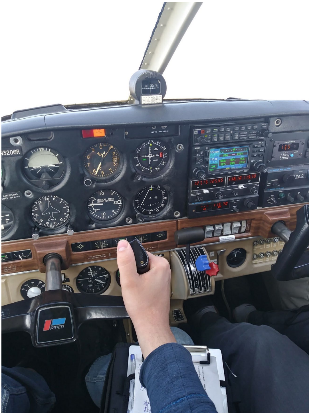
Figure 3. Photo taken from a previous flight showing the Gear in Transit light illuminated.
