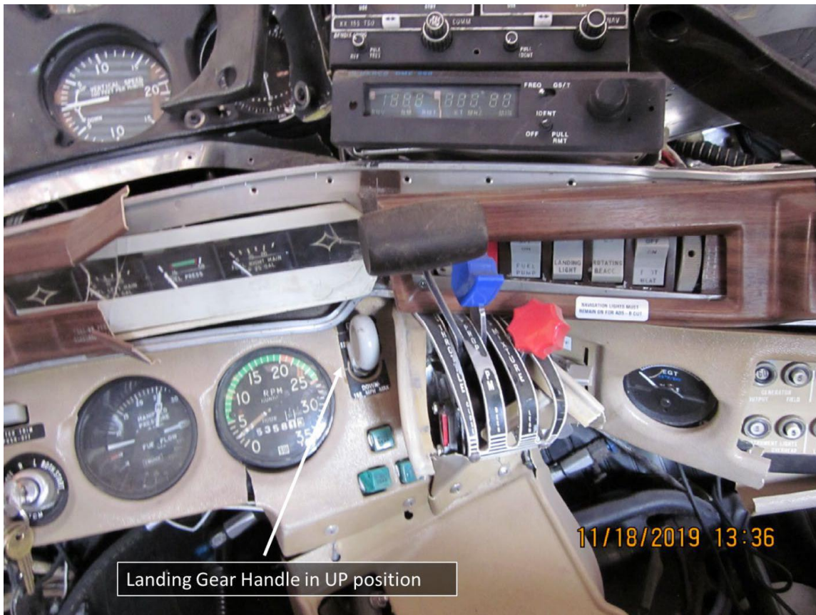
Figure 20. Image showing the main landing gear handle in the up position.
