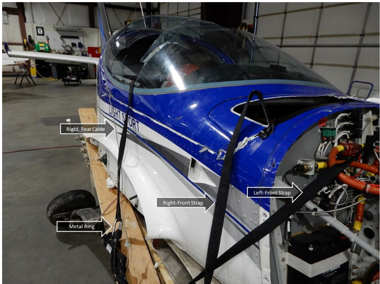
Figure 4. Photo showing the two straps, the right-rear cable, and the metal ring.
