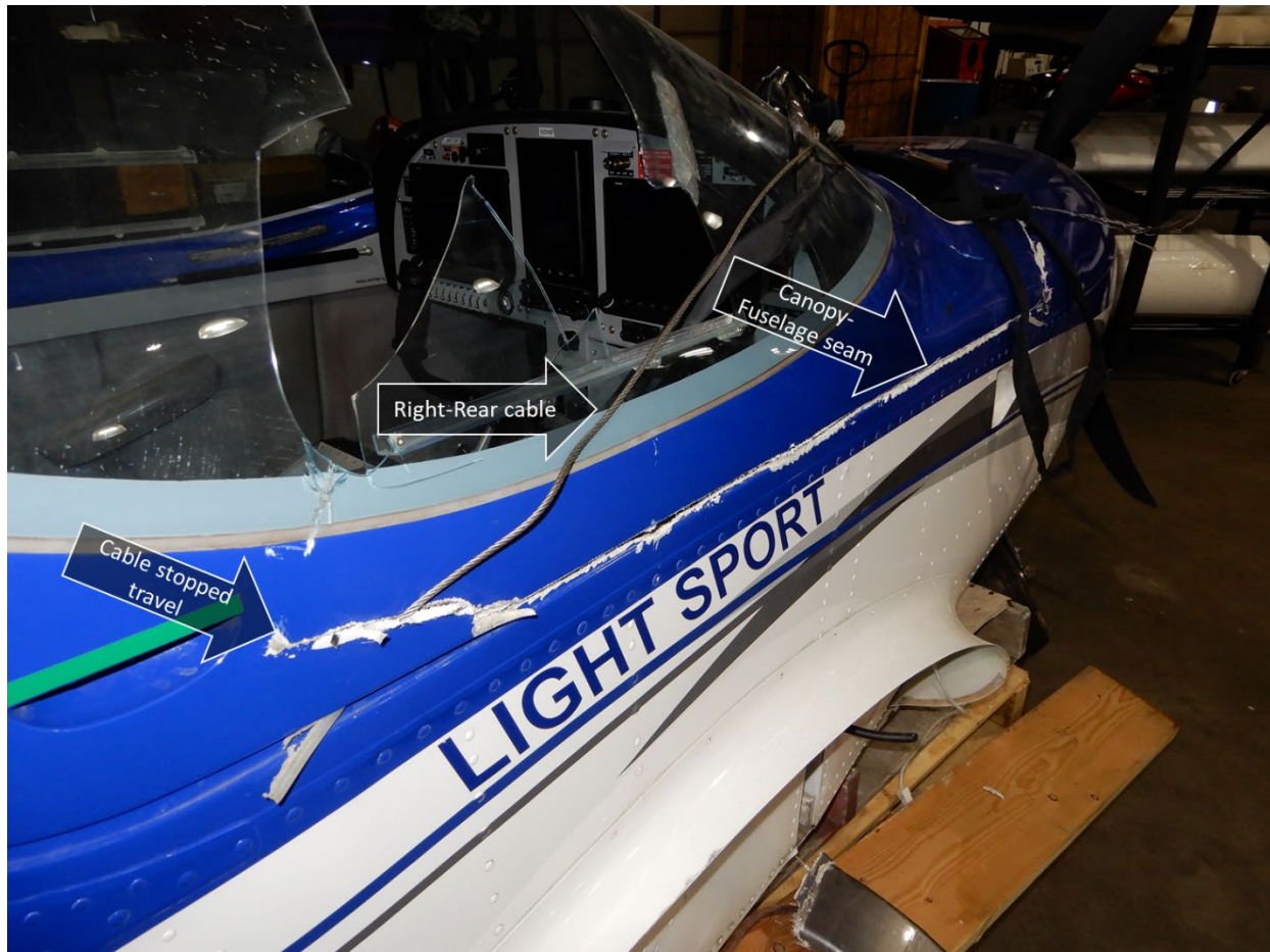
Figure 5. Photo showing the path of the right-rear cable.
