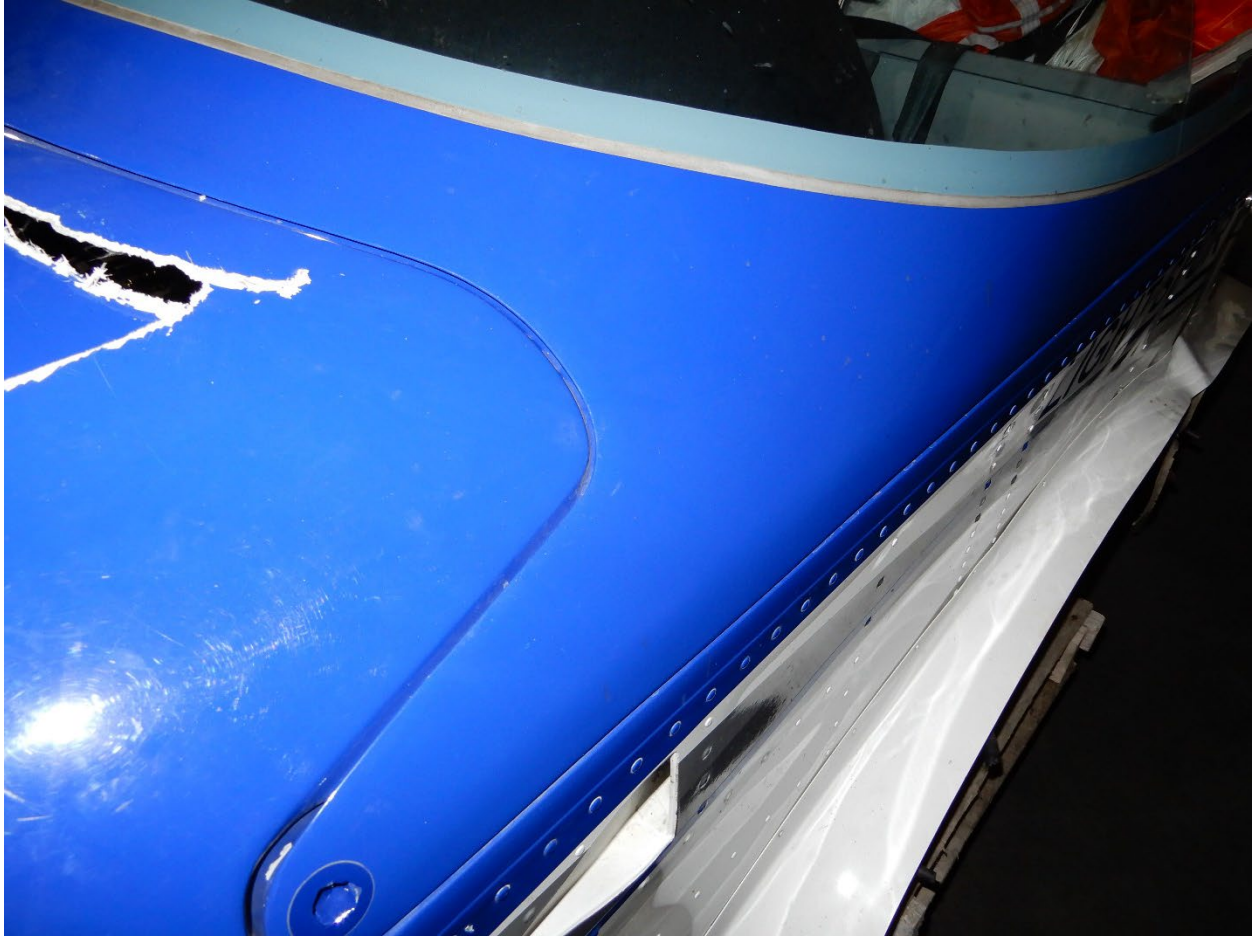
Figure 3. Photo showing the left-side suspension cable did not exit the forward nose compartment.
