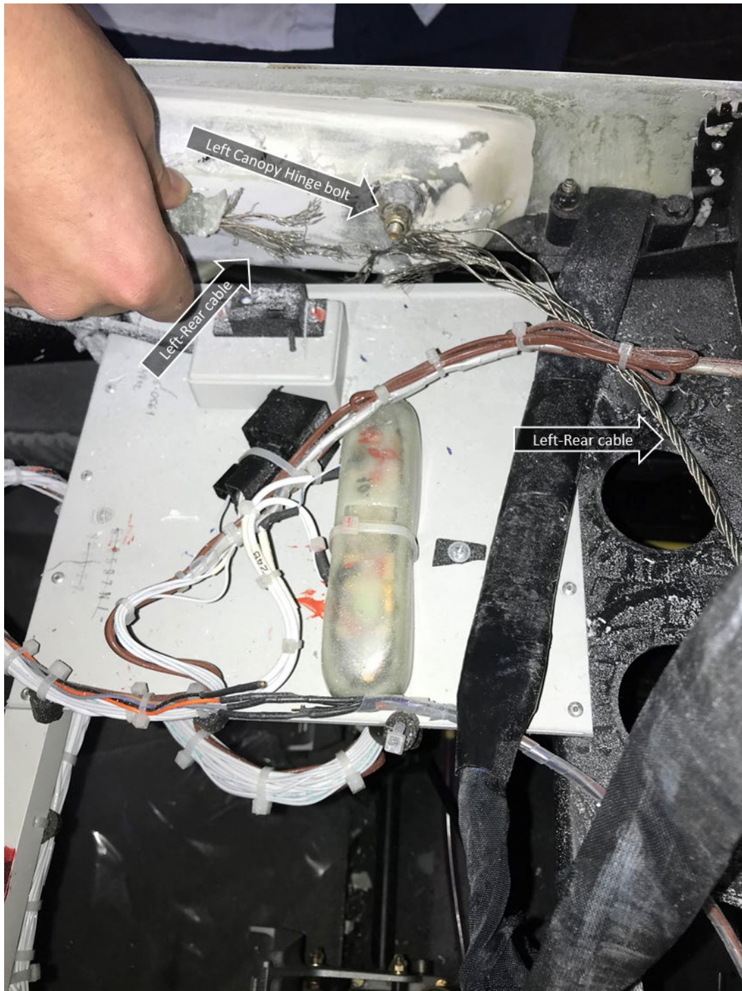
Figure 1 Photo showing both ends of the fractured left-side steel cable, and the left-side canopy hinge bolt and nut.
