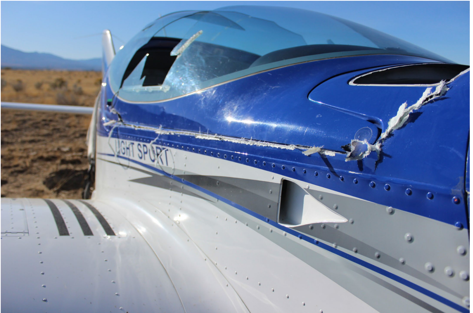
Photo 4 – Right-side view showing the fuselage damage from the BRS right-rear suspension cable. Photo courtesy of the operator.
