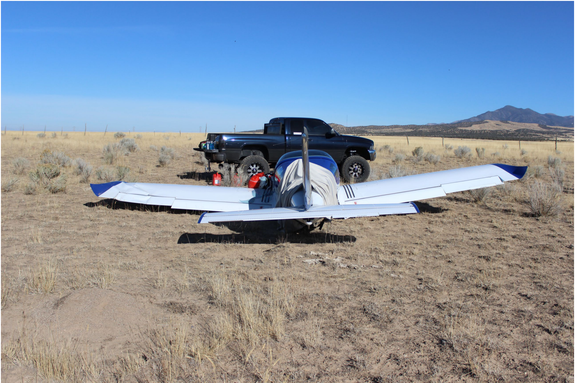
Photo 3 – Rear-view, showing substantial damage to the left wing
