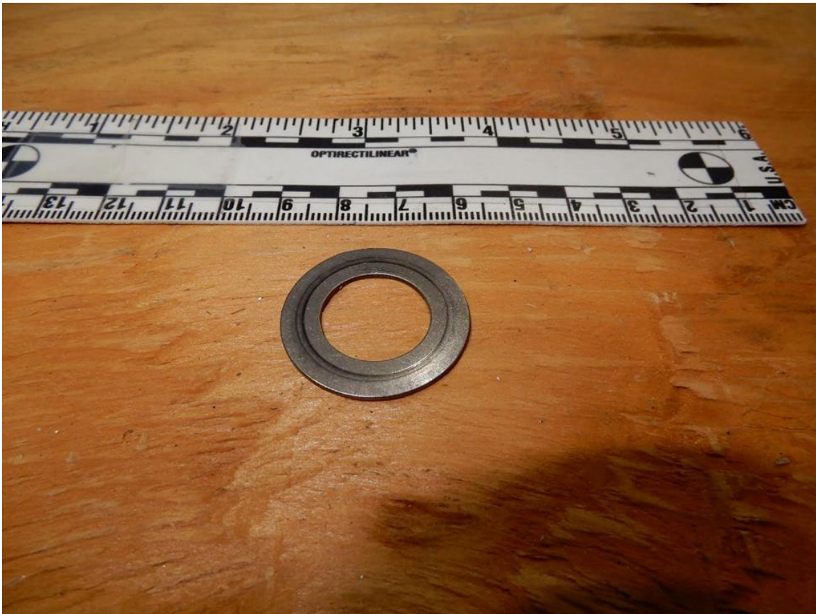
Figure 13. Number two-valve spring shim, showing a worn, circular groove.
