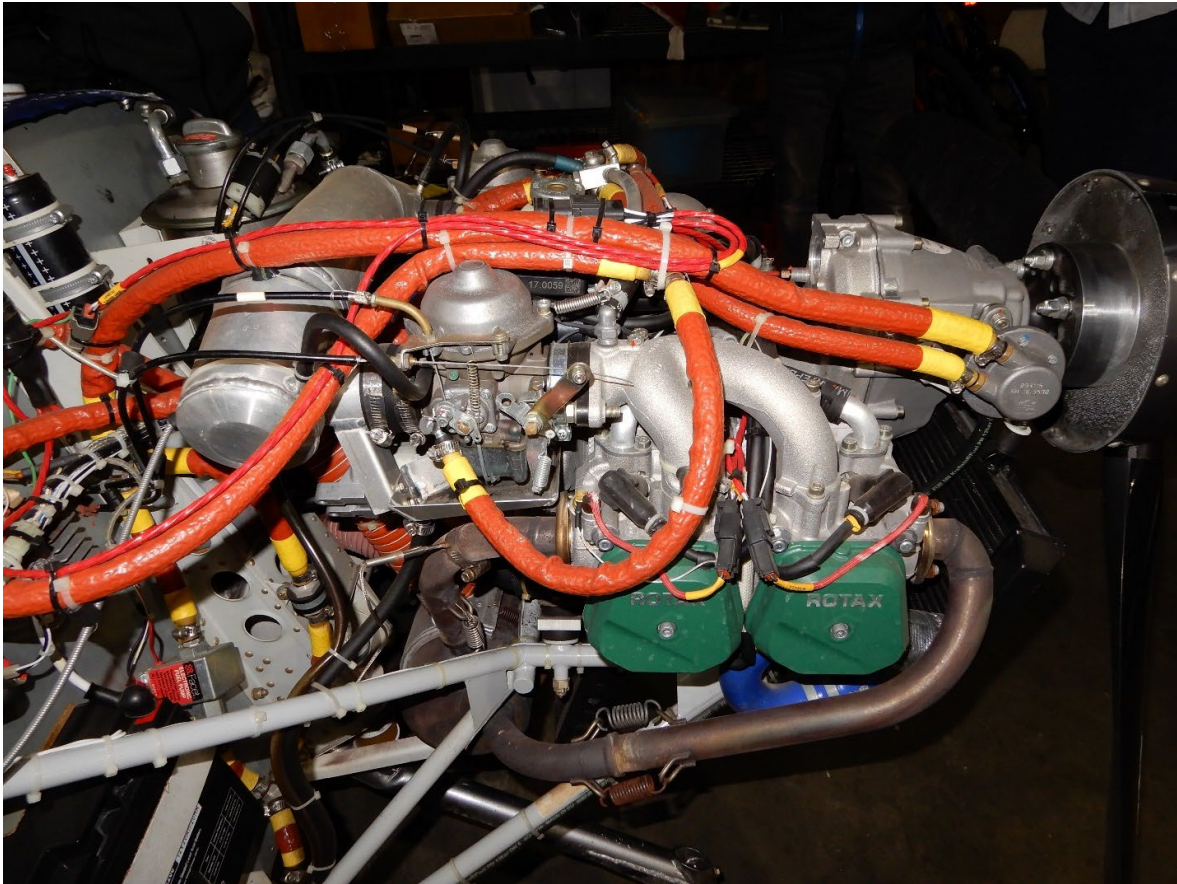
Figure 11. Right-side view of the engine, showing the number one and three-cylinders.
