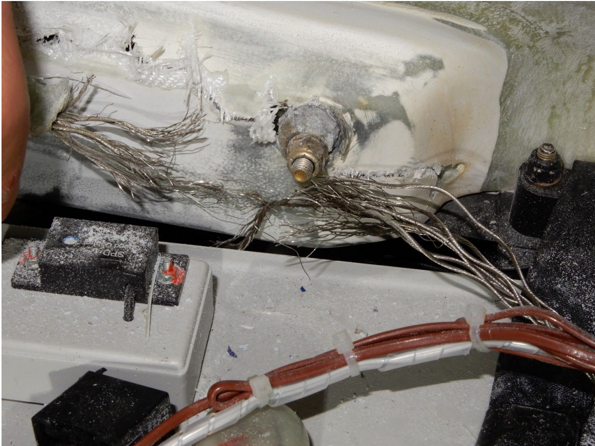
Figure 9. left-side internal view of the break in the left-side BRS suspension cable near the location of the canopy hinge bolt.
