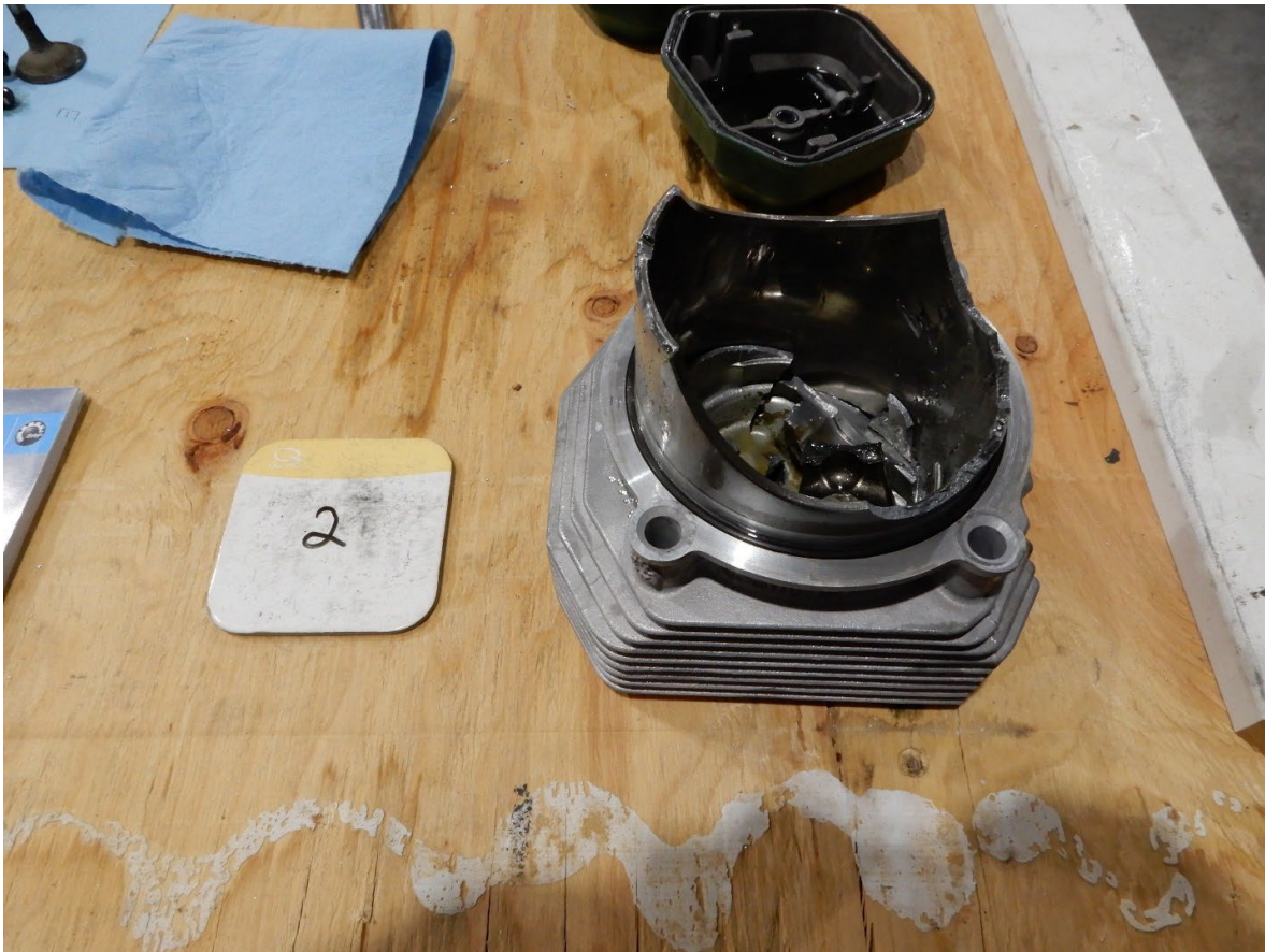
Figure 15. Number two-cylinder, bottom view, showing the fractured cylinder skirt. The fracture piston skirt is visible.
