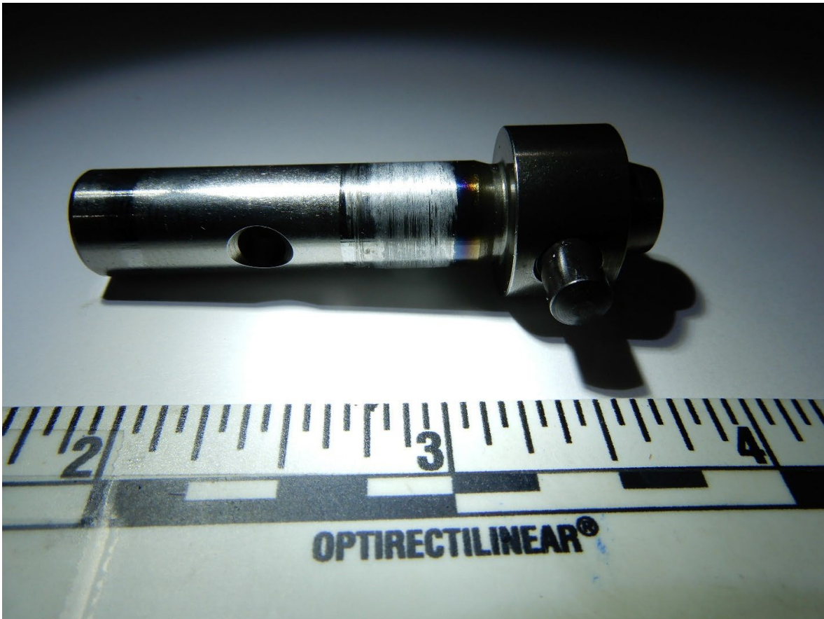
Figure 18. Oil pump shaft, showing discoloration and galling.
