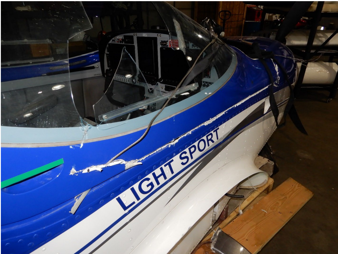
Figure 7. Right side, showing exemplar track for the BRS right-side suspension cable.
