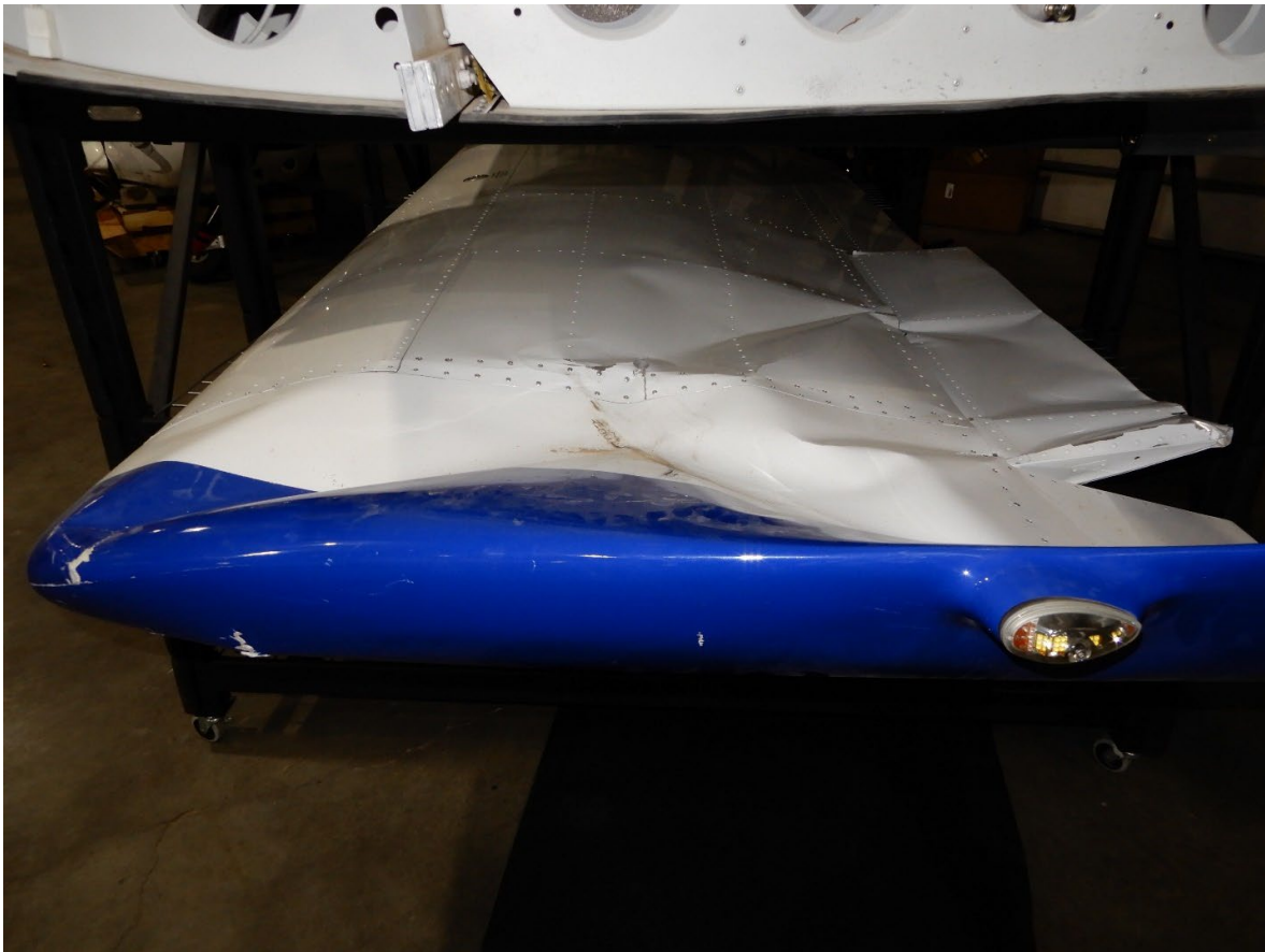
Figure 6. Left wing, showing substantial damage.
