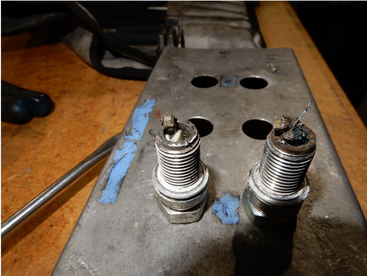
Figure 20. Number two-cylinder, top and bottom spark plugs.
