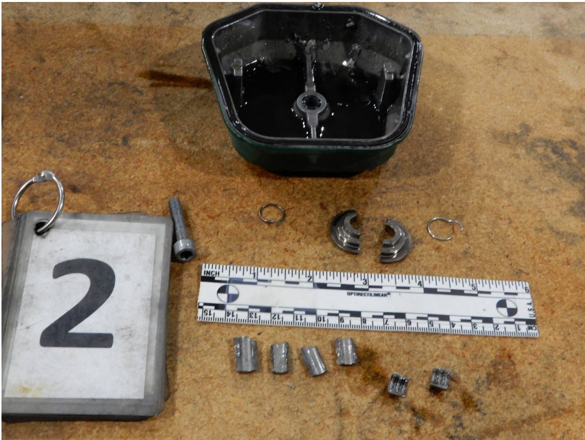
Figure 12. Number two-rocker box cover and contents found in it upon removal.
