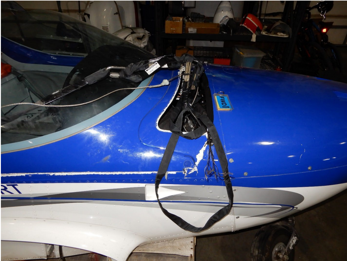
Figure 8. Right-side, forward view of the exemplar track for the BRS right-side suspension cable.
