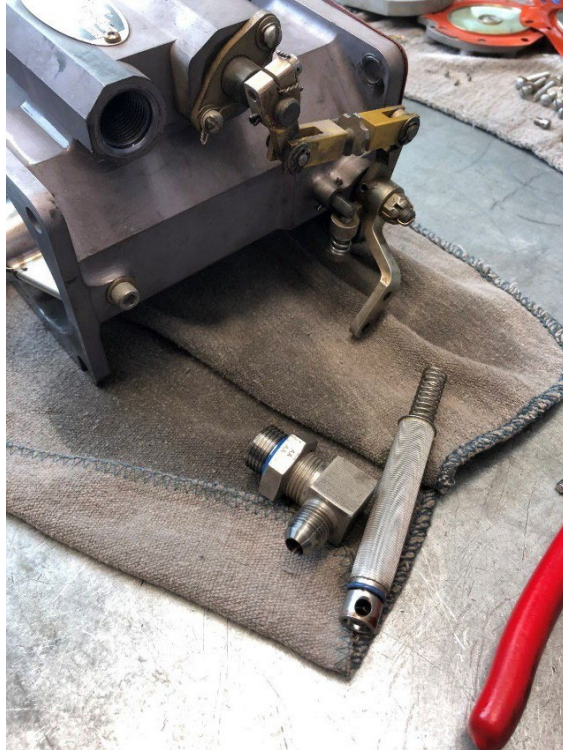
Figure 8: View of the fuel servo filter.
