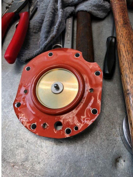
Figure 6: View of the inside (second) fuel diaphragm.
