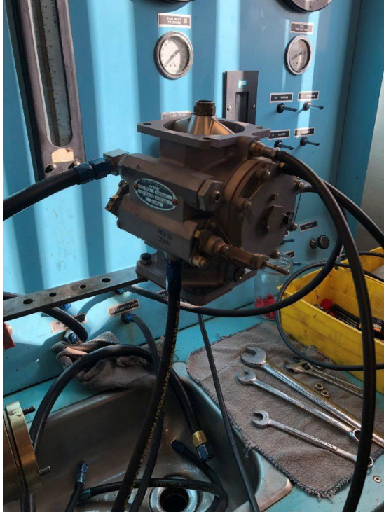
Figure 2: View of the fuel servo on flow test stand
