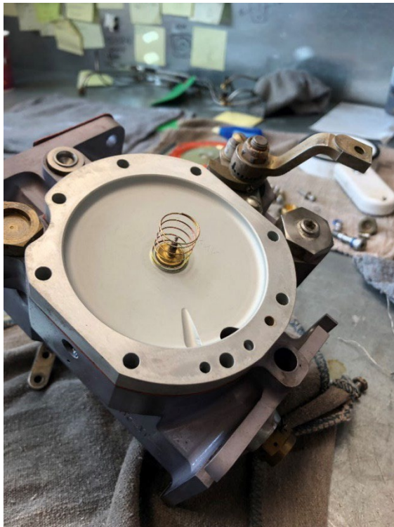
Figure 5: View of the top cover and first diaphragm removed.
