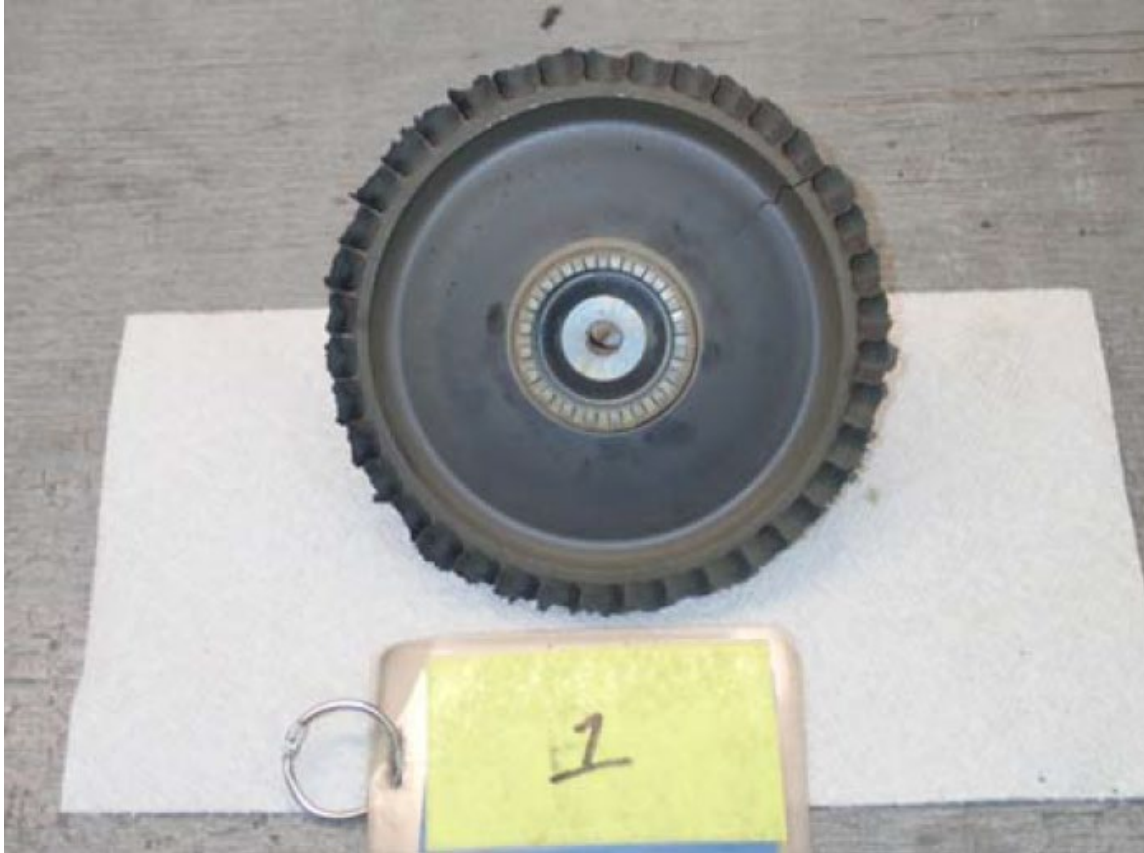
Figure 18. Stage 1 turbine wheel, showing crack extending into the web. Photo courtesy of Rolls-Royce.
