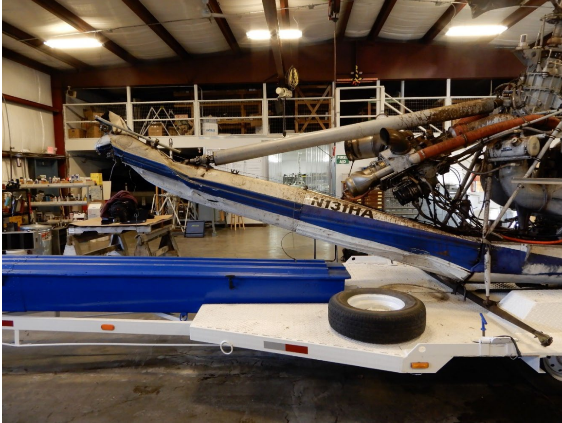
Figure 5. Right-side view showing damage to the tailboom. Photo NTSB.
