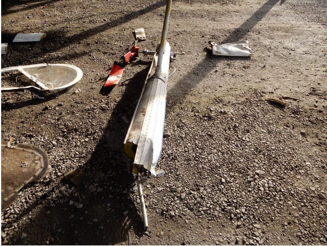
Figure 12. View of the separated tailboom and tail rotor assembly. Photo NTSB.
