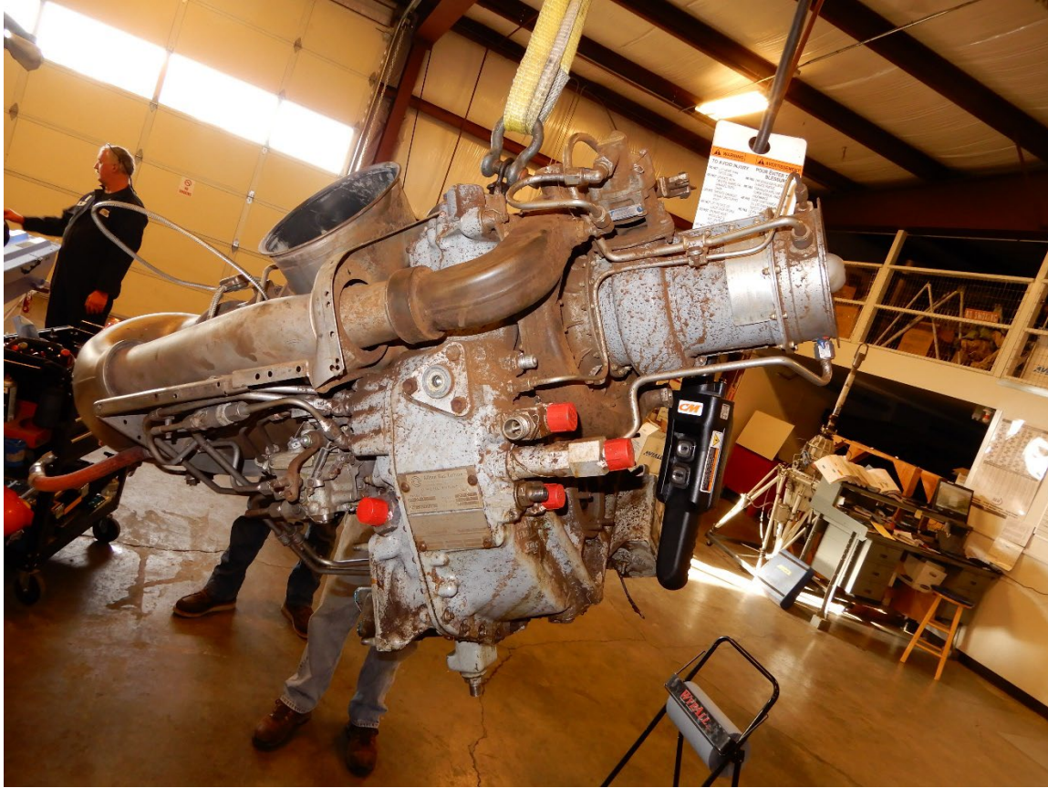
Figure 16. Right-side view of the 250-C20B turbine engine. Photo NTSB.
