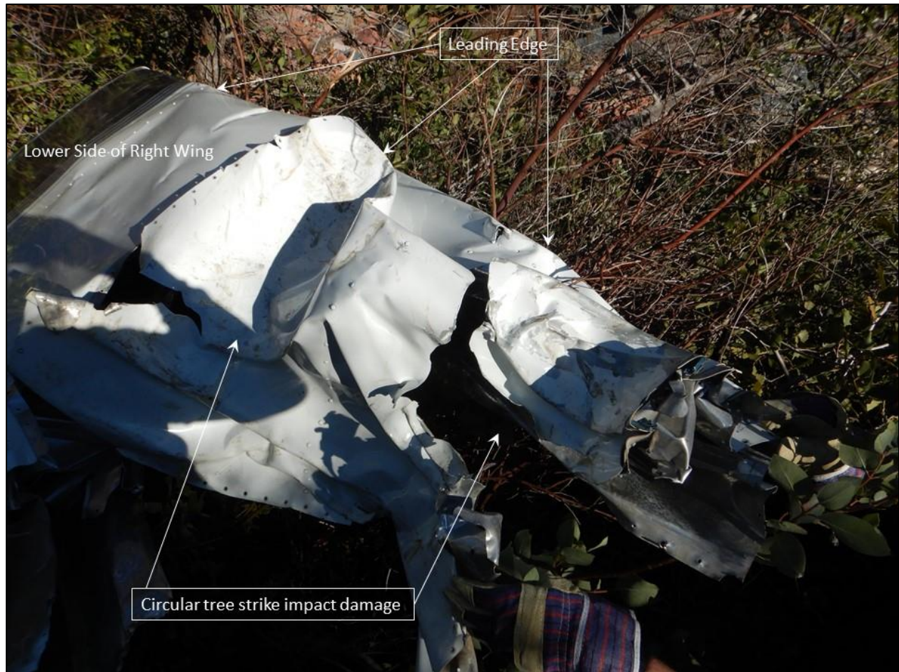
Figure 5-Right wing lower surface and tree strikes
