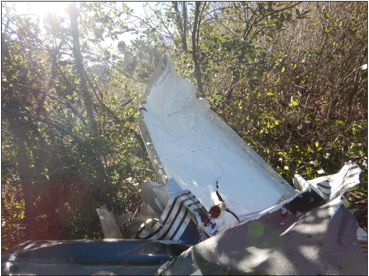
Figure 7-Inboard section of the right wing
