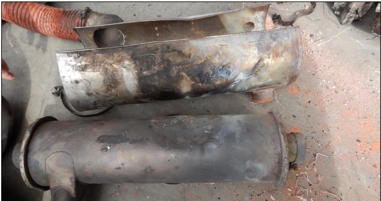
Figure 5-Exhaust assembly, removal of the cabin heat shield.
