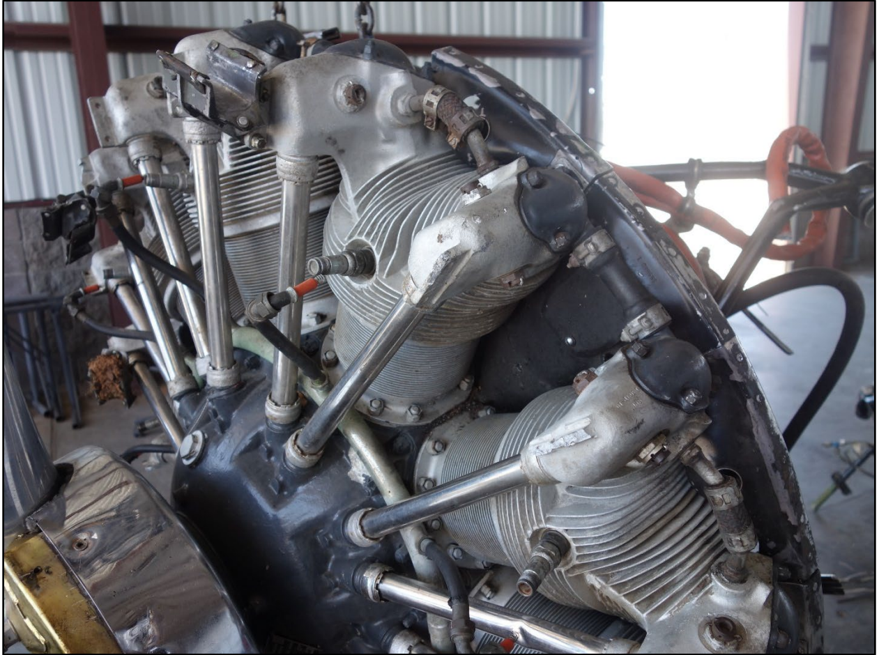
Figure 2: Ignition wire exhibiting wear and fraying as viewed from the front of the engine.
