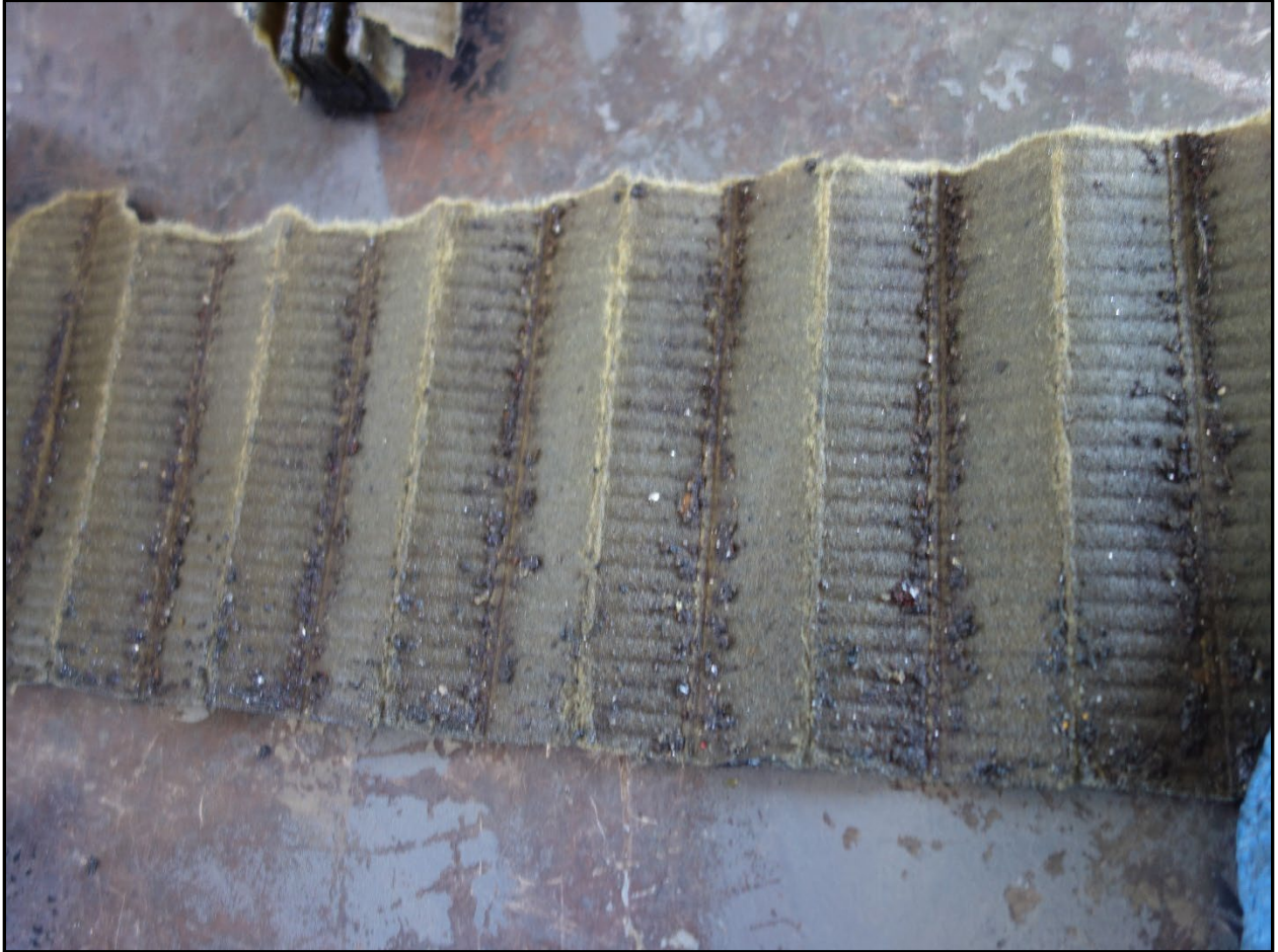
Figure 3: Oil filter element folds contained dark and shiny debris.
