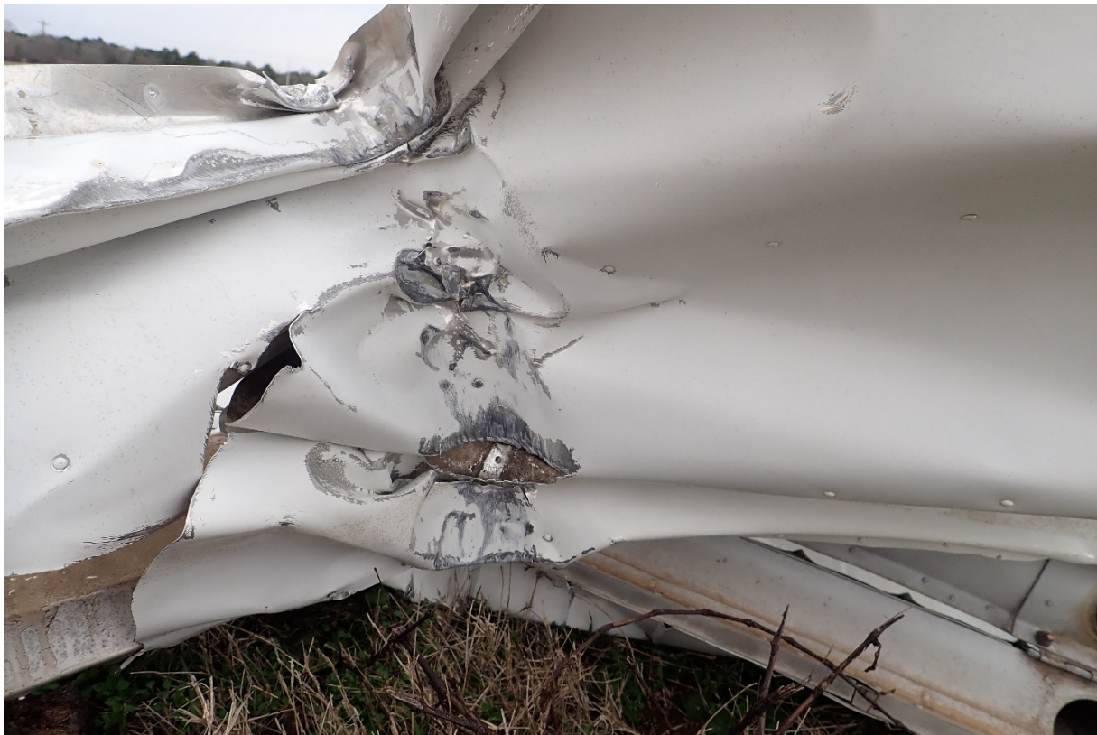
Wire marks on left outboard wing section, ASI-20-AE-081
