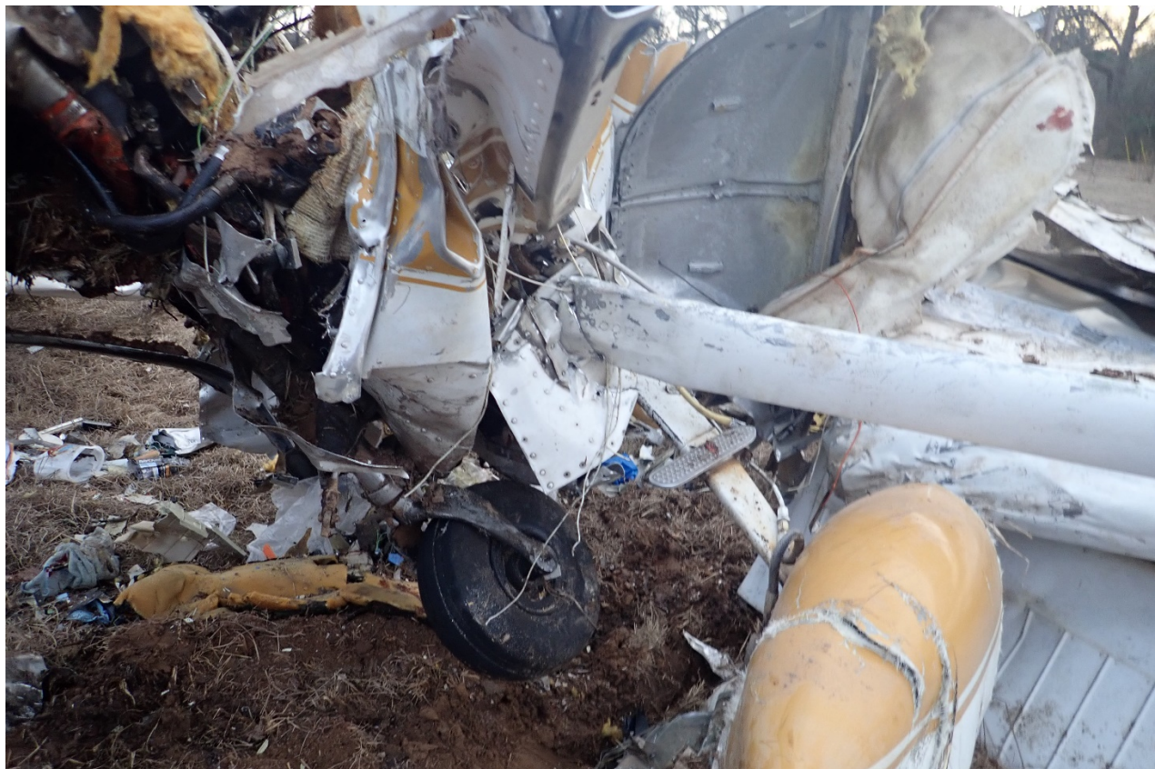
Nose and left main landing gear, ASI-20-AE-110
