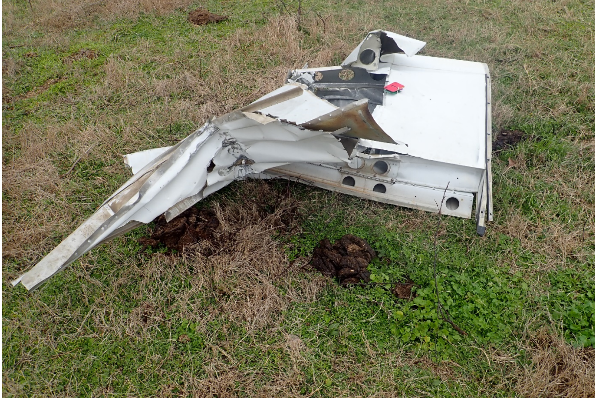
Separated section of left outboard wing, ASI-20-AE-079
