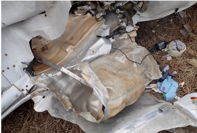
Right fuel tank in wing, ASI-20-AE-038
